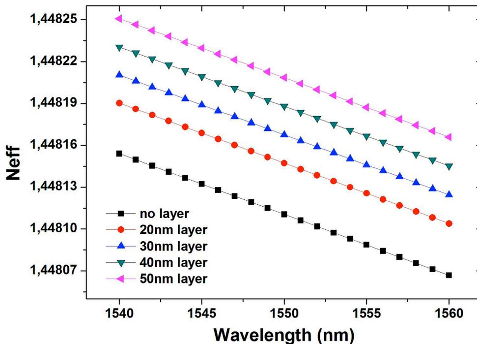
**Fig. 8.5** Results of finite element calculations carried out for different wavelengths and different thickness of the biolayer on the channel surface.
