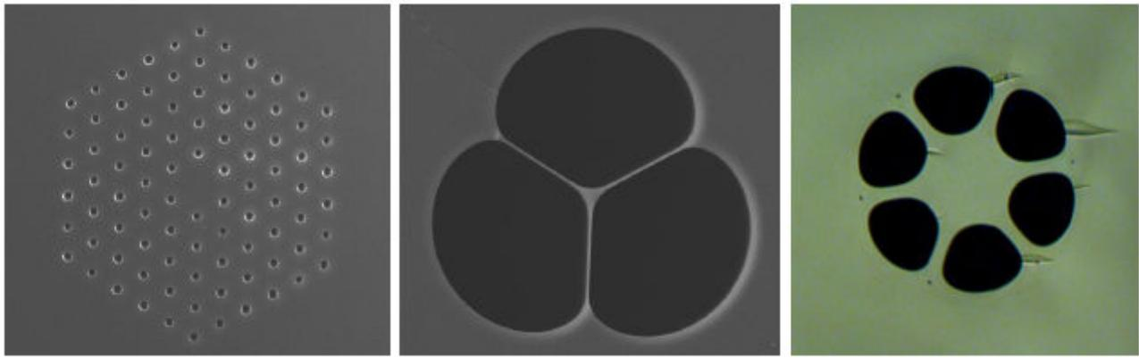
**Fig. 7.2.** Photonic crystal fibers with a hexagonal pattern of air holes forming the microstructured cladding (left), air-suspended core fiber (center), and hole assisted fiber (right). Adapted from R. Corradini, S. Selleri, *Photonic Crystal Fiber for Physical, Chemical and Biological Sensing in Photonic Bandgap Structures*, Bentham Publisher, **2010**, 80-84.<sup>[18]</sup>
