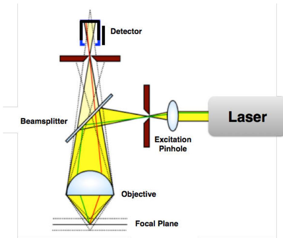
**Figure 10.6** Schematic picture showing the principle of confocal microscopy.
