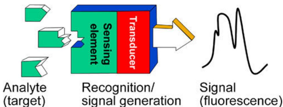
**Fig. 9.1** Schematic layout of a fluorescent biosensor. Springer, *Analytical and Bioanalytical Chemistry*, 399, 2011, 3157, Nucleic acid-based fluorescent probes and their analytical potential B. Juskowiak, Figure 1, with kind permission from Springer Science and Business Media.
