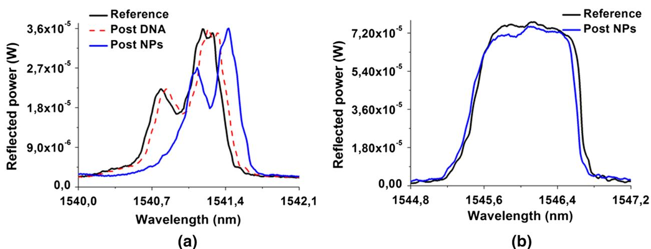
**Fig. 7.7** Spectral measurements after the hybridization process with 100 nM full-match DNA solution (dashed red line) and after ON-AuNPs flow (blue line). A) A clear wavelength shift was recorded for the higher order mode, in the range of 0.27 nm; B) The fundamental mode did not show any significant change in the peak position.
