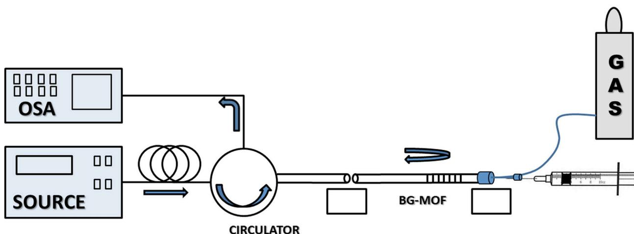
**Fig. 7.6** Schematic of the optical setup implemented for the analysis. The light beam from ASE source is guided through the fiber core and is then reflected due to the Bragg grating; the reflected light is collected through a circulator and sent to a OSA detector. All the samples and reagents are infiltrated through the fiber channels by a syringe pump. The fiber is kept at constant tension (measured by a dynamometer) in order to avoid stretching of the Bragg grating.
