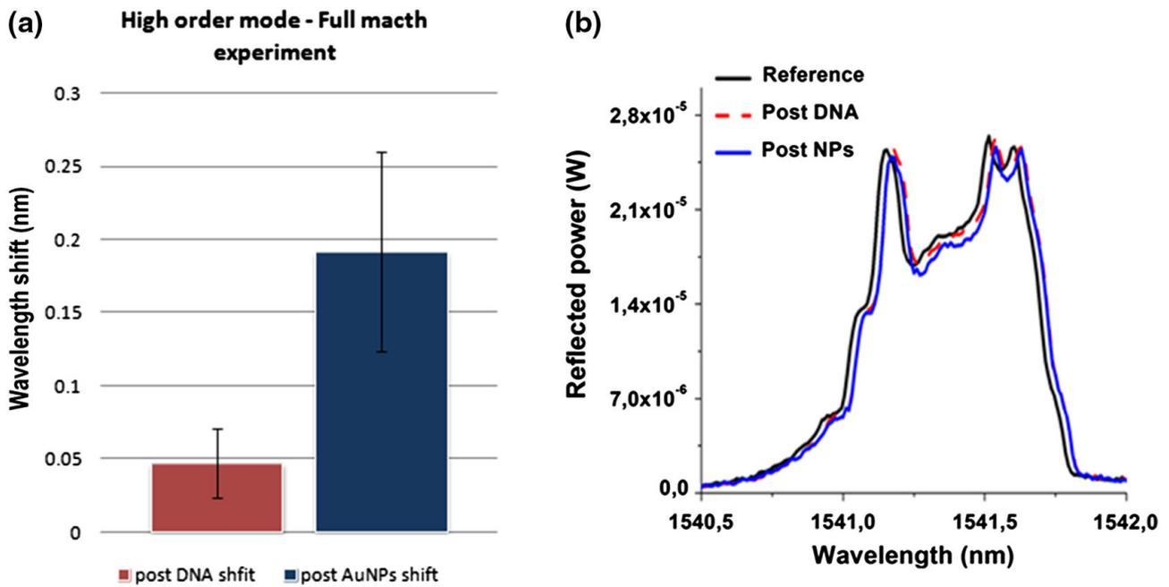
**Fig. 7.8** A) Mean values of the high order wavelength shift after target DNA infiltration (red) and after ON-AuNPs (blue). Vertical bars represent sample standard deviation; a small memory effect decreases the modulation observed for each experiment performed on the same fiber. B) Spectral measurements after the hybridization process using 100 nM mismatch DNA solution and ON-AuNPs.
