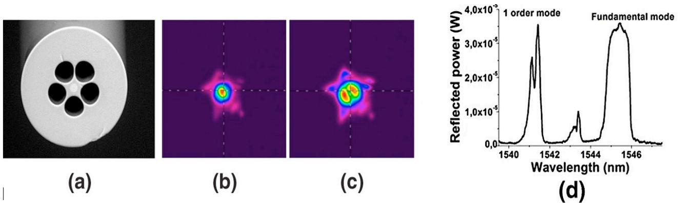
**Fig. 7.3** A) SEM picture of the 5 hole-microstructured optical fiber; B) Fundamental and C) first order beam profiles. D) Reflection spectrum of the PCF, showing the fundamental and the first order modes. The double peak effect visible in the first order band is due to a slight birefringence of the fiber.
