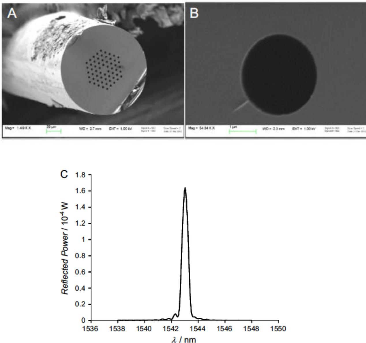
**Fig. 8.1.** LMA-10 fiber structure and Bragg-grating reflection. (A) SEM image of the LMA-10 fiber, showing the hexagonal geometry of the channels. (B) Magnification of a single hole. (C) Spectrum of the reflected light of the LMA-10 PCF with Bragg grating inscribed.
