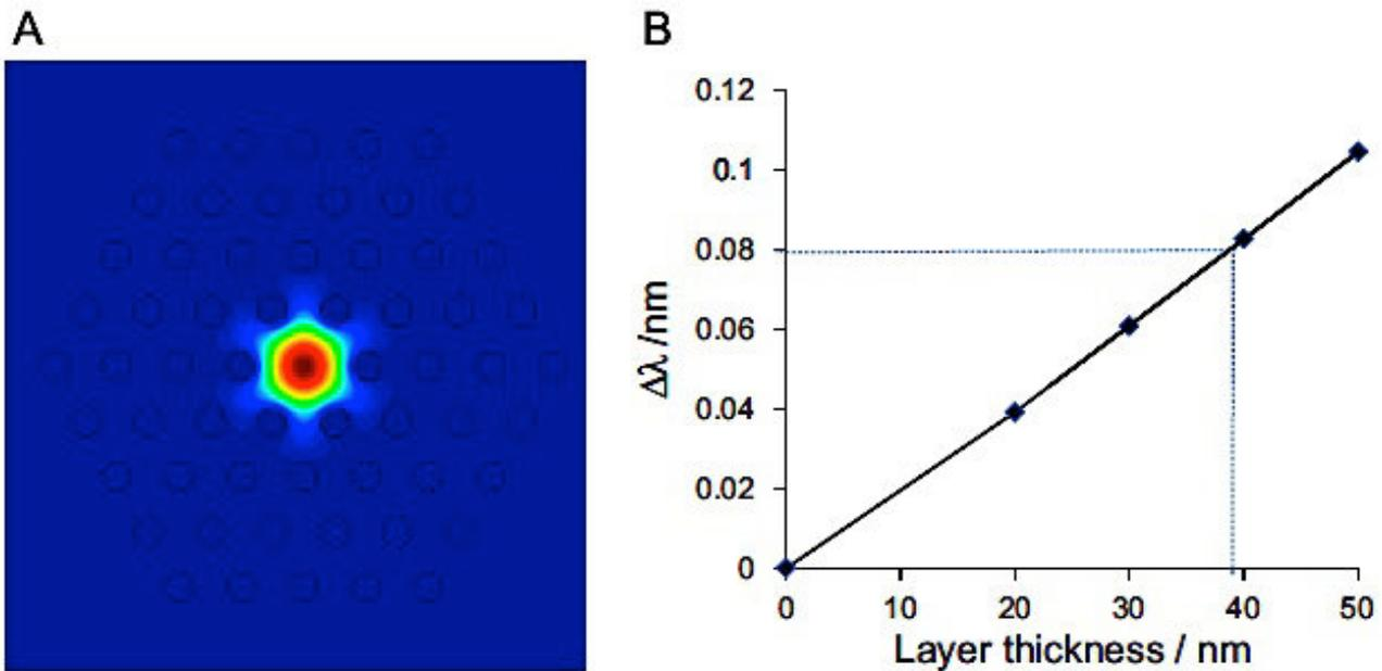
**Fig. 8.6** Modelling of the LMA-10 sensing process. A) Finite element method (FEM) simulations show the field distribution inside the microstructured optical fiber. B) Calculated wavelength shift vs. thickness of the biolayer created upon the functionalization and hybridization processes. The dashed lines represent the observed shift for the 10% RR sample and the corresponding calculated thickness.
