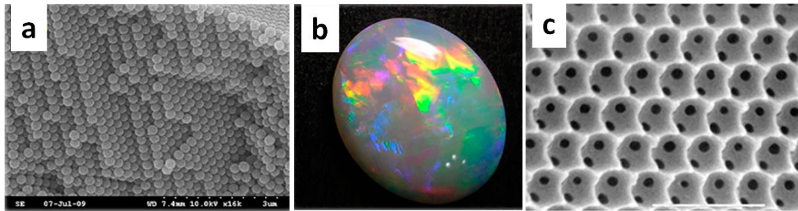
Figure 1.1. (a) SEM image of an artificial silica colloidal crystal (artificial opal) and (b) natural gemstone opal [6]. SEM image of an inverse opal structure obtained after infiltration of a silica-based colloidal crystal by a phenolic resin and its subsequent etching (c) [7].
