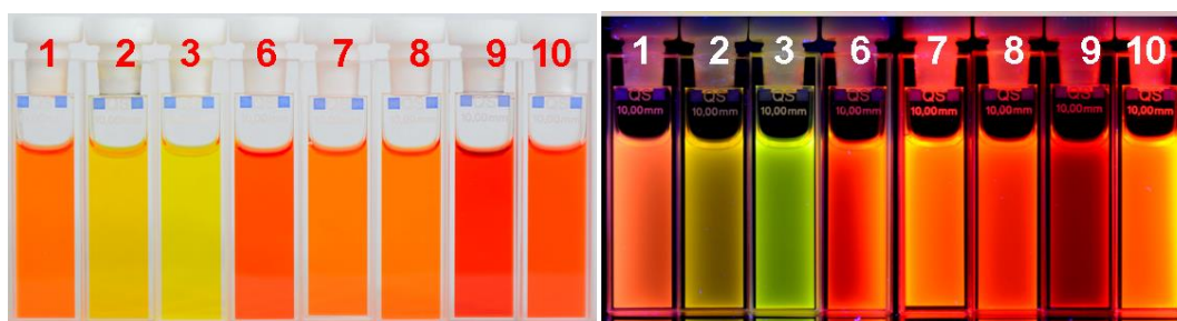
Figure 4-12. The UV-vis absorption and fluorescence emission photographs of dye@F127-SiO 2 NPs in water under UV lamp.
