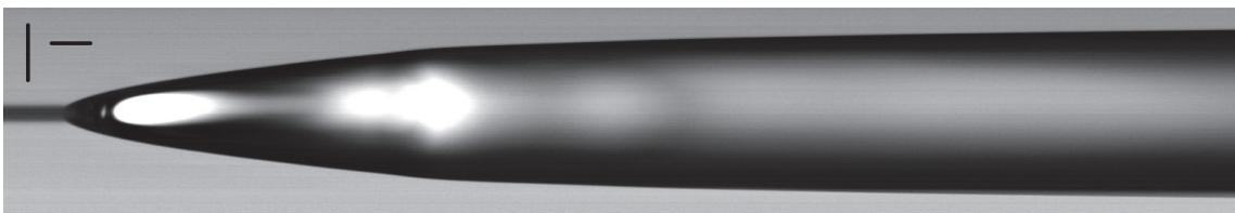
Figure 5.4 – Example of a resliced film (truncated to 1500 images after contact). The film is the same as in figure 5.2. The vertical bar stands for 1 mm and the horizontal one for 1 ms.
