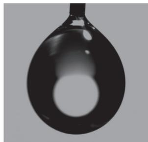
Figure 1.9 – Picture of a pendent drop used to measure the surface tension of a liquid, after fitting the drop outline with a Laplacian profile.
