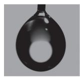
Figure 1.9 – Picture of a pendent drop used to measure the surface tension of a liquid, after fitting the drop outline with a Laplacian profile.
