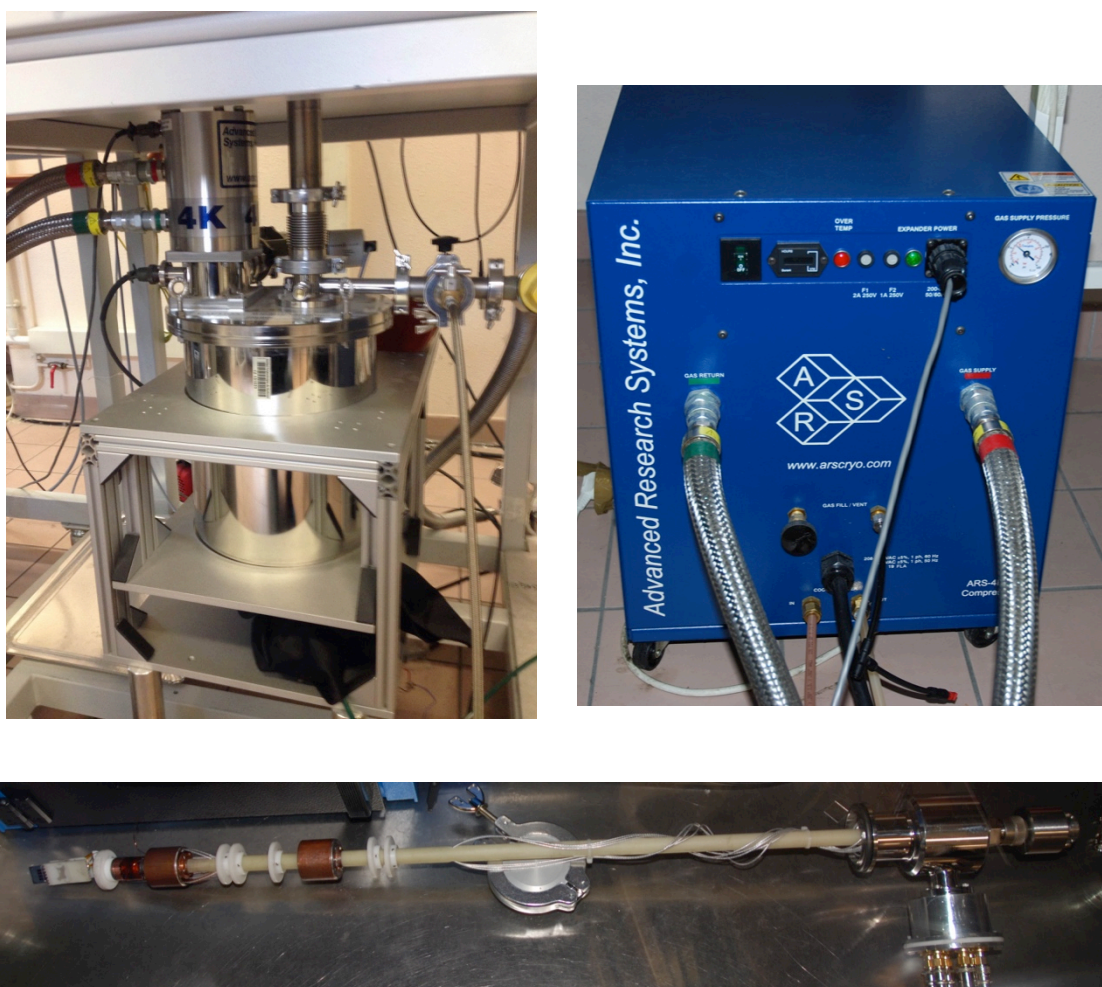
Fig. 3-13 Experimental setup for low temperature J - V - L measurement: Cryostat (upper left), helium compressor (upper right) and sampling rod (down).
