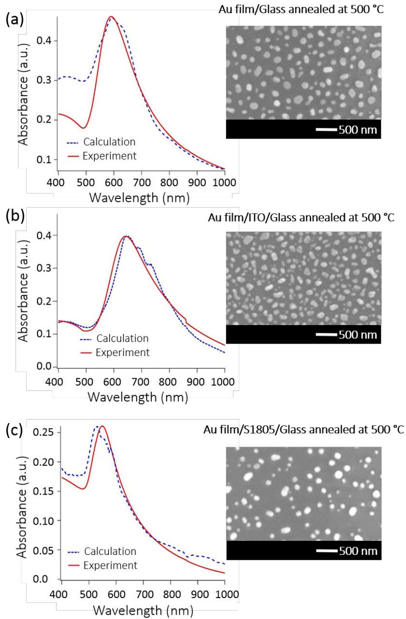
Figure C.2: *Experimental and simulation results of absorbance spectra of Au film structures obtained by thermally annealing Au film sputtered on different substrates: (a) glass, (b) glass coated with ITO, and (c) glass initially coated with S1805 photoresist. The annealing temperature was 500 °C.*
