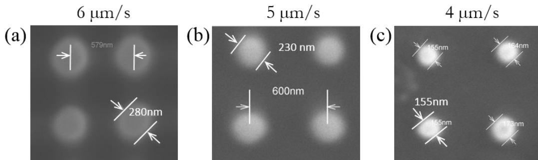
Figure 2.6: SEM images of 2D square structures with  $\Lambda = 0.6 \mu\text{m}$  fabricated by a laser power of  $10 \mu\text{W}$  and a scanning speeds of  $6 \mu\text{m/s}$ ,  $5 \mu\text{m/s}$ , and  $4 \mu\text{m/s}$ , respectively. The size of polymeric cylinders are 280 nm, 250 nm, and 155 nm, respectively.
