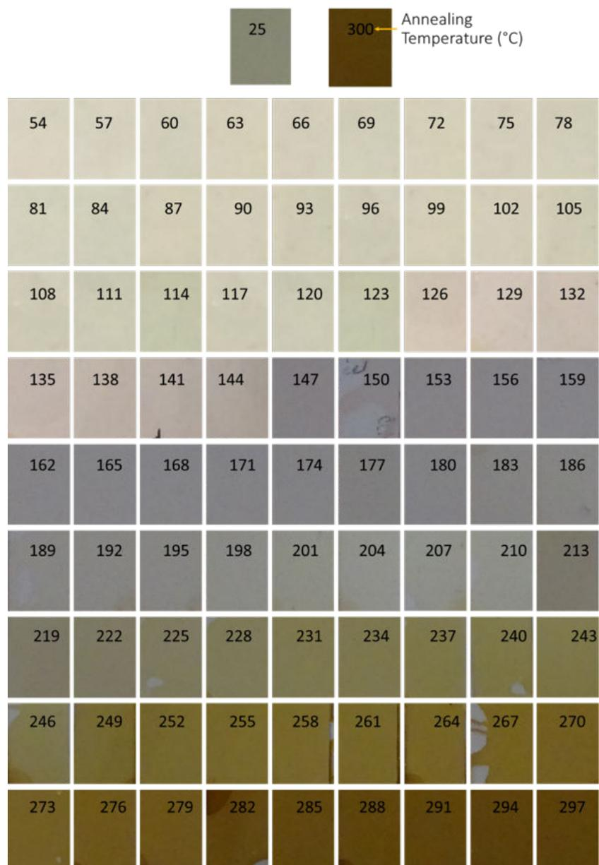
Figure 3.1: Images of S1805 films (thickness of 600 nm) coated on glass substrates and annealed at different temperatures (25-300°C) for 5 minutes.
