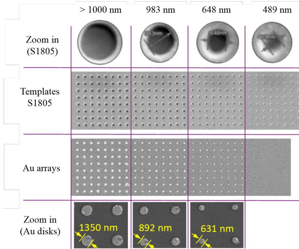
Figure 4.3: SEM images of templates S1805 fabricated at different exposure doses used for evaporation of Au film and corresponding periodic arrays of Au submicrometer disks obtained after lift-off process.
