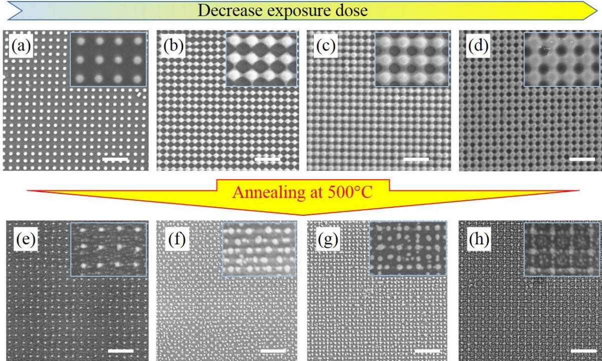
Figure 5.13: (a)-(d) SEM images of template structures (period =  $0.6 \mu\text{m}$ ) fabricated with various filling factors and sputtered with a 10 nm Au layer. (e)-(h) Corresponding GNIA structures obtained after annealing at  $500^\circ\text{C}$ . The scale bar is  $2 \mu\text{m}$ .
