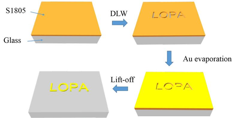
Figure 4.1: Illustration of fabrication process of arbitrary plasmonic structure.
