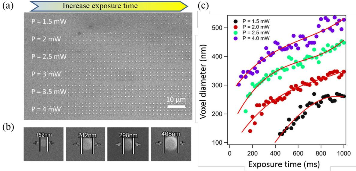
Figure 3.8: (a) SEM images of voxels fabricated on S1805 positive photoresist by DLW technique with different laser powers and different exposure times. (b) Voxels fabricated by an exposure time of 450 ms and different laser powers of 1.5 mW, 2mW, 2.5 mW, and 4 mW, respectively. (c) Dependence of the diameters of the voxels on exposure times and laser powers. Dots are experimental data, and continuous curves are fitting results.
