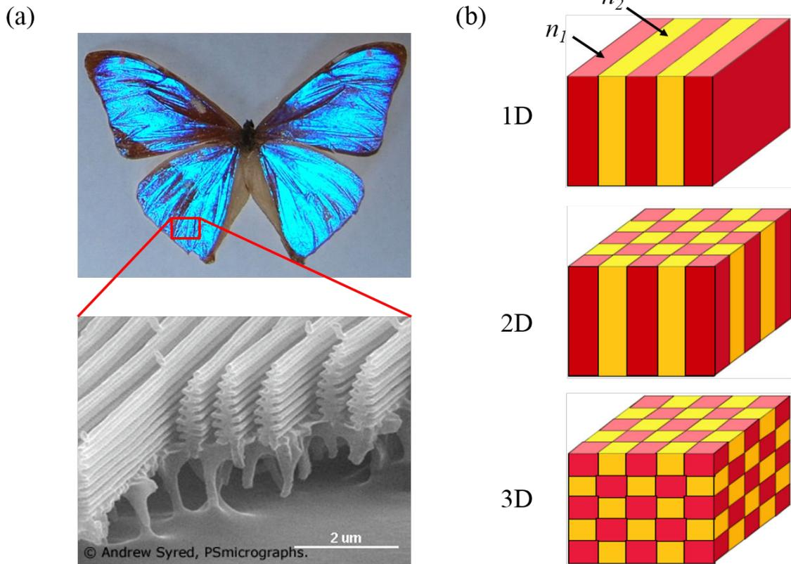
Figure 1.1: (a) A male *Morpho aega* and a SEM image of the wings. Photo from <http://www.microscopy-uk.org.uk/mag/indexmag.html>. (b) Models of 1D, 2D and 3D photonic crystal structures. The colors represent materials with different refractive indices ( $n_1$  and  $n_2$ ).
