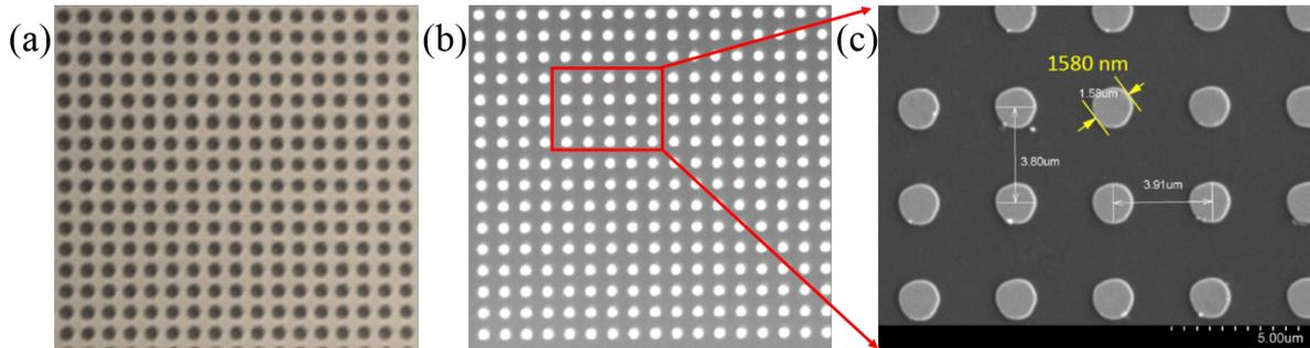
Figure 4.2: (a) Optical microscope image of a polymeric template (2D square structure) used for evaporation of Au film. (b) Periodic array of Au submicrometer disks obtained after lift-off process. (c) A zoom in of Au disks.
