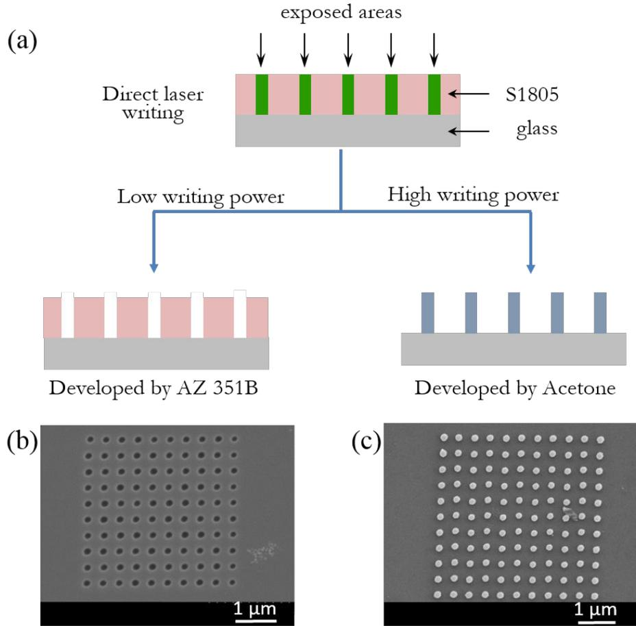
Figure 3.4: (a) Fabrication processes of nanostructures on a positive photoresist. (b) SEM image of a structure written at low power ( $\sim \mu\text{W}$ ) and developed by AZ 351B. (c) SEM image of a structure written at high power ( $\sim \text{mW}$ ) and developed by acetone.
