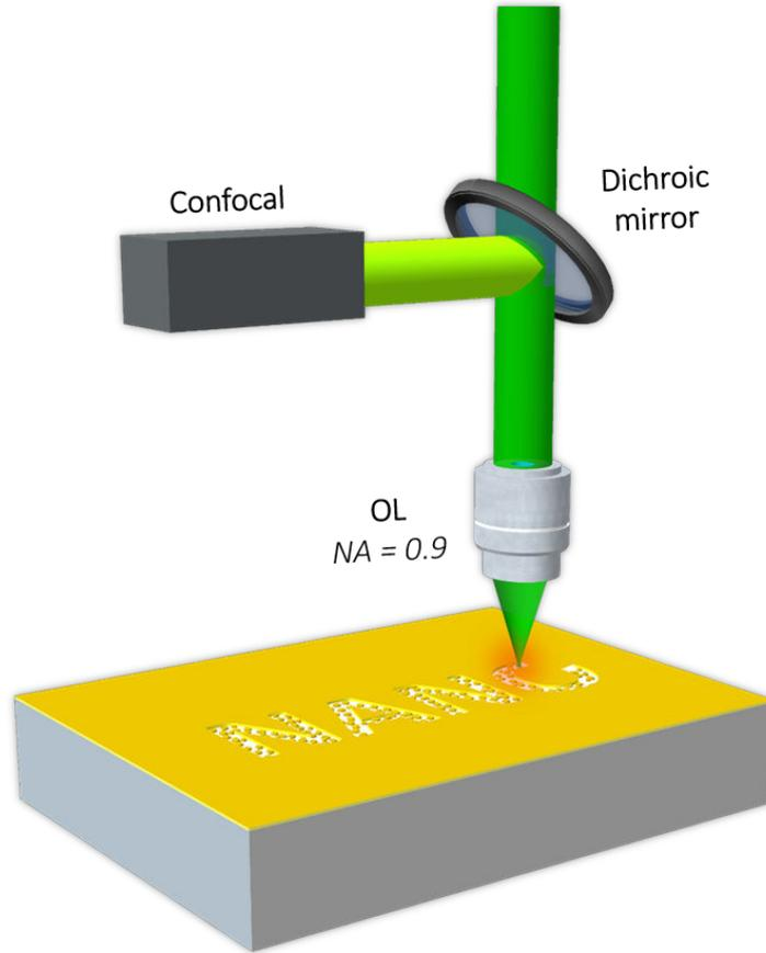
Figure 6.3: Experimental set up of DLW technique used to directly create Au nanostructures by local dewetting effect.
