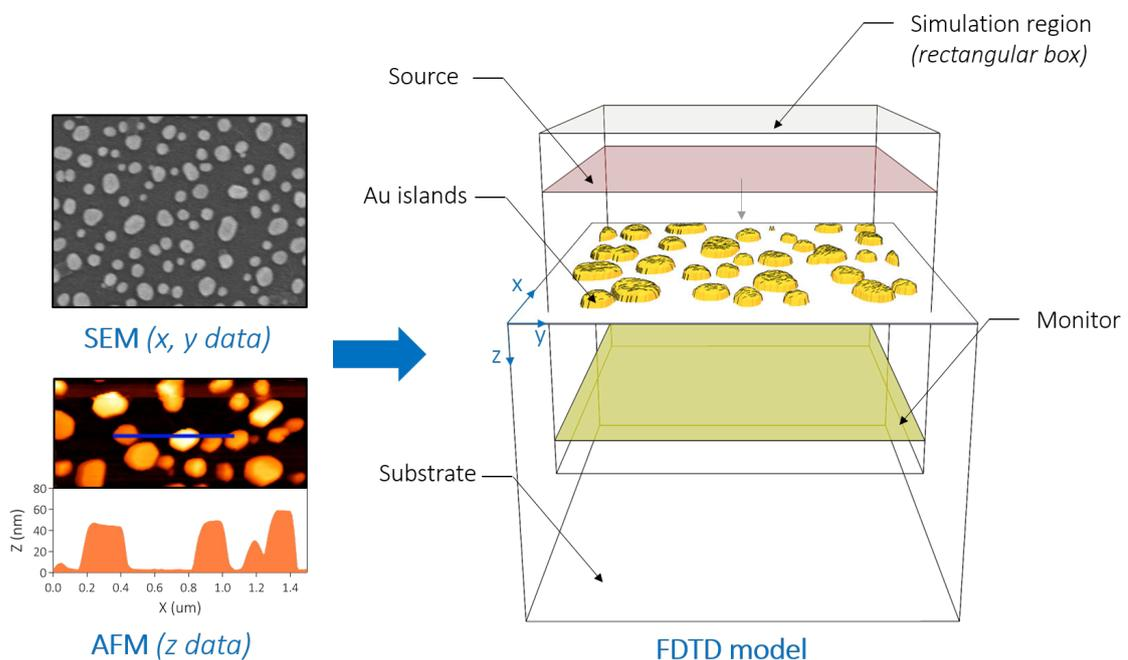
Figure C.1: *FDTD model of Au nano-islands on glass substrate. The Au nano-islands are reconstructed by SEM and AFM data. SEM images provide a large-scale (x,y) data, whilst AFM data is used to estimate the average height of nano-islands.*
