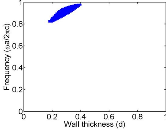
Figure 2.12: A map of PBG as a function of the ring-wall thickness for TM mode of the lattices containing air-rings in a polymeric background  $r = 1.18 \mu\text{m}$ ,  $a = 1.5 \mu\text{m}$ ; refractive index  $n = 1.6$ .
