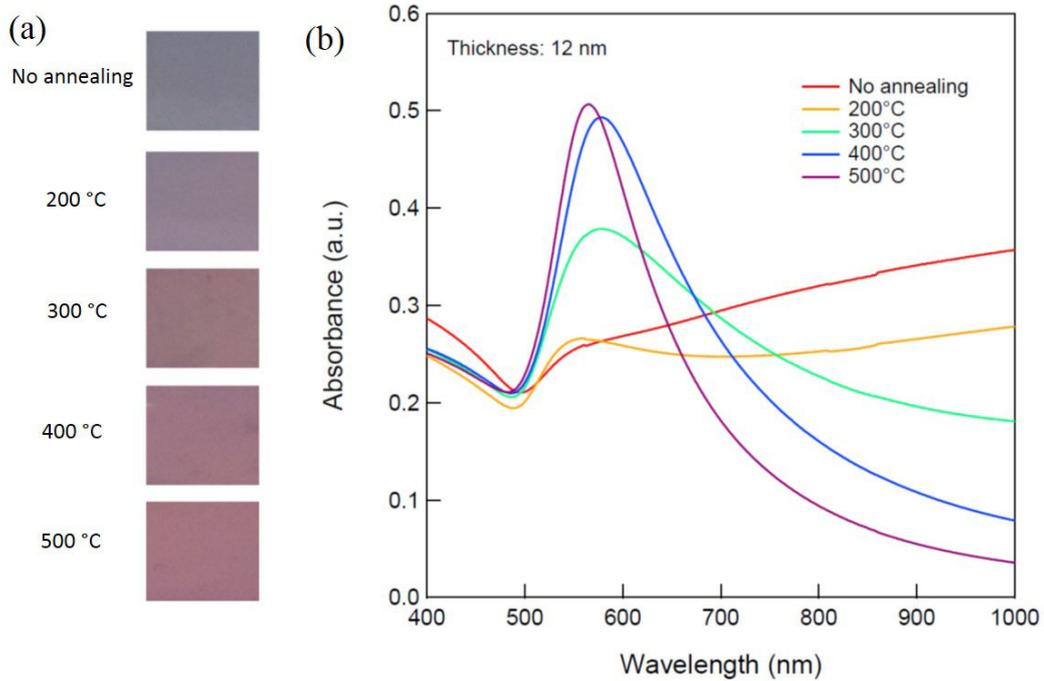
Figure 5.7: Microscope images (a) and UV-VIS spectra (b) of sputtered Au thin films on glass substrate, obtained before and after annealing at different temperatures.
