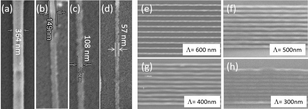
Figure 3.9: (a-d) SEM images of 1D line structures fabricated by different laser powers: 4, 3, 2.5, and 2 (mW). The scanning velocity is fixed at  $10 \mu\text{m/s}$ . (e-h) SEM images of 1D structures with different periods of  $0.6 \mu\text{m}$ ,  $0.5 \mu\text{m}$ ,  $0.4 \mu\text{m}$ , and  $0.3 \mu\text{m}$ , respectively. The exposure power is kept at 2 mW and the scanning velocity is fixed at  $5 \mu\text{m/s}$ . These structures were fabricated with S1805 (thickness = 600 nm).
