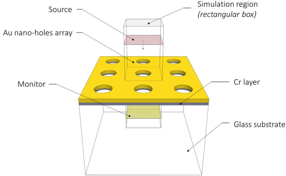
Figure 4.5: Illustration of FDTD model for Au nano-holes array.
