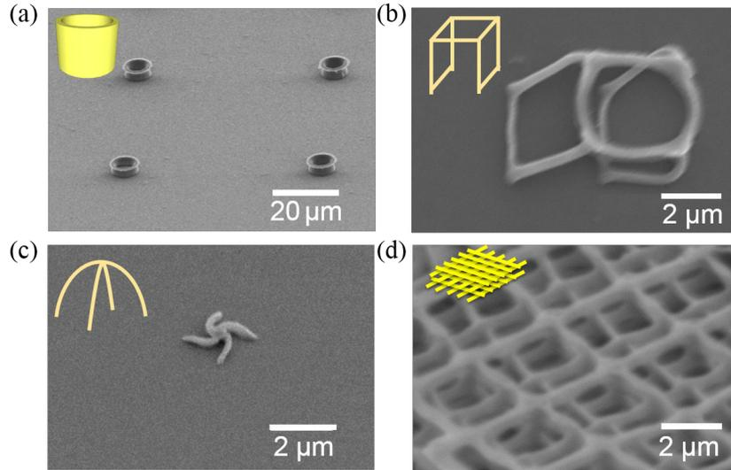
Figure 3.12: SEM images of different 3D structures fabricated by 6 mW in S1818 (thickness =  $6 \mu\text{m}$ ). (a) 3D micro-rings fabricated at a scanning velocity of  $20 \mu\text{m/s}$ . (b)-(d) Different 3D structures fabricated with corresponding designs shown in insets. Fabricated structures are quite soft and are easily to be deformed.
