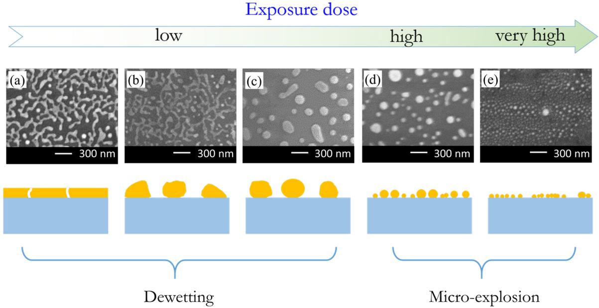
Figure 6.6: Top: SEM images of 12 nm Au island films, sputtered on glass substrate and written by a focused laser beam with 40 mW and different scanning velocities of 40  $\mu\text{m/s}$  (a), 20  $\mu\text{m/s}$  (b), 5  $\mu\text{m/s}$  (c), 2  $\mu\text{m/s}$  (d), and 0.5  $\mu\text{m/s}$  (e). Bottom: Illustrations of Au film morphological transformation as a function of exposure dose.
