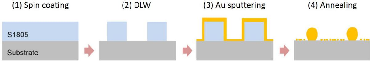
Figure 5.10: Illustration of fabrication process of structured Au arrays by a combination of DLW and thermal annealing.
