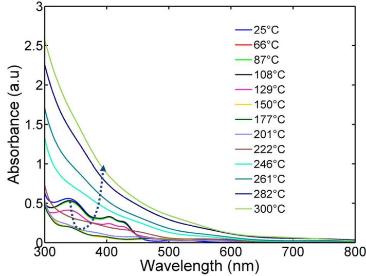
Figure 3.2: The absorbance spectra of the S1805 films annealed at different temperatures (25-500°C) for 5 minutes. The dot arrow indicates the variation of absorption spectra as a function of annealing temperature.
