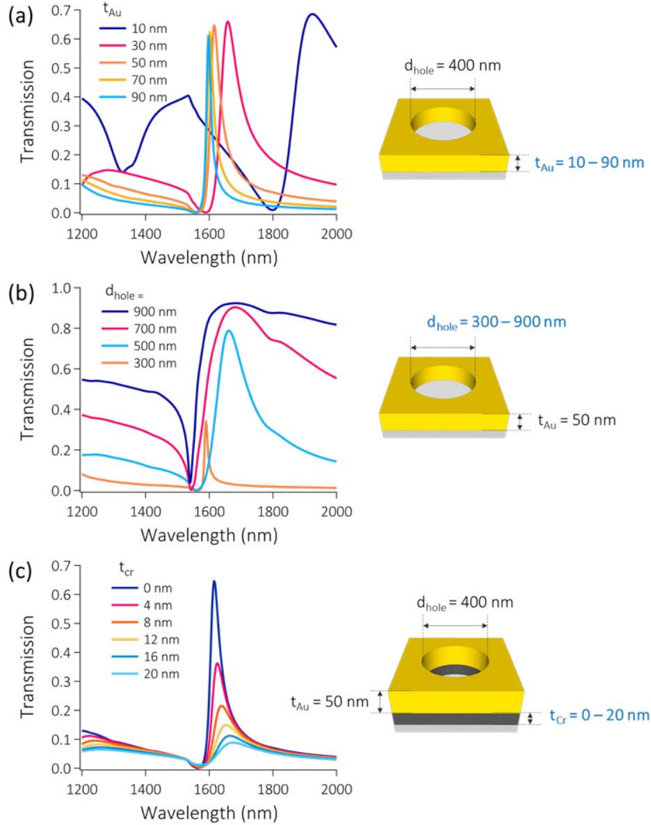
Figure 4.6: Calculated transmission spectra of Au nano-holes array: (a) As a function of Au layer thickness,  $t_{Au}$ ; the diameter of the nano-hole is fixed at  $d_{hole} = 400$  nm; (b) As a function of nano-hole diameter,  $d_{hole}$ ; the thickness of the Au layer is fixed at  $t_{Au} = 50$  nm; (c) As a function of Cr layer thickness,  $t_{Cr}$ ; the thickness of the Au layer and hole diameter are fixed at  $t_{Au} = 50$  nm and  $d_{hole} = 400$  nm, respectively.
