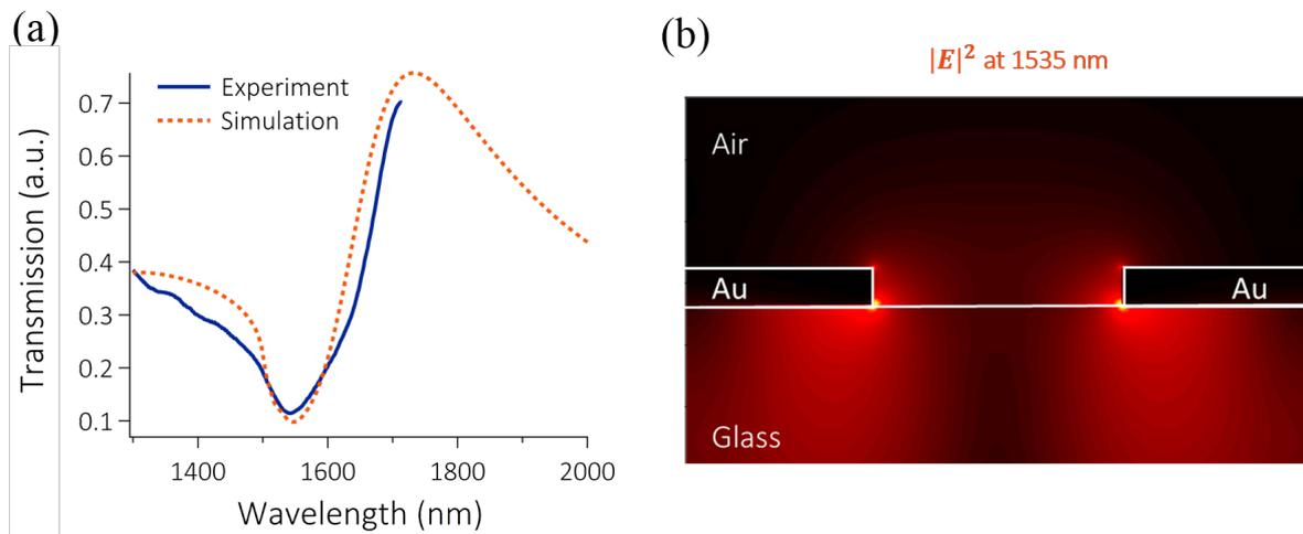
Figure 4.10: (a) Experimental and calculated transmission spectra in air of fabricated Au nano-holes array structures. Parameters for simulation are:  $\Lambda = 1000$  nm,  $d_{hole} = 400$  nm,  $t_{Au} = 50$  nm and  $t_{Cr} = 15$  nm. (b) Simulation of the near field distributions of the electric field intensity (normalized) at wavelength of 1535 nm.
