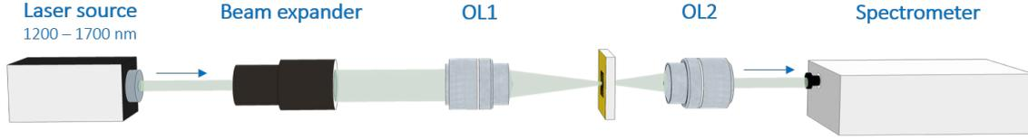
Figure 4.9: Experimental setup of Au nano-holes array transmission measurement.
