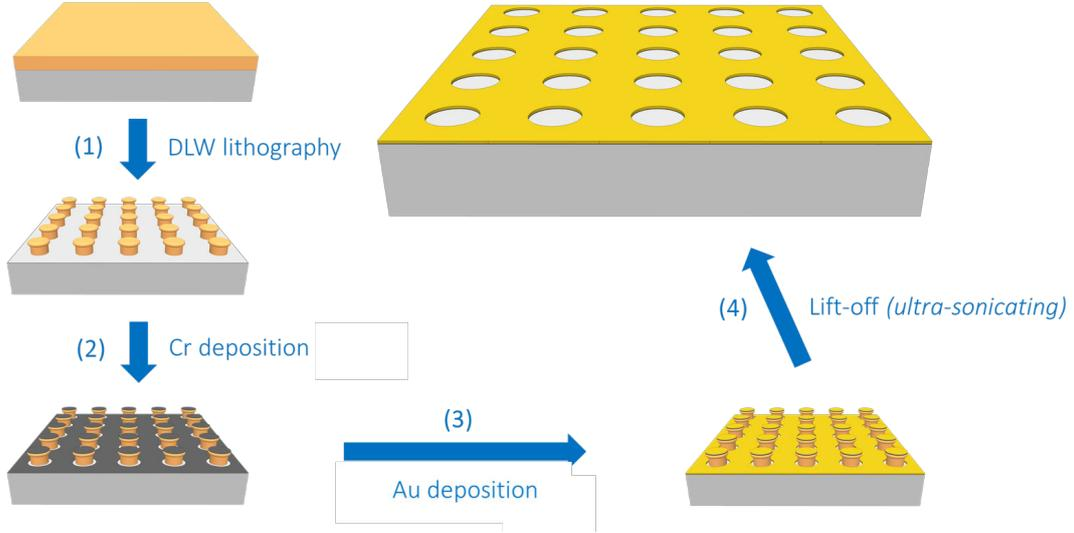
Figure 4.7: Illustration of fabrication process of GNHA structure.
