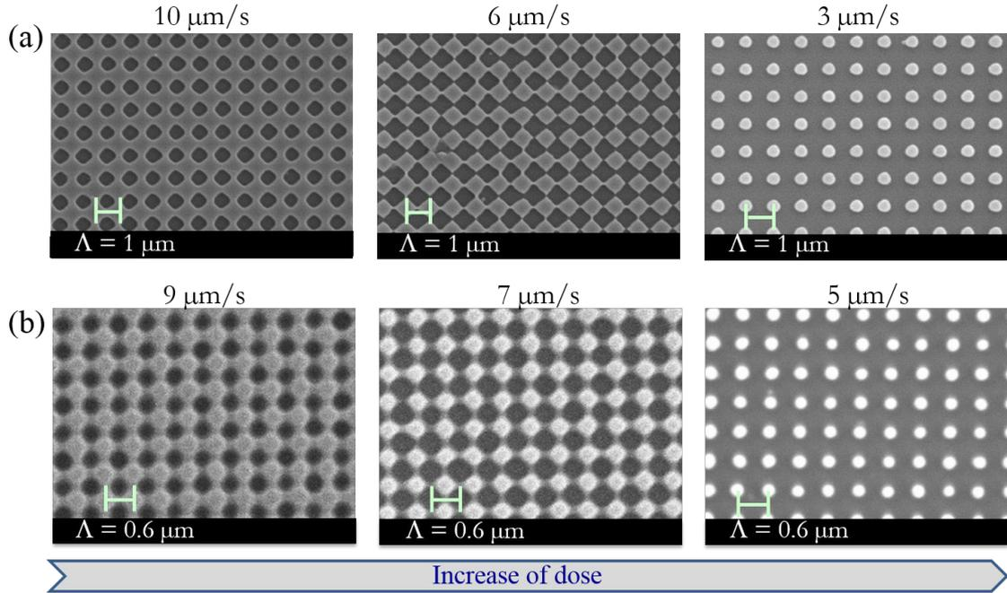
Figure 2.5: (a) SEM images of 2D square structures (period =  $1 \mu\text{m}$ ) fabricated by a laser power of  $15 \mu\text{W}$  and scanning speeds of  $10 \mu\text{m/s}$ ,  $6 \mu\text{m/s}$ , and  $3 \mu\text{m/s}$ , respectively. (b) SEM images of 2D square structures (period =  $0.6 \mu\text{m}$ ) fabricated by a laser power of  $10 \mu\text{W}$  and scanning speeds of  $9 \mu\text{m/s}$ ,  $7 \mu\text{m/s}$ , and  $5 \mu\text{m/s}$ , respectively.
