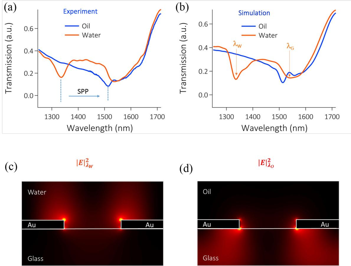
Figure 4.11: (a) Experimental and (b) calculating transmission spectra of fabricated Au nano-holes array structures in different media. Parameters for simulation are:  $\Lambda = 1000$  nm,  $d_{hole} = 400$  nm,  $t_{Au} = 50$  nm and  $t_{Cr} = 15$  nm. Simulations of the near field distributions of the electric field intensity (normalized) (c) at wavelength of 1335 nm in water and (d) at wavelength of 1510 nm in oil medium.
