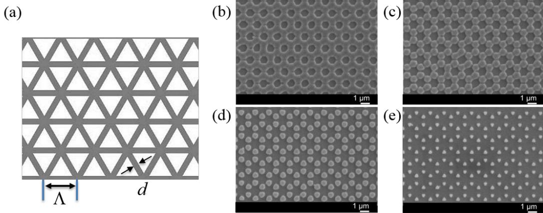
Figure 2.8: (a) The model of a honeycomb lattice created by moving the laser beam following a triangular shape,  $\Lambda$  is the period and  $d$  is track width. (b-e) SEM images of honeycomb lattices (period of  $\Lambda = 1.5 \mu\text{m}$ ) fabricated with a laser power of  $10 \mu\text{W}$  and an average scanning speed of  $9 \mu\text{m/s}$  (b),  $8 \mu\text{m/s}$  (c),  $7 \mu\text{m/s}$  (d),  $6 \mu\text{m/s}$  (e).
