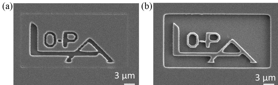
Figure 2.7: 2D arbitrary structures fabricated on S1805 photoresist by a laser power of  $15 \mu\text{W}$  and a scanning speed of  $10 \mu\text{m/s}$ . (a) Negative structure. (b) Positive structure.
