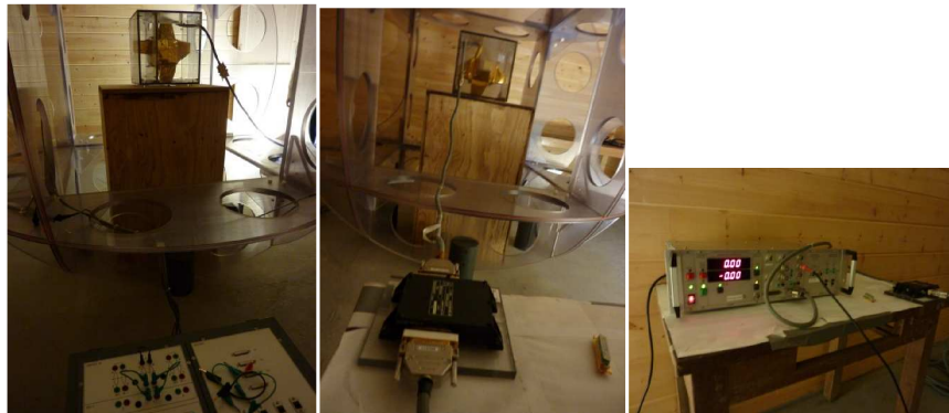
Figure 1 : (Left) Cassini EM sensor located within the new Helmholtz coils inside the new facility. One can see that the YY' coils are connected in the connection panel (on the bottom of the photo) for which the 50 Hz noise is the smallest. (Middle) Cassini EM preamplifier connected to the sensor with the EM harness and connected to the rack GSE2 (Right) Rack GSE2 (+12/-12V power supply) connected to Cassini EM PA. The Y axis (red coaxial cable) is connected to the spectrum analyzer.
