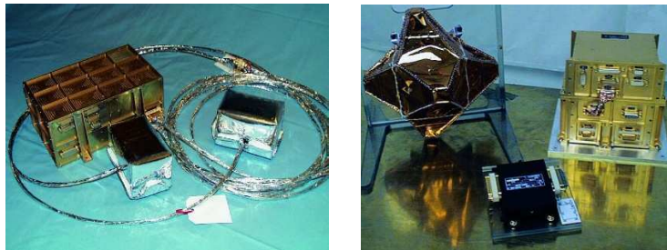
Figure 4.8: Left: FGM instrument ©Imperial College. Right: STAFF covered by the thermal blanket and the preamplifier ©LPP.
