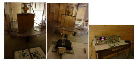
Figure 1: (Left) Cassini EM sensor located within the new Helmholtz coils inside the new facility. One can see that the YY' coils are connected in the connection panel (on the bottom of the photo) for which the 50 Hz noise is the smallest. (Middle) Cassini EM preamplifier connected to the sensor with the EM harness and connected to the rack GSE2 (Right) Rack GSE2 (+12/-12V power supply) connected to Cassini EM PA. The Y axis (red coaxial cable) is connected to the spectrum analyzer.
