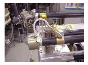
**Figure 5.3:** Flight unit of the FGM instrument (silver-colored cylinder at the foreground) and of the Search Coil Magnetometer (SCM) instrument (3 black colored, orthogonal rods at the background) mounted on their carbon-composite booms. The combination of these instruments measures the ambient magnetic field and its oscillations up to 4 kHz. ©NASA.
