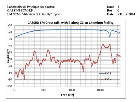
Figure 14: Cross talk between EM Z and EM Y when B is generated along ZZ'.
