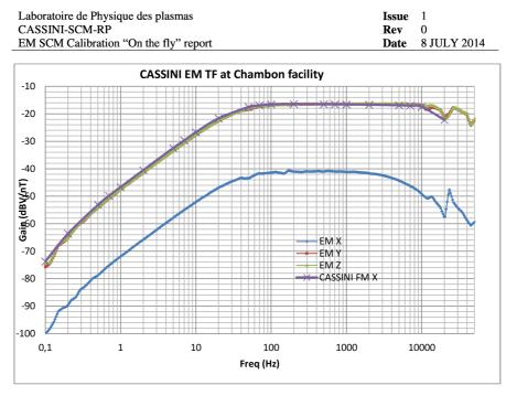
Figure 3: Comparison between Cassini EM (gain) in dBV/nT in the new facility and previous FM measurements (in the previous facility).
