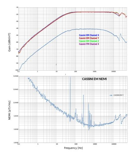
**Figure 4.38:** Top: Comparison between Cassini EM (gain) in dBV/nT at Chambon-la-Forêt facility and the previous FM measurements (back in the 90's in a different facility). Bottom: Cassini EM ground noise level (NEMI). The observed peaks correspond to the harmonics of the 50 Hz fundamental waveform.
