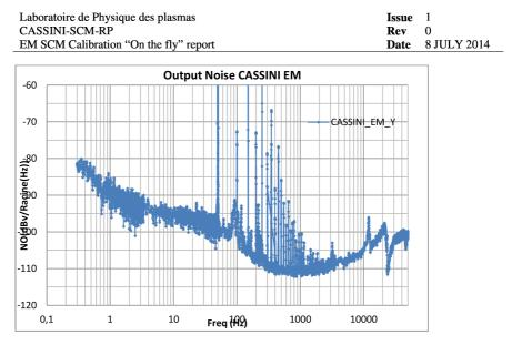
Figure 10: Cassini EM Output noise in dbV/sqrt(Hz). 50 Hz tone and harmonics are still present despite the fact that the sensor and the pa are in the mumetal box and the rack has been covered by mumetal tops.
