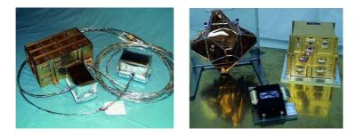
**Figure 4.8:** Left: FGM instrument ©Imperial College. Right: STAFF covered by the thermal blanket and the preamplifier ©LPP.
