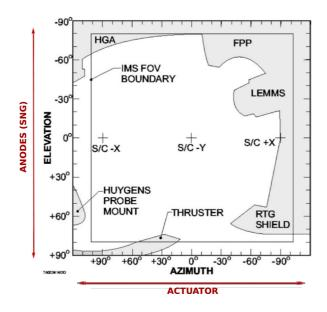
**Figure 4.30:** All-sky projection of the CAPS-IMS field of view (FoV). The shaded areas represent surrounding spacecraft instruments obscuring the CAPS FoV. Similar encroachments occur for IBS and ELS. Adapted from Young *et al.* [2004].
