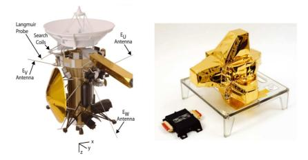
**Figure 4.4:** Left: The placement of the different RPWS hardware on Cassini Orbiter. Right: The tri-axial magnetic search coils assembly covered by thermal blankets. Adapted from Gurnett *et al.* [2004].
