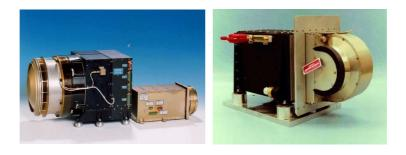
**Figure 4.9:** Left: The CODIF (on the left) and the HIA (on the right) ion detectors of the CIS experiment ©IRAP. Right: PEACE instrument sensor ©MSSL.
