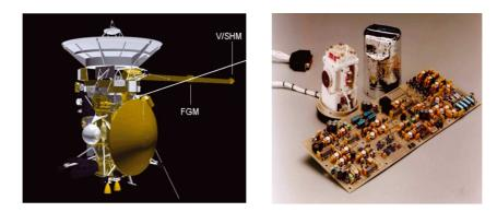
**Figure 4.3:** Left: The location of the magnetometer hardware on the spacecraft is shown halfway the "mag boom". Right: Electronics photograph of the FGM (with cover off) and electronics board. Adapted from Dougherty *et al.* [2002].
