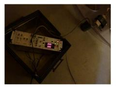
Figure 2: Rack GSE2 (+12/-12V power supply) connected to Cassini EM PA and located to the mumetal box in order to reduce the 50Hz tone produced by the power supply. The mumetal box is grounded to the rack ground. The Y axis (red coaxial cable) is connected to the spectrum analyzer.
