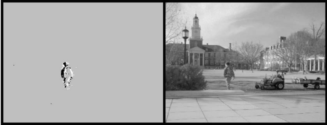
Figure 2.3: Example output from the ATIS sensor showing the TD output (left) and the EM output (right) for a typical outdoor scene [3]. The scene represents a person walking away from the camera, with the background remaining static. The TD image on the left was constructed by buffering all events over a fixed time period and displaying a black or white dot for pixels which have recently experienced an increase or decrease in intensity respectively. The EM image on the right shows the absolute pixel intensity, which receives pixel value updates whenever the TD circuit detects a change.
