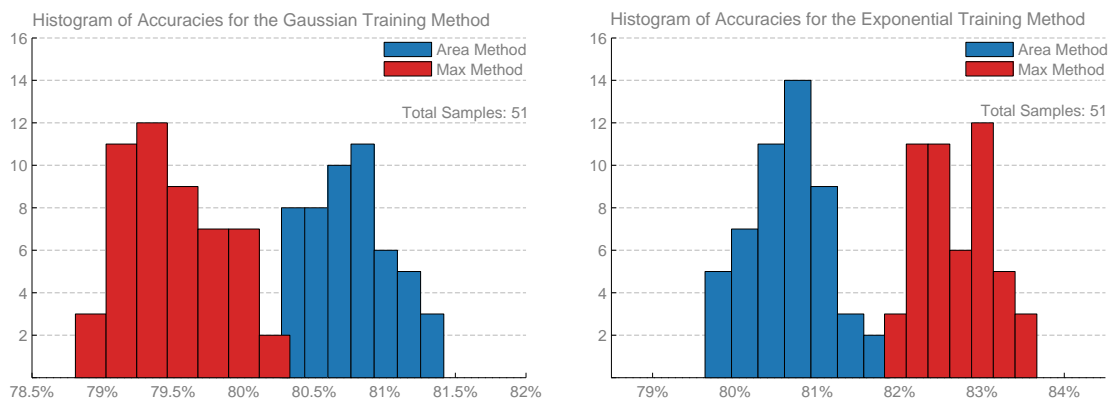
Figure 4.15: Histograms of accuracies showing the comparison between the Gaussian and Exponential training patterns under the Max and Area determination methods. The figure shows the histograms of accuracies obtained when using the Exponential and Gaussian patterns under the Max and Area output determination methods. It serves to demonstrate the important link between training method and output determination method. It is clear that the Exponential training method is a better choice when using the Max output determination method. This is of particular importance as the Max output determination method represents the easiest method to implement in hardware.
