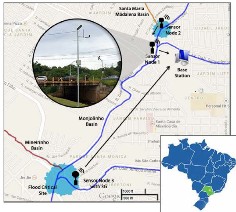
Figure 3 - Deployment layout of the flood monitoring system in a flood-prone area in downtown São Carlos, Brazil (adapted from [70])
