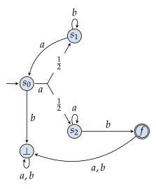
Figure 8: A probabilistic automaton with value 1
