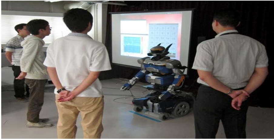
Figure 1.6: Typical CASA application: a robot quiz-master is able to locate, separate and process sound sources in a controlled environment [NIYO15].
