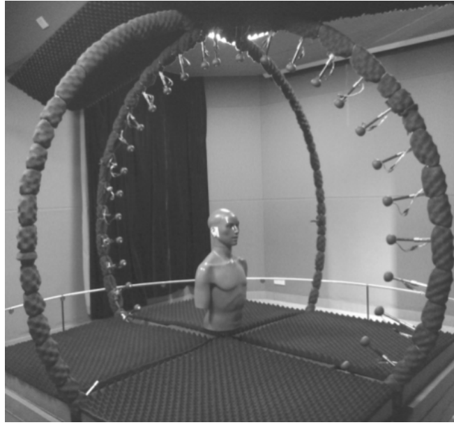
Figure 2.12: Typical material required for HRTF measurements [ZX14]. In this solution the measurements are performed from two rings of speakers that rotate according to azimuth and elevation angles.
