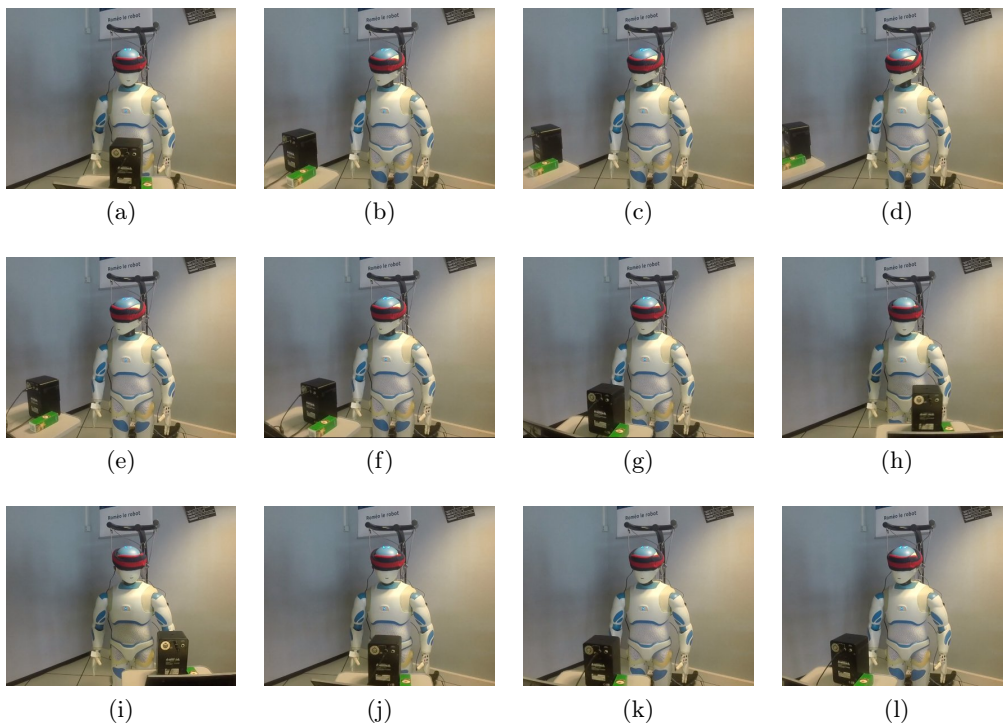
Figure 6.7: Tracking a continuously moving sound source from (a) to a final pose in (d) using ITD cues on Romeo .
