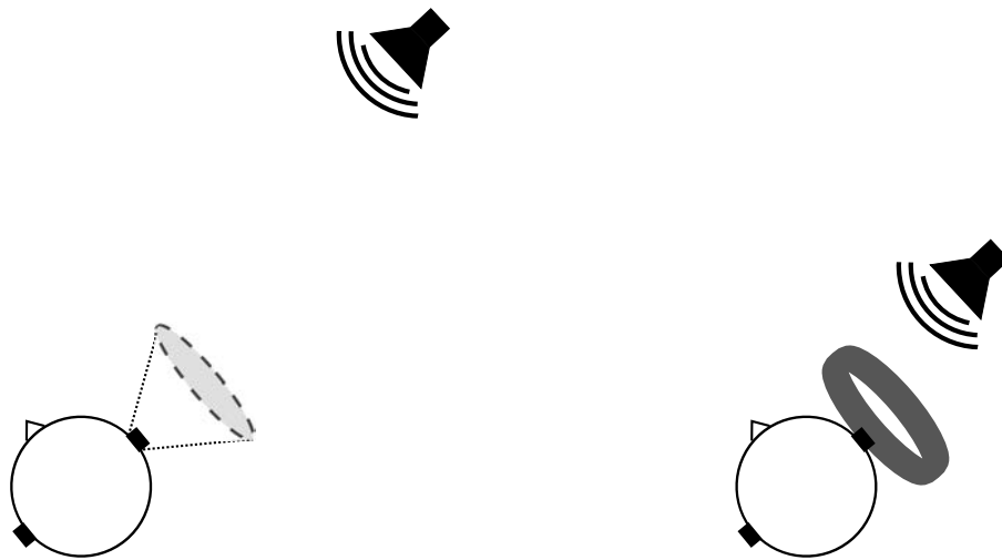
Figure 2.7: In the far field, localization based on interaural cues lead to a cone of confusion. In the near field the cone of confusion degenerates into a torus of confusion (black donut) principally because of the action of ILDs ( i.e. intersection of the cone and a sphere ).
