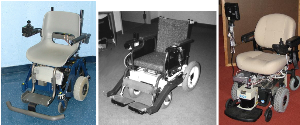
Figure 2.1: Evolution of Robotic Wheelchairs. The Wheelesley from MIT, 1996 (left), The TAO project wheelchair, 1998 (middle), and the MIT Intelligent Wheelchair Project, 2010 (right). Early intelligent wheelchair designs were robots built from the ground up or adapted by rigidly attaching a chair on a mobile robot base.
