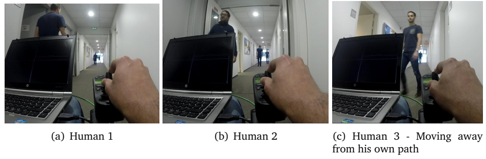
Figure 7.10: Frames captured during one of the tests that depict encounters of the wheelchair with humans while following a corridor.
