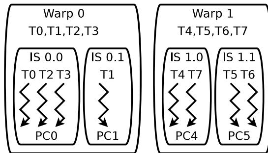
Figure 3.3: Logical organization of hardware threads on 2-warp  $\times$  4-thread DITVA. Scalar threads are grouped into 2 warps of 4 threads. Scalar threads sharing the same PC within a warp form an Instruction Stream (IS).
