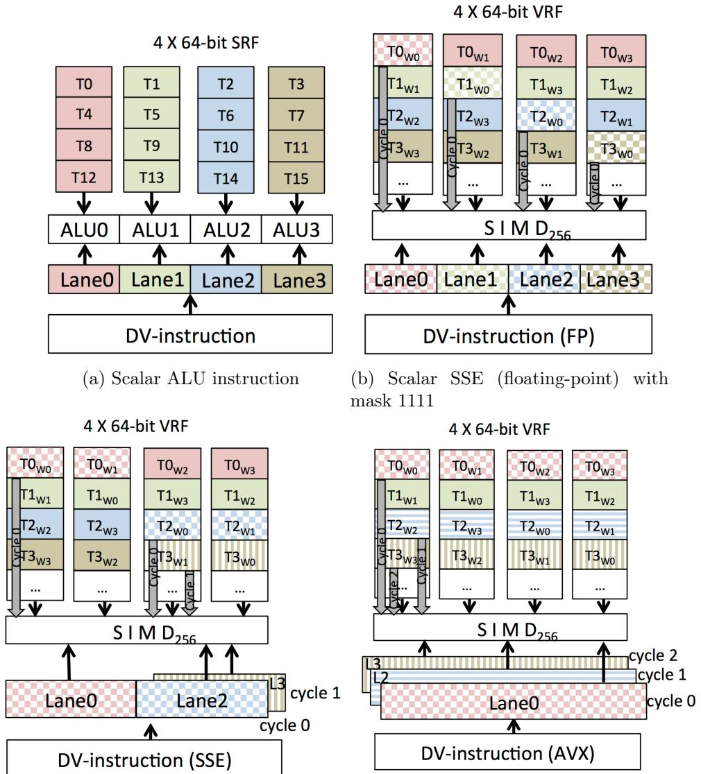
Figure 3.9: Operand collection on  $4W \times 4T$  DITVA depending on DV-instruction type and execution mask. 'w' represents a 64-bit word
