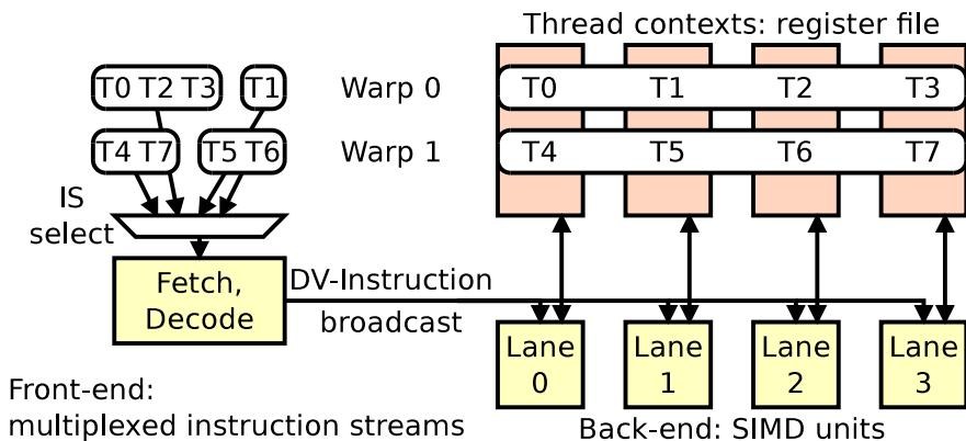
Figure 3.4: Thread mapping to the physical organization.
