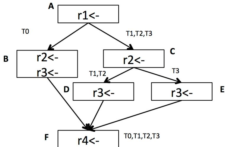
Figure 5.2: Program control flow for threads T0,T1,T2 and T3.  $<-$  represents write to a register.
