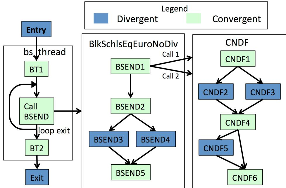
Figure 2.1: Control flow graph of blackscholes benchmark
