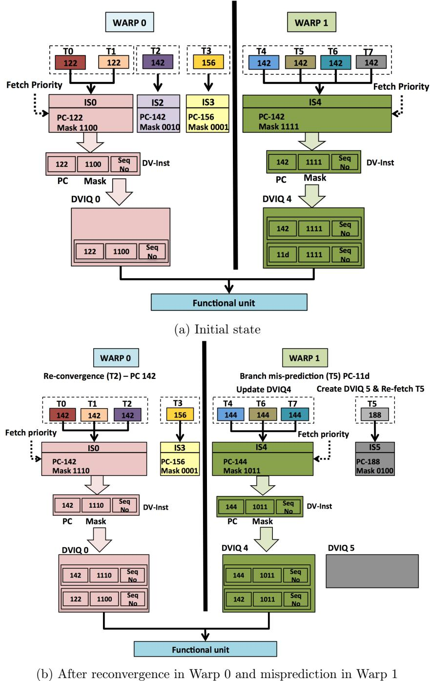
Figure 3.10: Evolution of the IS and DVIQ states upon thread divergence and reconvergence
