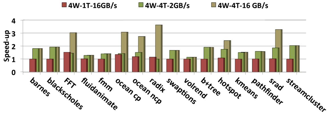
Figure 4.6: Performance scaling with memory bandwidth, relative to 4-thread SMT with 2 GB/s DRAM bandwidth
