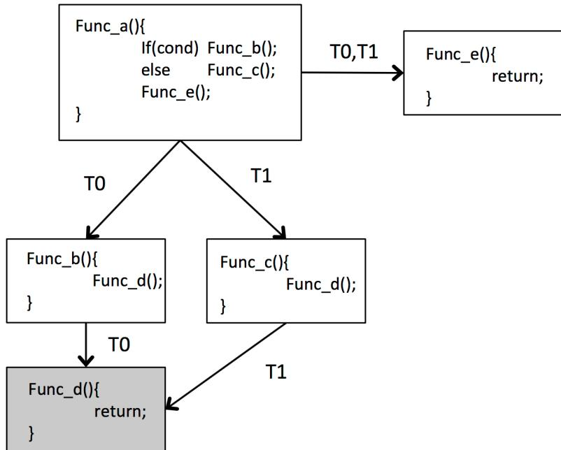
Figure 2.6: Control flow with synchronization point at Func\_d
