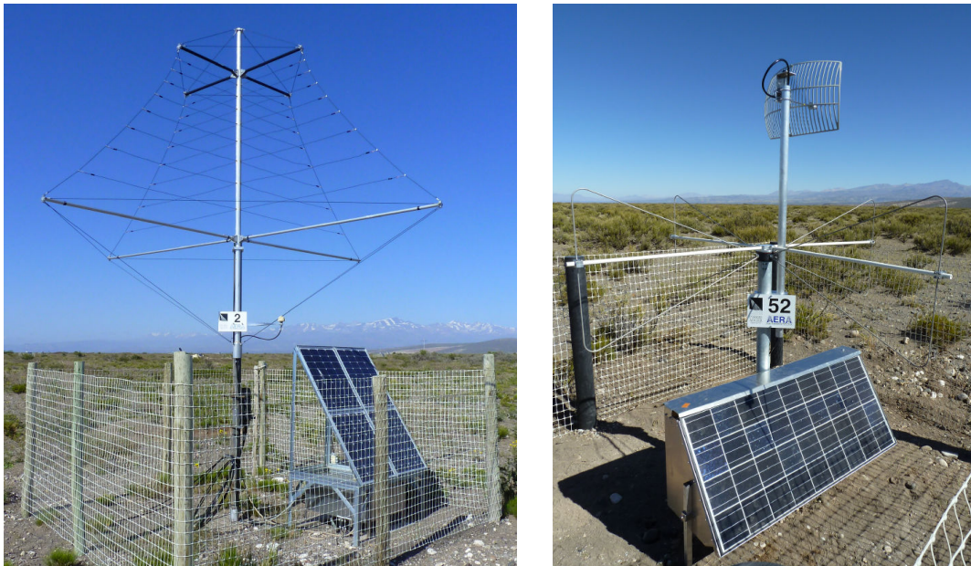
Figure 2.9: Left: a logarithmic periodic dipole antenna (LPDA) installed at AERA (phase one). Right: butterfly antennas installed during phase two or three. Both set up have two horizontal polarizations.
