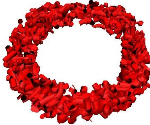
FIGURE 6.2: Local polarization field lines at T = 450 K for a torus included in a 38 \times 38 \times 9 box.
