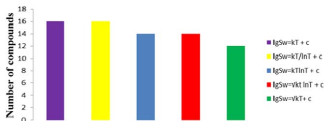
Figure 1. The best fitting equations and maximum number of compounds for which temperature dependence of solubility is described appropriately according to F -test value. [Color figure can be viewed in the online issue, which is available at wileyonlinelibrary.com .]
