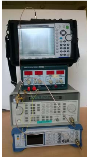
Figure 2.22: The circuit inter-modulation measurement set up.
