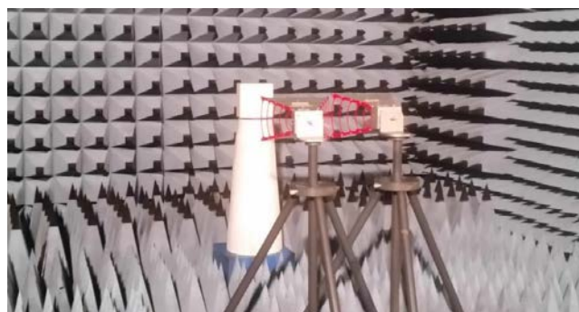
FIG. 2.7 Photo of measurement configuration for normal incidence in anechoic chamber of IETR localized at INSA, Rennes, France
