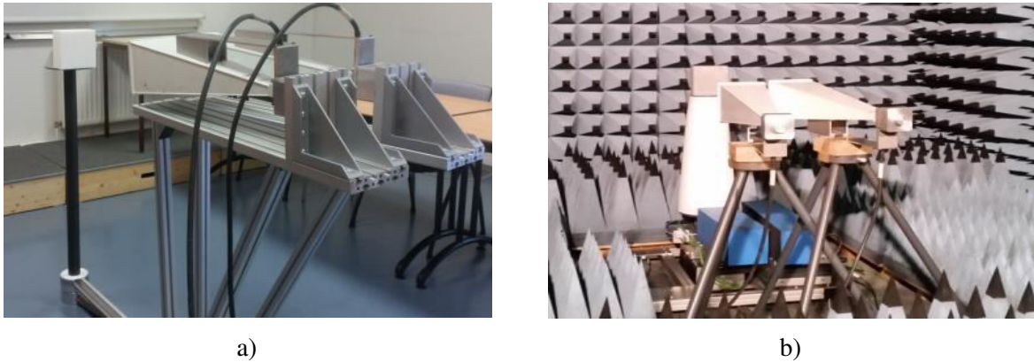
FIG. 1.14 Measurement configurations in a) a multipath environment and b) in anechoic chamber
