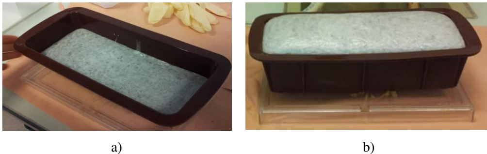
FIG. 2.4 a) The mixture composite put in the mold and b) the mixture composite after foaming step
