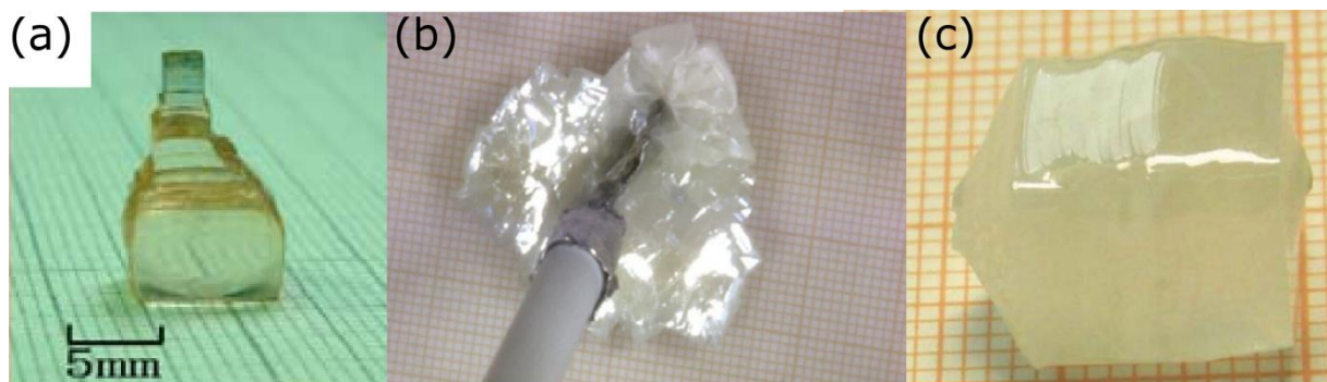
Figure 2.20. Examples of as-grown crystals: (a) colorless cubic KNTN (TSSG) [178], (b) KNLTNS (SSSG) [46], and (c) KNTN (TSSG) single crystals [179]. Reprinted from Ref. [46,178,179], with permission of Elsevier Masson, Springer, and Royal Society of Chemistry.
