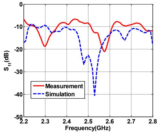
Figure III-32: Simulated and measured return losses of the FP OAM antenna (array radius equals to 60 mm)
