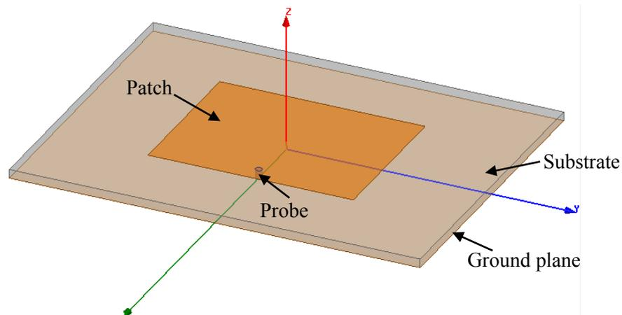
Figure II-1: 3D model of a single patch antenna
