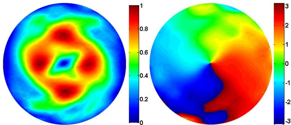
Figure III-29: Normalized magnitude (left) and phase (right) patterns of  $E_x$  component for the second FP OAM antenna at 2.5 GHz, plotted on a circular area with a radius of 300 mm, lying 30 mm above the PRS
