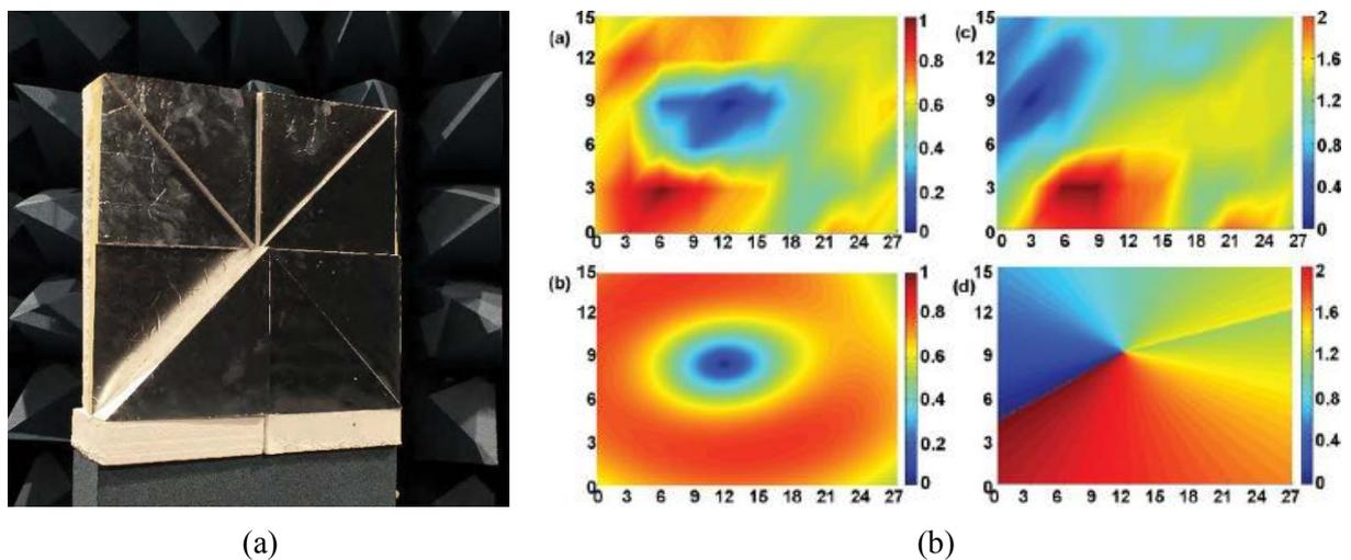
Figure I-21: Generation of radio OAM waves with a spiral reflector: (a) view of the realized reflector; (b) measured (top) and simulated (bottom) results [26]
