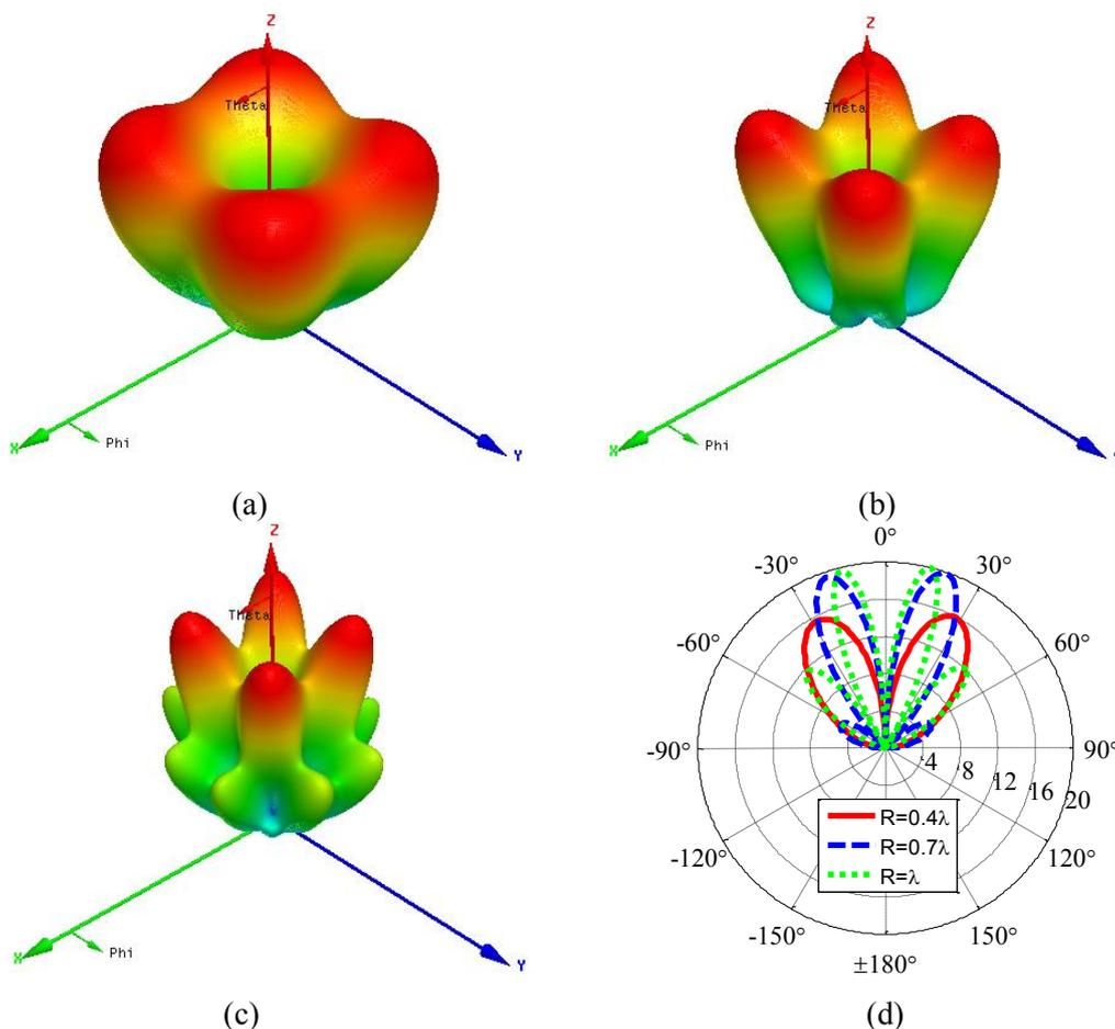
Figure II-11: 3D and 2D radiation patterns for OAM mode  $\ell = 1$  with different array radiuses at 2.5 GHz: (a)  $R = 0.4\times\lambda$ ; (b)  $R = 0.7\times\lambda$ ; (c)  $R = \lambda$ ; (d) E-plane radiation pattern.
