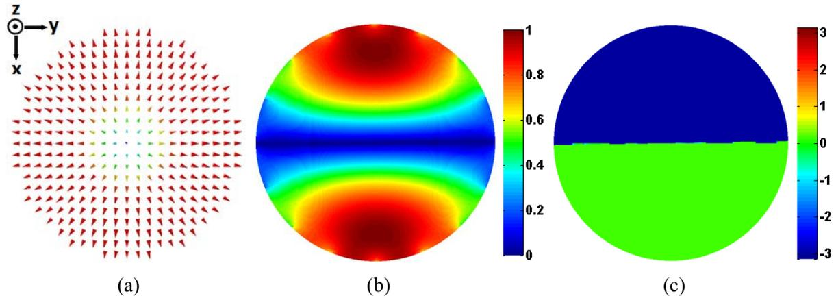
Figure IV-14: Field distribution of  $TM_{01}$  mode and the corresponding magnitude and phase patterns of  $E_x$  component: (a) Field distribution; (b) Normalized magnitude pattern; (c) Phase pattern.
