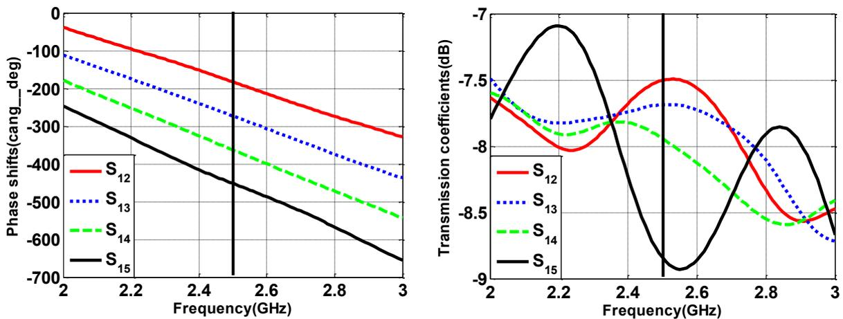
Figure III-15: Simulated parameters of the phase shifter-power divider: phase shifts (left) and transmission coefficients (right). At 2.5 GHz, the phase shifts of  $S_{21}$ ,  $S_{31}$ ,  $S_{41}$ ,  $S_{51}$  are  $-182^\circ$ ,  $-273^\circ$ ,  $-363^\circ$ ,  $-452^\circ$ , respectively; and the corresponding amplitudes are  $-7.5$  dB,  $-7.7$  dB,  $-7.9$  dB,  $-8.8$  dB.
