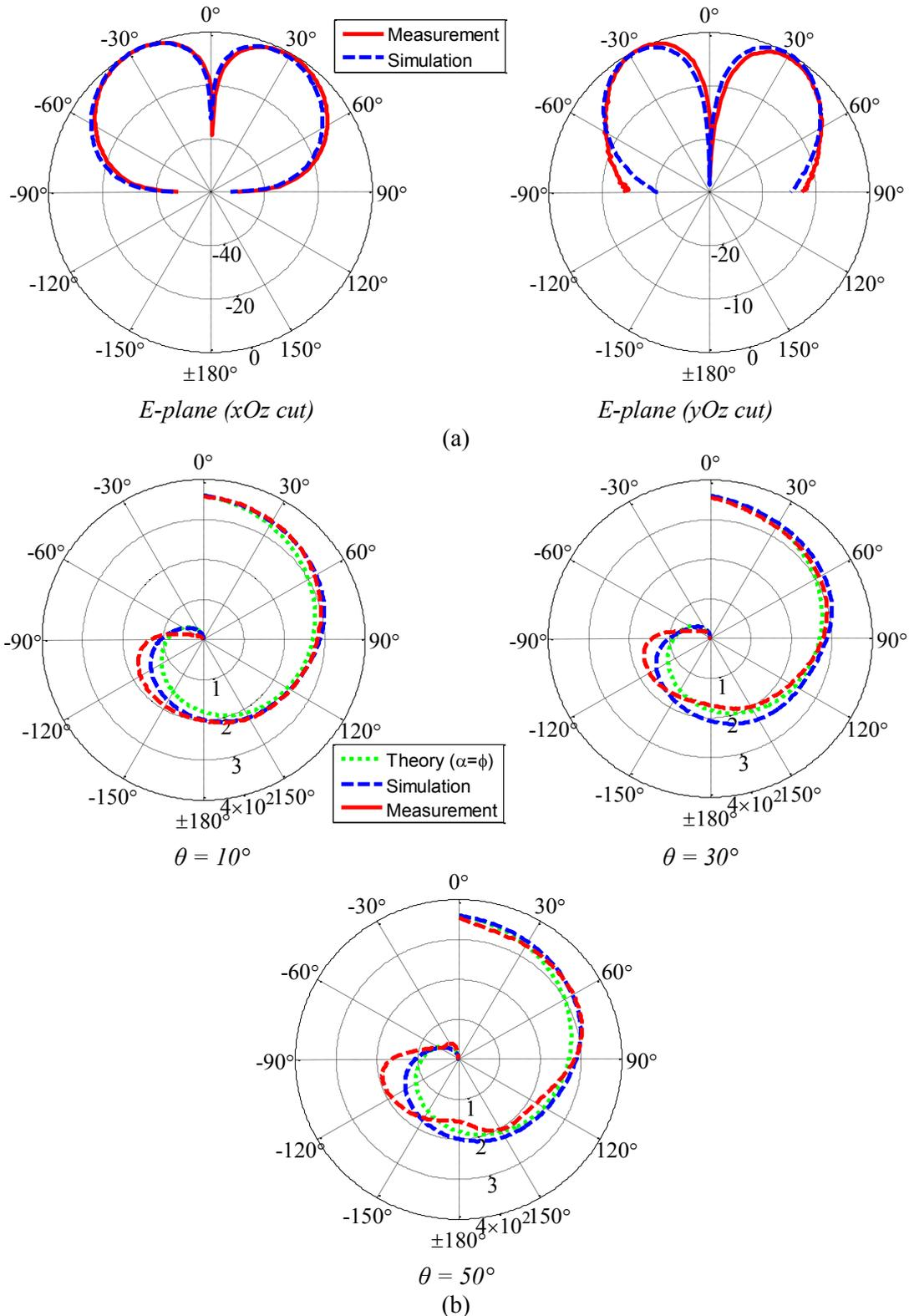
Figure II-20: Simulated and measured 2D radiation and phase patterns of the OAM antenna at 2.5GHz: (a) Normalized magnitude patterns; (b) Normalized phase patterns (in degree).
