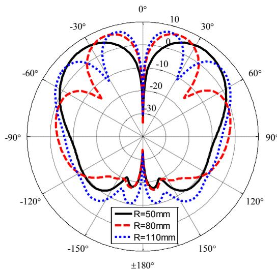
Figure III-7: E-plane radiation patterns with different array radiuses  $R$  at the frequency of 2.5 GHz
