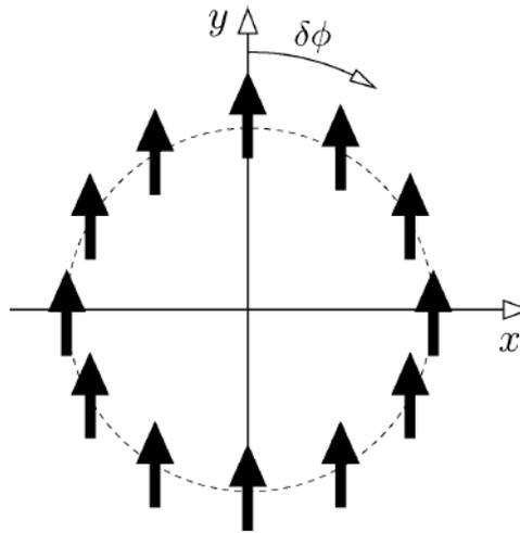
Figure I-23: Configuration of a circular antenna array ( $N = 12$ , dipoles) for generating waves bearing OAM. The phase shift  $\delta\phi$  between two neighboring antennas is defined in (I-17) [5].
