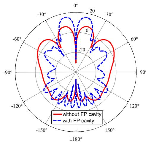
Figure III-13: Comparison of E-plane radiation patterns of the OAM antenna with and without FP cavity (array radius equals to 110mm) (width of strips: 4 mm, period of strips: 20 mm, cavity thickness: 58 mm, cavity aperture: 600 mm  $\times$  600 mm)
