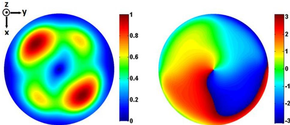
Figure IV-19: Normalized magnitude (left) and phase (right) patterns of  $E_x$  component for the OAM horn antenna with two half-turn SPPs at the frequency of 7.4 GHz (based on  $TM_{01}$  mode) (observation window: circular area with a radius of 7 cm, lying 1 cm above the horn aperture)
