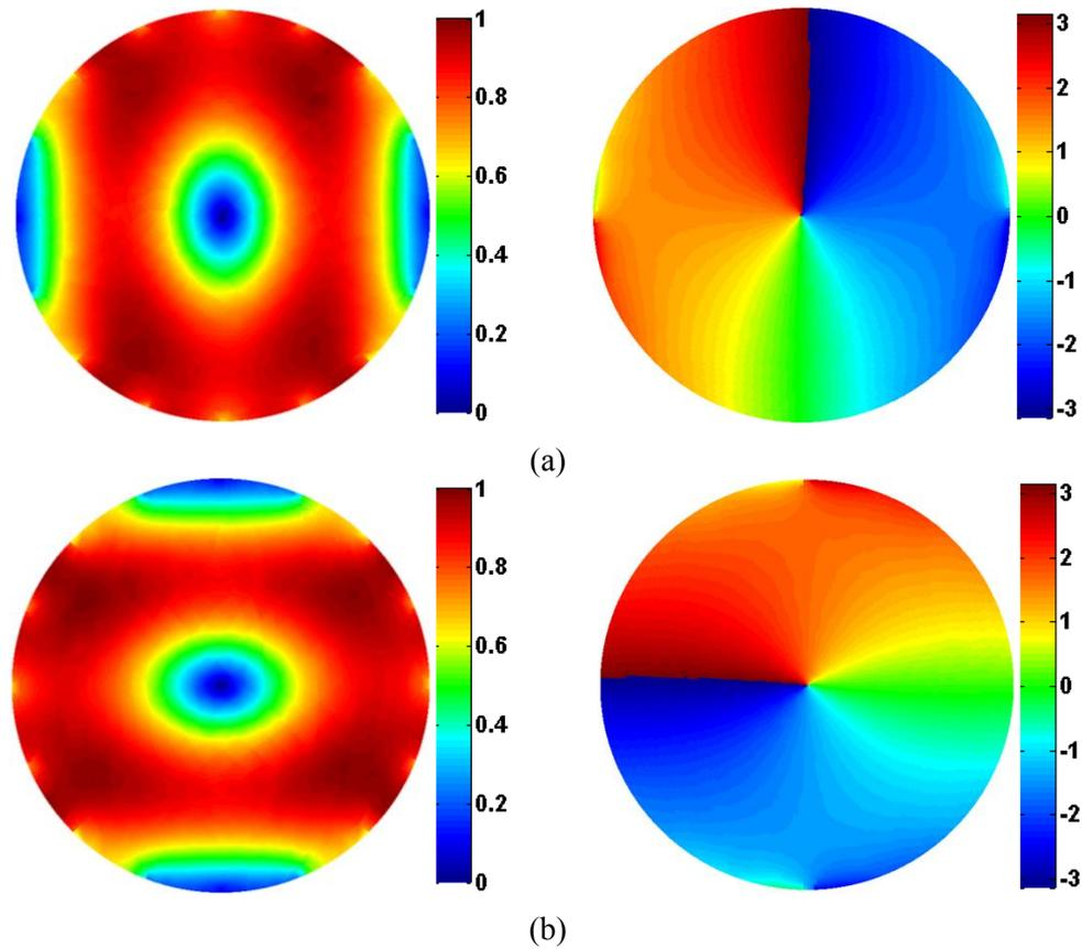
Figure IV-29: Magnitude (left) and phase (right) patterns of the combined  $TM_{01}$  and  $TE_{21}$  modes: (a)  $E_x$  component; (b)  $E_y$  component
