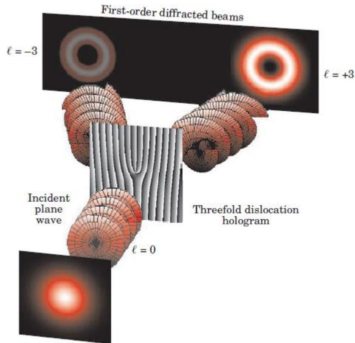
Figure I-9: A pair of helically phased waves with  $\ell = \pm 3$  transformed from a plane wave using a hologram [50]
