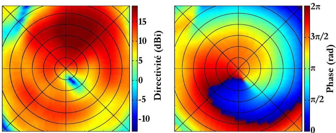
Figure I-16: Magnitude (left) and phase (right) patterns generated by the OAM horn antenna with the flat drilled phase plate [23]
