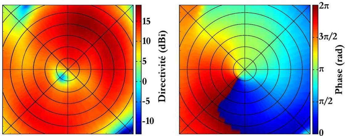
Figure I-11: Magnitude (left) and phase (right) patterns generated by the OAM horn antenna with the SPP at 30 GHz [23]
