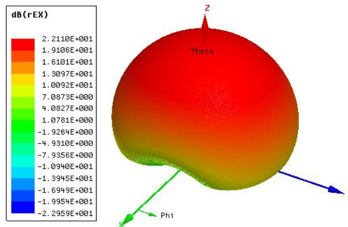
Figure II-3 Simulated 3D radiation pattern of a single patch antenna
