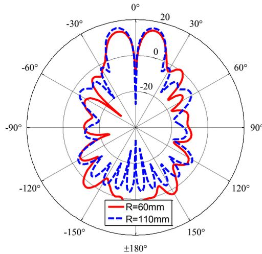
Figure III-30: Comparison of E-plane radiation patterns of the FP OAM antenna with different array radiuses
