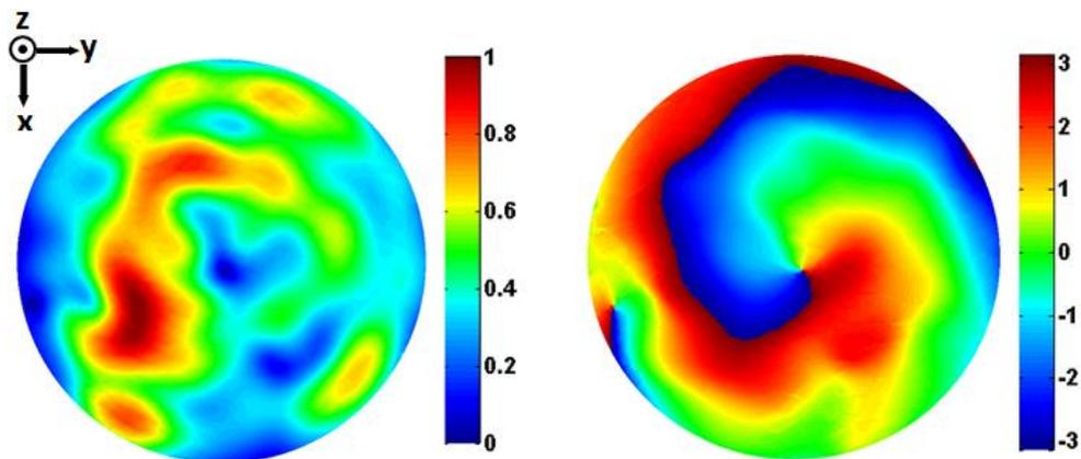
Figure IV-12: Normalized magnitude (left) and phase (right) patterns of  $E_x$  component for the OAM horn antenna with a single SPP at the frequency of 20 GHz (observation window: circular area with a radius of 5 cm, lying 2 cm above the horn aperture)
