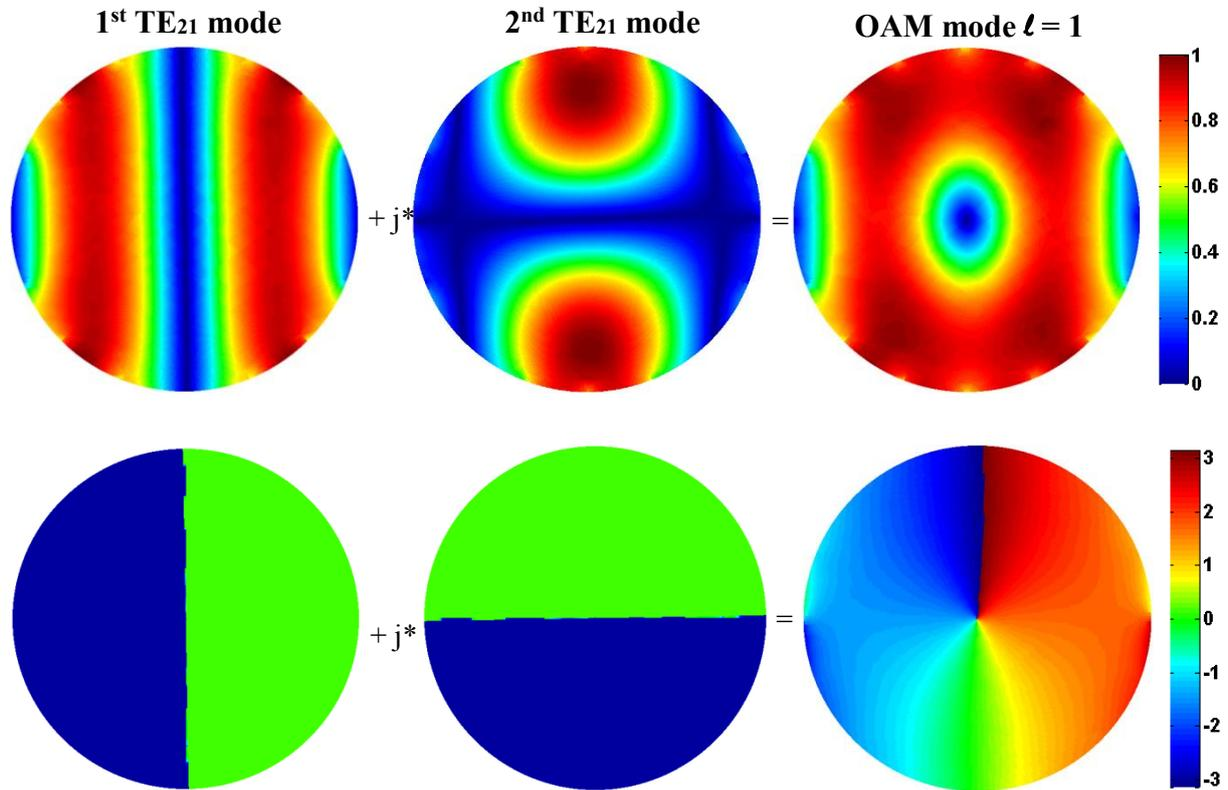
Figure IV-27: Evolutions of magnitude (top) and phase (bottom) patterns of  $E_x$  component for the generation of an OAM wave, by combining two kinds of  $TE_{21}$  modes with a  $\pi/2$  phase difference
