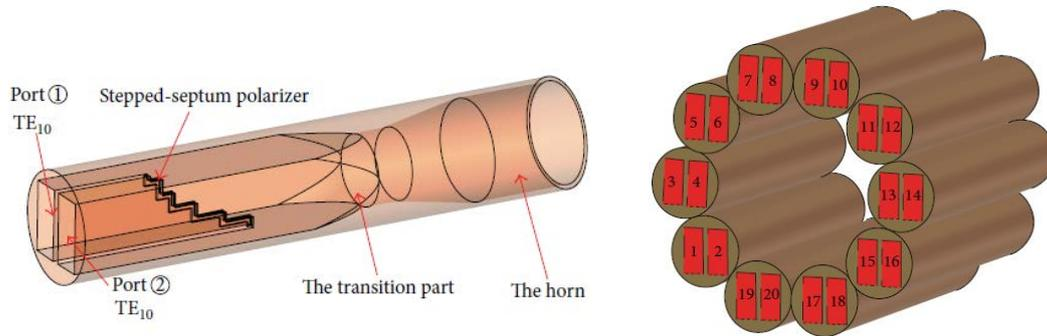
Figure I-29: Configuration of single horn antenna (left) and geometry of the horn antenna array (right) [30]
