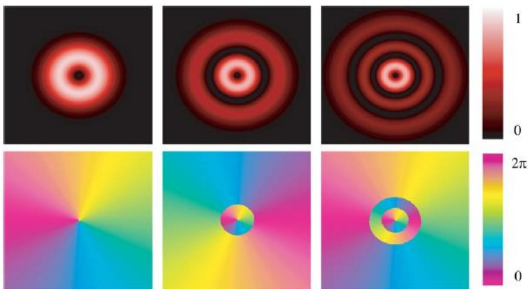
Figure I-3: Normalized intensity (top) and phase (bottom) plots of LG modes:  $\text{LG}_{01}$ ,  $\text{LG}_{11}$ , and  $\text{LG}_{21}$  (left to right) showing the  $p + 1$  concentric rings and the effect on the phase pattern [38]
