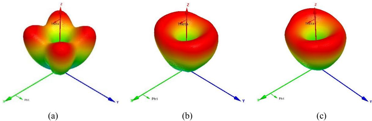
Figure II-8: 3D radiation patterns for OAM mode  $\ell = 1$  with different numbers of array elements at 2.5 GHz: (a)  $N = 4$ ; (b)  $N = 6$ ; (c)  $N = 8$ .
