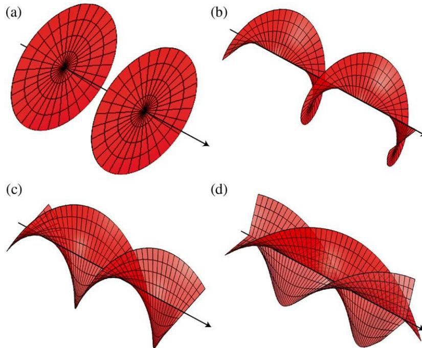
Figure I-4: Plane phase front for (a)  $\ell = 0$  and helical phase fronts for (b)  $\ell = 1$ ; (c)  $\ell = 2$ ; (d)  $\ell = 3$  [38]
