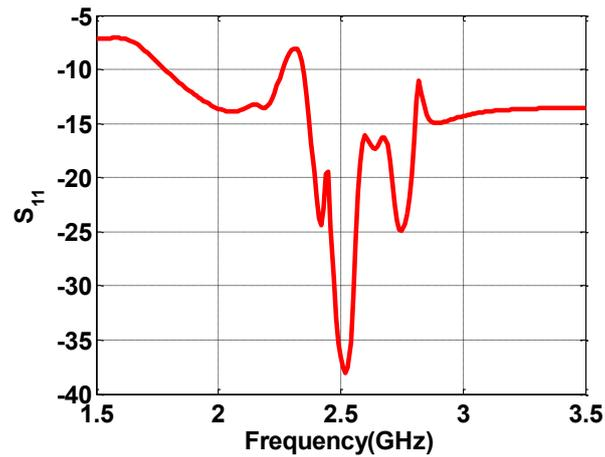
Figure III-17: Reflection coefficient of the FP OAM antenna with phase shifter-power divider
