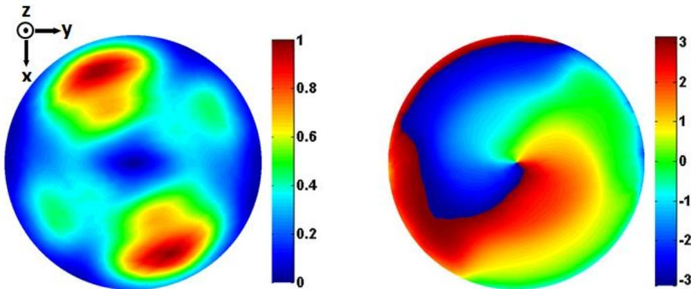
Figure IV-25: Normalized magnitude (left) and phase (right) patterns of  $E_x$  component for the OAM horn antenna with two half-turn SPPs at the frequency of 10 GHz (based on  $TE_{21}$  mode) (observation window: circular area with a radius of 6 cm, lying 1 cm above the horn aperture)
