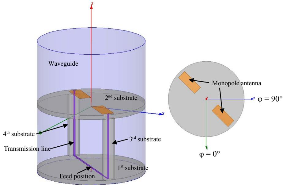
Figure IV-30: Configuration of the proposed OAM antenna, using the combination of  $TM_{01}$  and  $TE_{21}$  modes
