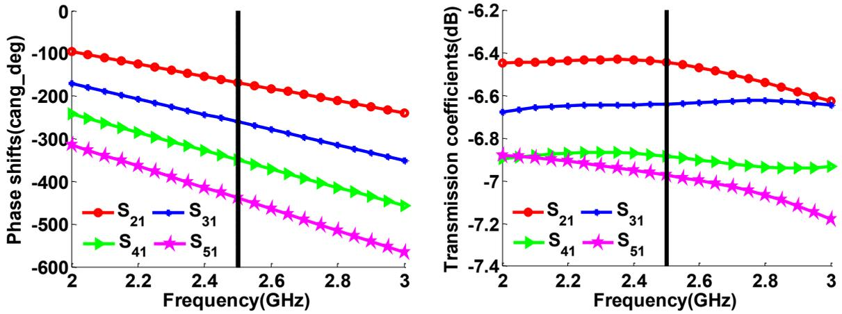
Figure II-13: Simulated parameters of the phase shifter-power divider: phase shifts (left) and transmission coefficients (right). At 2.5 GHz, the phase shifts of  $S_{21}$ ,  $S_{31}$ ,  $S_{41}$ ,  $S_{51}$  are  $-168^\circ$ ,  $-261^\circ$ ,  $-350^\circ$ ,  $-439^\circ$ , respectively; and the corresponding amplitudes are  $-6.4$  dB,  $-6.6$  dB,  $-6.9$  dB,  $-7$  dB.
