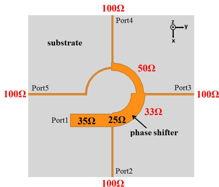
Figure II-12: Geometry of the phase shifter-power divider
