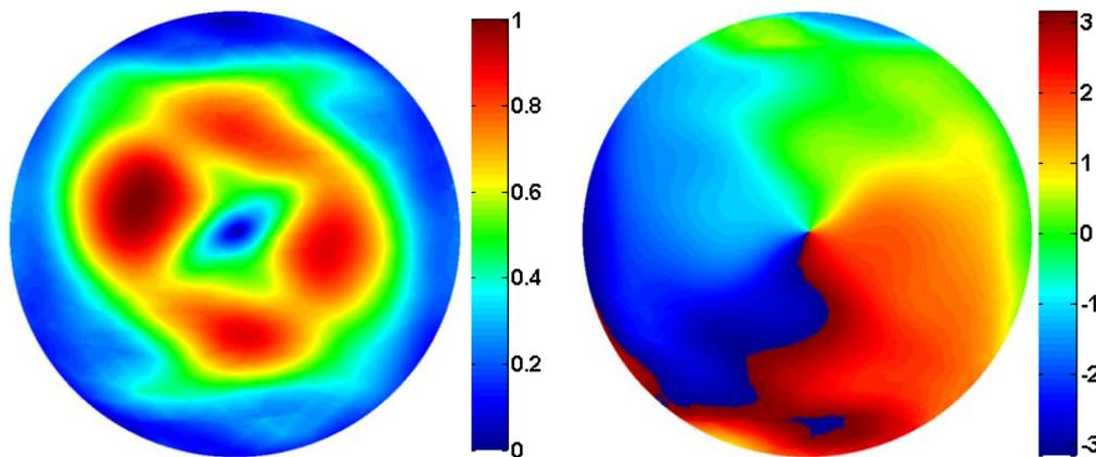
Figure III-19: Normalized magnitude (left) and phase (right) patterns of  $E_x$  component for the FP OAM antenna at 2.5 GHz (circular observation window with a radius of 300 mm, lying 30 mm above the PRS)
