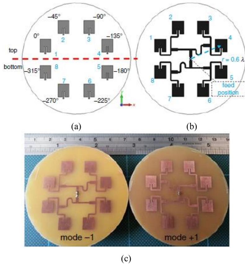
Figure I-25: Geometry of OAM circular phased array: (a) ideal model; (b) practical design; (c) prototypes [29]
