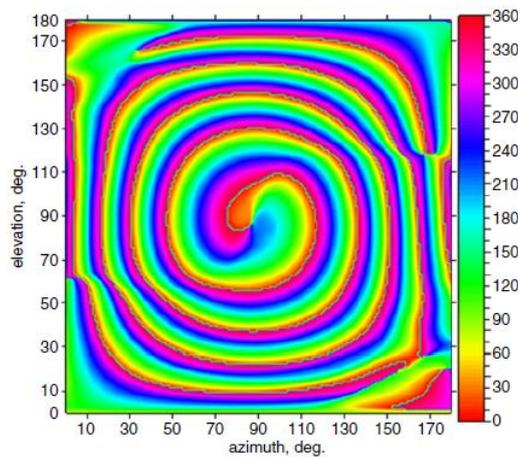
Figure I-26: Measured far-field phase pattern with an OAM mode of  $l = 1$ [29]
