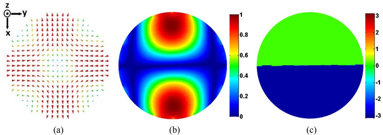
Figure IV-26: Field distribution of the 2<sup>nd</sup> kind of  $TE_{21}$  mode and the corresponding magnitude and phase patterns of  $E_x$  component: (a) Field distribution; (b) Normalized magnitude pattern; (c) Phase pattern.
