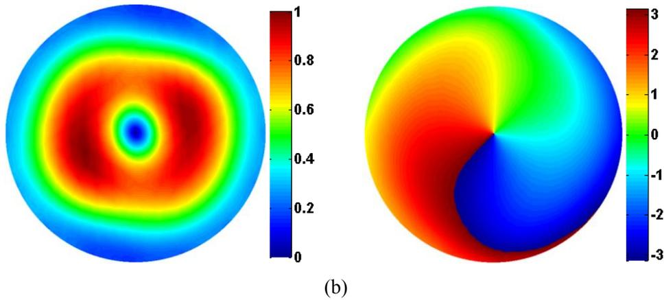
Figure IV-32: Magnitude (left) and phase (right) patterns of the propagated wave: (a)  $E_x$  component; (b)  $E_y$  component (observation window: circular area with a radius of 3 cm, lying 1 cm above the waveguide aperture)
