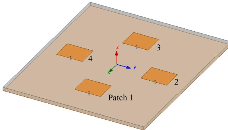
Figure II-4: 3D model of a 4-patch-antenna array
