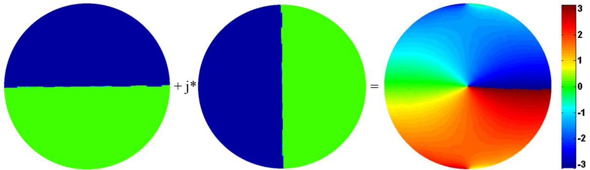
Figure IV-28: Evolutions of magnitude (top) and phase (bottom) patterns of  $E_y$  component for the generation of an OAM wave, by combining two kinds of  $TE_{21}$  modes with a  $\pi/2$  phase difference
