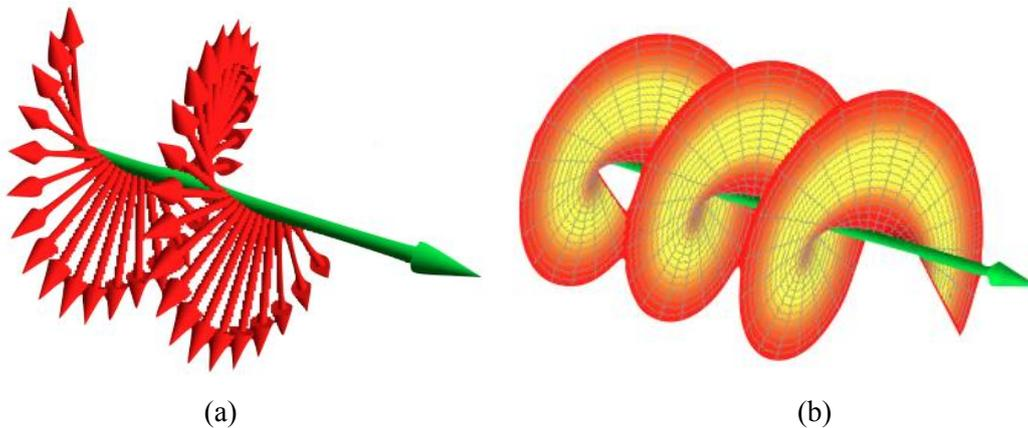
Figure I-1: (a) The SAM of an EM wave; (b) the OAM of an EM wave [33]
