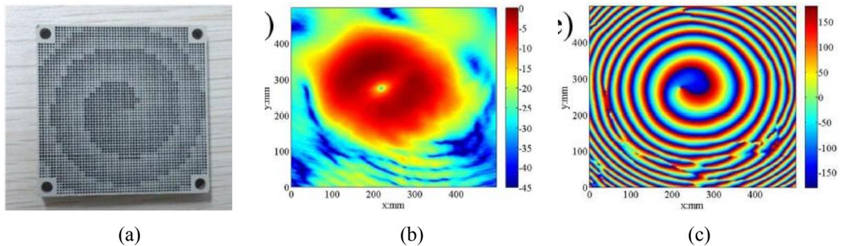
Figure I-18: (a) View of a single mode OAM antenna; (b) Measured transverse magnitude pattern; (c) Measured transverse phase pattern [53]
