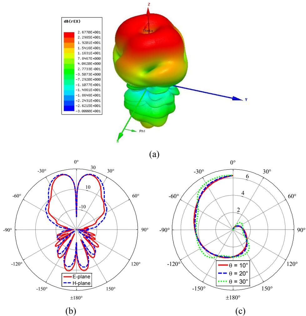
Figure IV-18: Radiation and phase patterns of the OAM horn antenna with two half-turn SPPs at the frequency of 7.4 GHz (based on  $TM_{01}$  mode): (a) 3D radiation pattern; (b) 2D radiation patterns in E and H planes; (c) Normalized phase patterns (in radians) at different  $\theta$  angles
