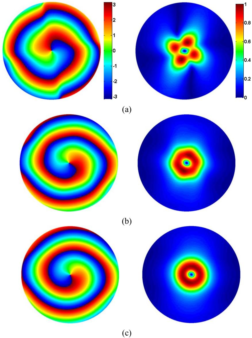
Figure II-7: 2D phase (left) and magnitude (right) patterns of  $E_x$  component for OAM mode  $\ell = 1$  with different numbers of array elements at 2.5 GHz: (a)  $N = 4$ ; (b)  $N = 6$ ; (c)  $N = 8$ .
