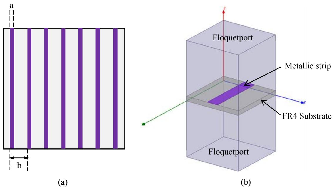
Figure III-4: (a) Geometry of the PRS made of metallic strips; (b) a unit cell of the PRS
