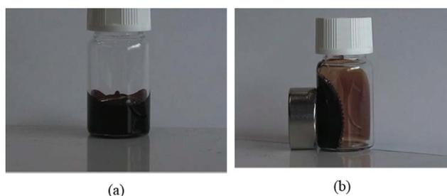
**Fig. 7.** Behavior of the ferrofluid in absence (a) and presence (b) of a magnetic field.<sup>31</sup>
