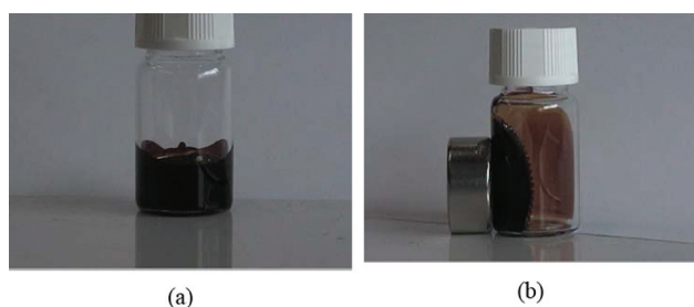
Fig. 7. Behavior of the ferrofluid in absence (a) and presence (b) of a magnetic field. 31
