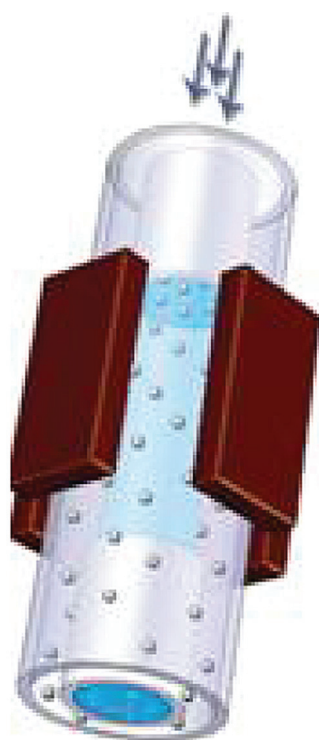
Fig. 18. Magnetic Quadrupole separator as “microfluidic” because of functionality of laminar flow [86].
