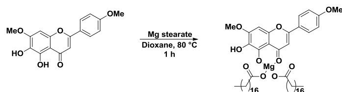
Scheme 2. Synthesis of FOMe.MgStearate complex from ladanein and MgStearate.
