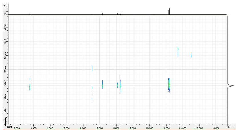
Figure 17. DOSY ^1\text{H} NMR spectrum of the flavone FOMe in \text{DMSO-}d_6 . T = 298\text{ K} . Frequency = 600 MHz.
