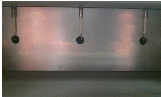
Figure 3.11: Photograph of the three hot wires mounted in the near vicinity of the injection plate.
