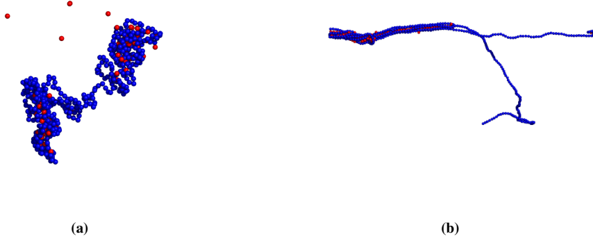
Figure 2.9 – Two equilibrium configurations of a polymer chain (blue) interacting with binding spheres (red) in the absence of bending rigidity ( l_p = 0 ) and with strong bending rigidity ( l_p = 30 ), obtained with BD simulations. We used a truncated Lennard-Jones potential with \varepsilon = 3.0k_B T and r^{th} = 2 . In both cases, the system is phase separated. (a) For l_p = 0 , the dense phase consists of several globular aggregates distributed in a necklace fashion along the chain. (b) For l_p = 30 , the dense phase adopts a tubular structure.
