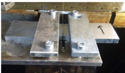
Fig. 16 Part clamping during wire electro-discharging machine cutting
