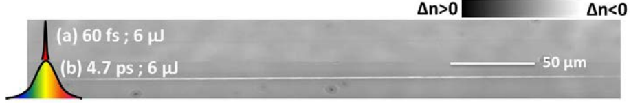
Figure 4.3: Selected phase contrast microscopy images of the structural modifications using single shot ultrafast Bessel beam under moderate focusing conditions (conical half-angle of the Bessel in the medium \sim 8.3^\circ ). (a) Smooth refractive index structure at 60 fs and 6 \mu\text{J} /pulse. (b) Uniform void structure at 4.7 ps and 6 \mu\text{J} /pulse
