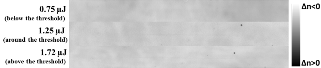
Figure 6.1: Single pulse static phase contrast images of the smooth refractive index structure are shown around the modification threshold. The structures at 0.75 \mu\text{J} , 1.25 \mu\text{J} and 1.72 \mu\text{J} are corresponding to the below, around and above the modification threshold respectively.
