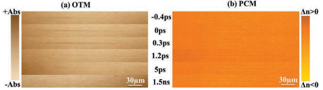
Figure 6.2: Transient optical transmission and phase contrast images in conditions corresponding to formation of smooth refractive index structure are shown in (a) and (b) respectively at various probe delays around the damage threshold at laser pulse energy of 1.25 \mu\text{J} and pulse duration of 60 fs.
