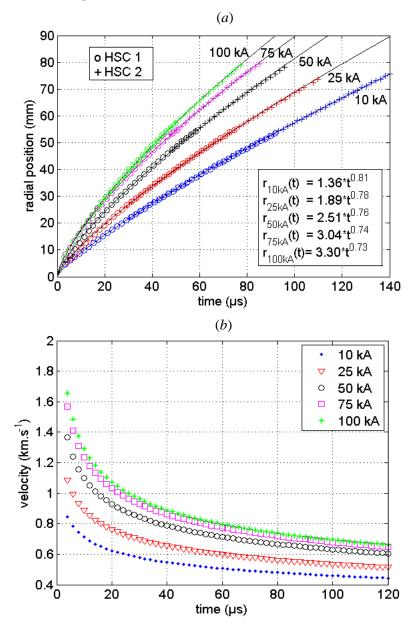
*Figure III.11. (a) Shock wave position measured by the HSC 1 at 2 m and the HSC 2 at 3 m from the arc column and (b) the shock wave velocity.*
