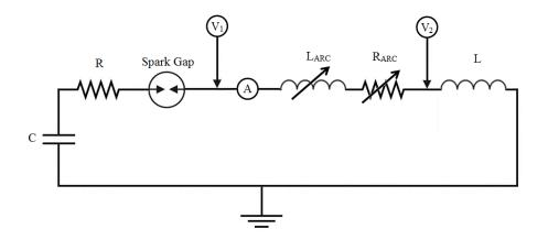
Figure IV.1. Equivalent electric circuit of the lightning current generator with variable components  $L_{ARC}$  and  $R_{ARC}$  and the probes  $V_1$  and  $V_2$  for voltage measurements and A for current measurements.
