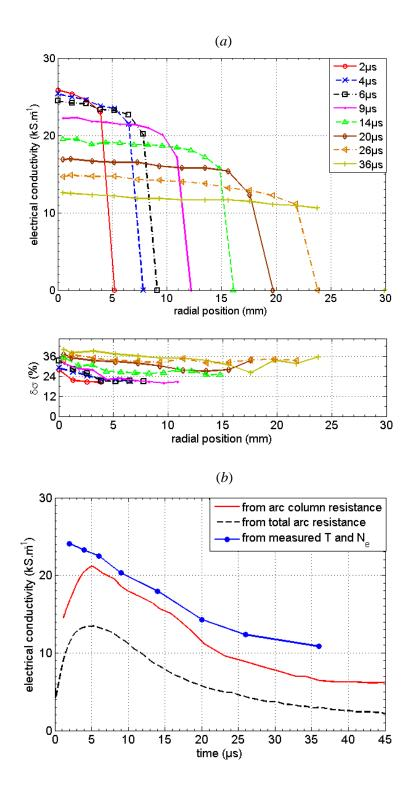
Figure V.17. (a) Electrical conductivity profile for the 100 kA current peak level.
