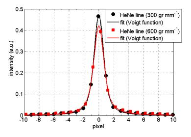
*Figure II.9. Measured HeNe line (632.816 nm) used for slit function determination. For the gratings of 300 grooves mm*<sup>-1</sup> and 600 grooves mm<sup>-1</sup>, one pixel corresponds to 0.104 nm and 0.05 nm, respectively.
