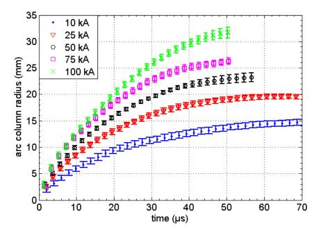
Figure III.6. Luminous arc radius for different current peaks.
