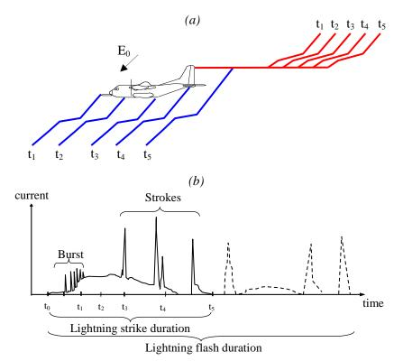
Figure I.7. Illustration of the swept stroke process. (a) The swept represented in the frame of reference of the aircraft for different times t<sub>i</sub>. (Chemartin (2008)). (b) Typical current waveform obtained by in-flight measurements (Lalande et al. (1999)).
