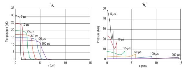
Figure I.16. Temperature (a) and pressure (b) profiles resulting from the MHD code developed by Peyrou (2012). The input is a D-component with current peak of 100 kA and peak time of 6.4 μs.
