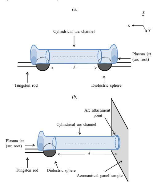
Figure II.2. Electrodes configuration. (a) diverter-diverter. (b) diverter-panel.
