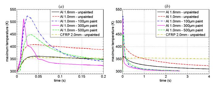
Figure VI.20. Maximum temperature in the rear face of the different panels. Detail in the first 200 ms (a) and the evolution during 4 s (b).
