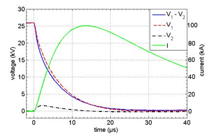
*Figure IV.2. Example of voltage measurements by probes V*<sub>1</sub> and V<sub>2</sub> and current measurements I by the probe A for the 100 kA peak.
