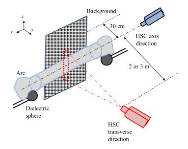
*Figure II.6. Schematic diagram of the BOS setup and the two directions utilized to characterize the shock wave.*
