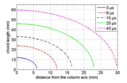
Figure V.3. Example of chord lengths that cross the column as a function of the distance from the column axis, calculated for 100 kA peak.
