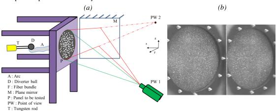
*Figure II.13.* (a) Setup for Stereo-DIC measurement. (b) Example of two points of view taken using only one HSC and a plane mirror (resolution: 800 × 500 pixels; scale: 0.75 mm/pixel).
