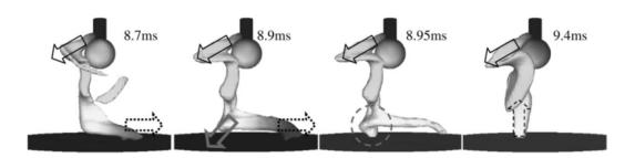
Figure I.15. Simulation of an unsteady continuous arc (400 A) using the MHD approach, considering the electrode effects and the arc reattachment process. The grey region represents an isotherm surface at 8000 K (Chemartin et al. (2011)).
