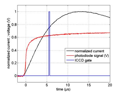
Figure II.11. Synchronization between the current waveform and the spectra acquisition. In this example, the gate is opened 6 µs after the current initiation and has a width of 200 ns.
