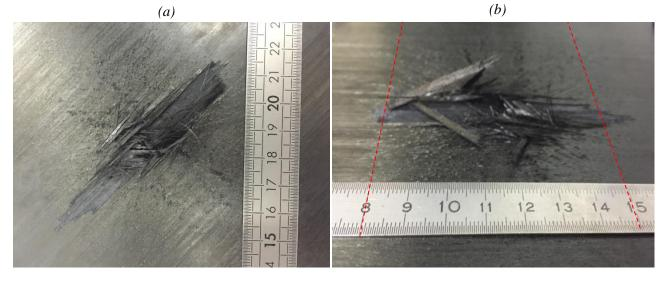
Figure VI.18. Damage in CFRP panel after the direct lightning arc test.
