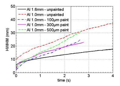
*Figure VI.22. Half width at half maximum (HWHM) for the temperature profile in the panel surface.*
