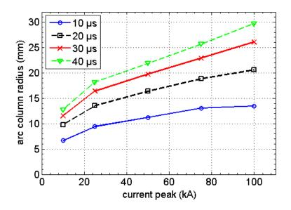
Figure III.7. Arc column radius versus the current peak for different times.
