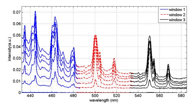
Figure V.9. Example of the overlapping of the collected spectra from the three spectral windows after relative intensity calibration. Experimental parameters: peak of current = 100 kA; time = 14 µs; chord positions from the central arc: 11 mm, 8.3 mm, 5.7 mm, 4.4 mm, 3.1 mm 1.8 mm; exposure time = 200 ns.
