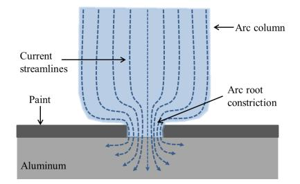
Figure VI.7. Illustration of the current streamlines constriction in paint aluminum panels.
