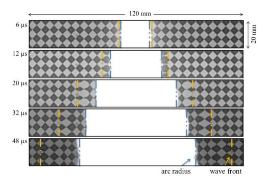
*Figure II.7. Pictures of the luminous central arc region and shock wave evolution for the 100 kA peak.*
