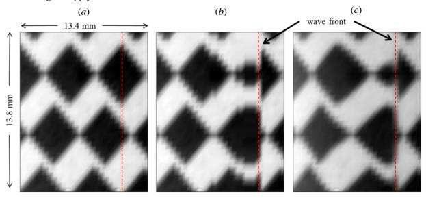
Figure III.13. Example of image reconstruction from a mass density profile. (a) Reference image; (b) Simulated image; (c) Measured image.
