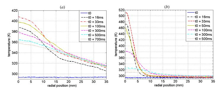
Figure VI.21. Radial profiles of temperature of aluminum panels with 1 mm thickness. (a) Unpainted panel. (b) 100 µm painted panel.
