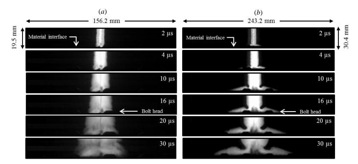
Figure VI.9. Pictures of the arc root evolution over time applied to a carbon fiber composite panel. (a) Camera axis perpendicular to the surface ply orientation (resolution: 256 × 32 pixels; scale: 0.61 mm/pixel; exposure time: 0.3 μs).
