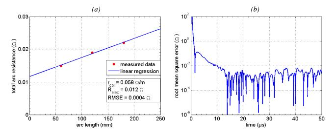
Figure IV.8. Example of (a) linear regression for the 100 kA peak at 15 µs and (b) the root mean square error (RMSE).
