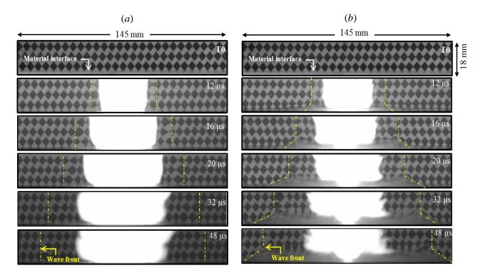
*Figure VI.12. Pictures of the shock wave propagation for the case of (a) unpainted and (b) painted aluminum panels.*
