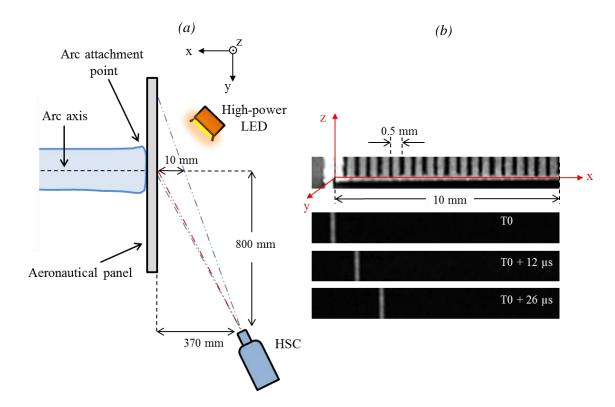
Figure II.15. (a) Top-view of the diagnostic setup for fast direct deflection measurements.
