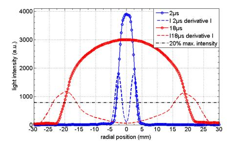
Figure III.4. Criteria for luminous radius determination. Experimental parameters resolution: 256 × 32 pixels; scale: 0.29 mm/pixel; exposure time: 300 ns; saturation: 4095 a.u..
