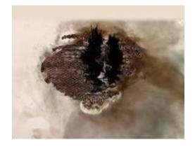
Figure I.11. Damage of carbon fibers tows at the lightning attachment point (Source: National Institute for Aviation Research (NIAR))
