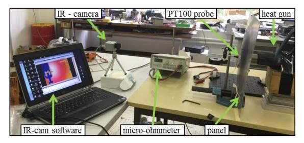
Figure VI.1. Diagnostic setup for infrared thermography measurement calibration.
