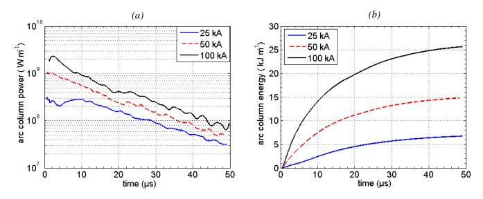
Figure IV.11. Power (a) and accumulated energy (b) dissipated per length inside the arc column by Joule effect.
