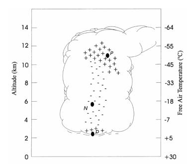
*Figure I.1. Generalized diagram showing distribution of electrical charge in a typical cumulonimbus cloud (ARP5412A (2005)). 'P' indicates the positive charge regions and 'N' indicates the negative ones.*
