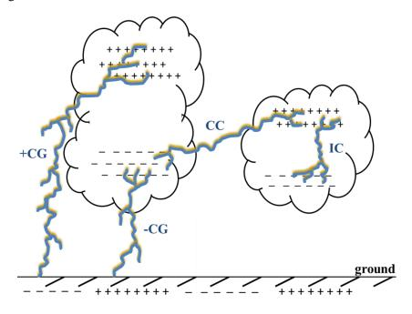
Figure I.4. Illustration of four types of lightning flashes.
