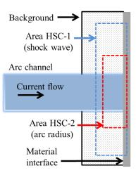
*Figure VI.2. Side view of the arc attachment point. Area of collection for the two high speed cameras (HSC).*
