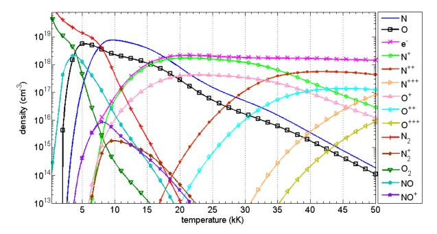
Figure V.5. Population densities of LTE air plasma composition calculation at 15 bar (Argon not shown).
