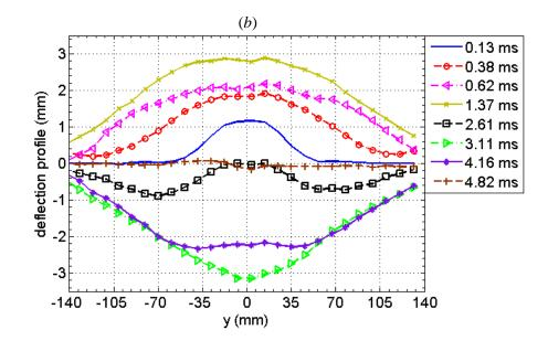
Figure VI.24. Example of deflection profile along y-axis. (a) 1.0 mm aluminum panel with 100 µm paint. (b) 2.0 mm CFRP panel.
