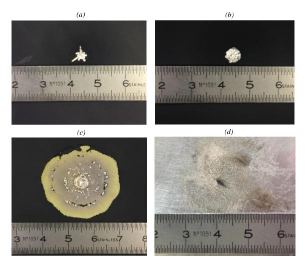
Figure VI.16. Some pictures of the damage in the aluminum panels after the direct lightning arc test. (a) 100 μm. (b) 300 μm. (c) 500 μm. (d) unpainted.
