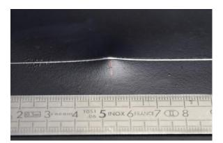
Figure VI.17. View of the rear face of the panel, highlighting the plastic deformation for the 1 mm aluminum 100 µm paint, after the application of a 100 kA current waveform.
