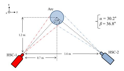
Figure III.2. Schematic diagram for different azimuthal position collection.
