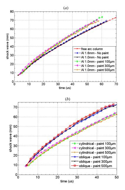
Figure VI.14. Shock wave position for different paint thicknesses. (a) Comparison of the cylindrical shock wave for all aluminum panels and the free arc column.
