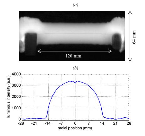
Figure II.5. (a) Picture of the arc in the diverter-diverter configuration for a 100 kA peak waveform at 14 µs after ignition (resolution: 256 × 96 pixels; scale: 0.67 mm/pixel; exposure time: 300 ns).
