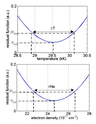
*Figure V.8. Examples of variation of the residual fit (equation (V.7)) as a function of two parameters and the criterion for the error bar estimations.*
