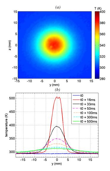
Figure II.12. (a) Surface temperature in the rear face of an aluminum panel of 1 mm thickness with paint of 100  $\mu$ m at 33 ms after the trigger. (b) Temperature profiles for z = 0 at different times (scale: 0.31 mm/pixel; current peak: 100 kA).
