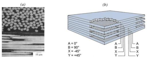
*Figure I.10. (a) Laminated composite magnification picture highlighting the carbon fibers of a tow. (b) Layup of plies with different fiber orientations (Chawla (2012)).*
