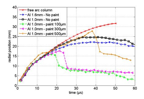
Figure VI.6. Evolution of the visible arc root radius for aluminum panels and the radius of a free arc column.
