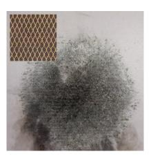
Figure I.12. After test result for a carbon composite sample with copper mesh protection (Source: Morgan-Botti Lightning Laboratory)
