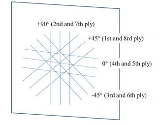
Figure VI.1. Example of a unit cell structure in a multi-layup CFRP panel.
