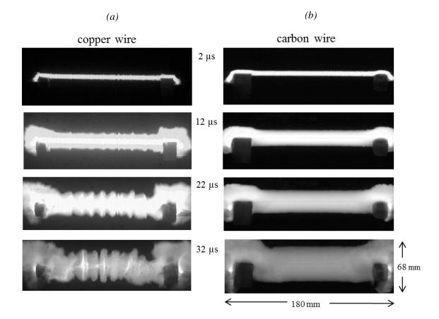
Figure III.1. Comparisons of the development of the arc column using two different ignition wire. (a) Copper wire. (b) Carbon wire. Experimental parameters resolution: 256 × 96 pixels; scale: 0.70 mm/pixel; exposure time: 300 ns; current peak: 100 kA.
