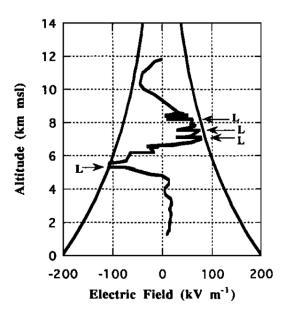
Figure I.2. Thundercloud electric field and breakeven field as a function of altitude. Each "L" marks a horizontal discontinuity in electric field produced by a lightning flash occurrence (Marshall et al. (1995)).
