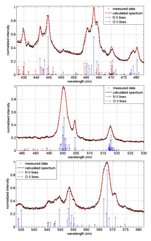
Figure V.10. Examples of measured and calculated spectra for the three spectral windows. Experimental parameters: peak of current = 100 kA; time = 6  $\mu$ s; chord position from the central arc = 3.6 mm; exposure time = 200 ns.
