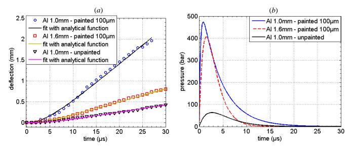
Figure VI.27. (a) Measured and calculated deflection, using the analytical function derived from a bi-exponential pressure (equation (VI.10)). (b) Pressure obtained from the three fit parameters.
