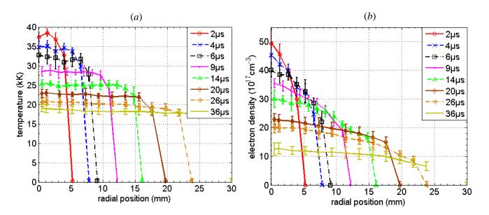
Figure V.12. Average radial distributions of temperature and electron density calculated from the profiles of the three spectral windows for the 100 kA peak current; error bars indicate here the dispersion of the three results.
