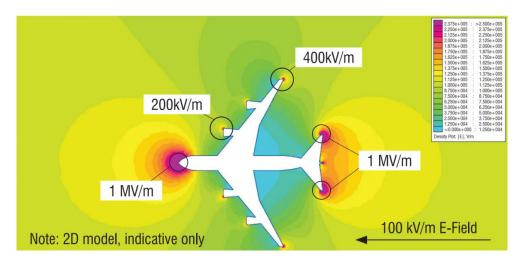
*Figure I.5.* Indicative 2D electrostatic model of an aircraft in a 100 kV m<sup>-1</sup> ambient field calculated by Morgan et al. (2012).
