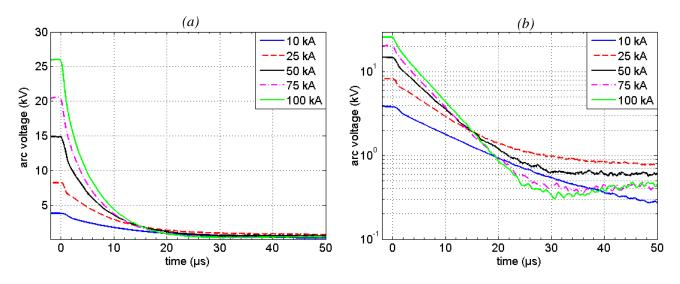
Figure IV.3. (a) Arc voltage for the five levels of current peak. (b) Arc voltage in semi-logarithmic scale.
