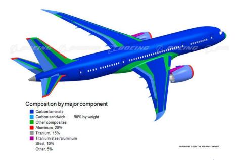
Figure I.9. Boeing 787 Dreamliner material composition (Source: <sup>©</sup>Boeing).
