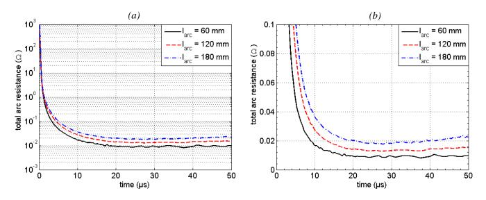
Figure IV.7. (a) Example of total arc resistance for three arc lengths, for the case of 100 kA peak. (b) Plot in linear scale to highlight the linearity of the arc resistance as a function of the arc length.
