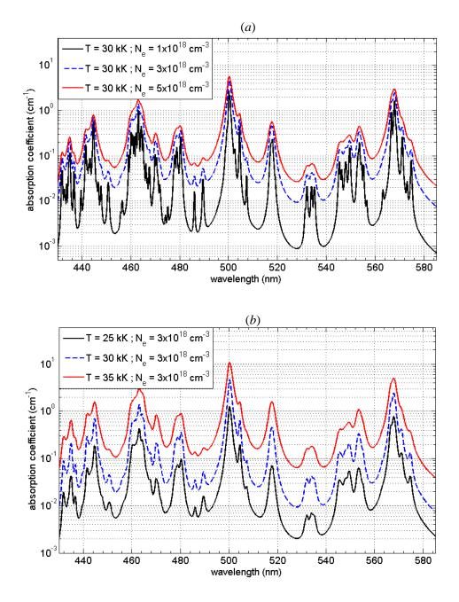
Figure V.6. Absorption coefficient calculated from equation (V.1) for different values of T and  $N_e$ . (a) Variation with electron density. (b) Variation with temperature.
