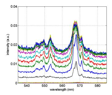
Figure II.10. Example of spectra collected by the diagnostic setup at different position inside the channel arc. Experimental parameters: current peak = 100 kA; time = 9  $\mu$ s; exposure time = 200 ns.
