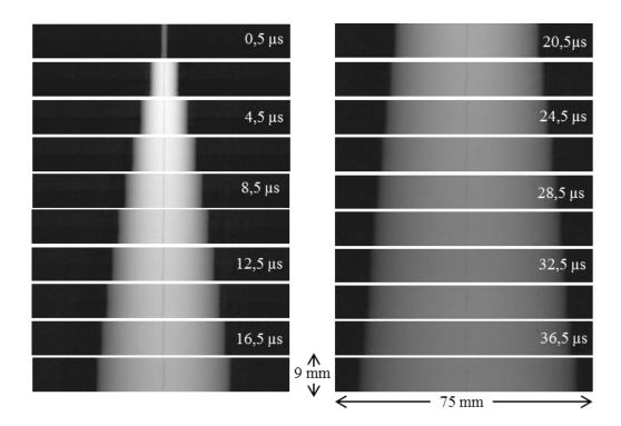
Figure III.5. Pictures of the column expansion during the first 38.5 µs. Experimental parameters – current peak: 100 kA; resolution: 256 × 32 pixels; scale: 0.29 mm/pixel; exposure time: 300 ns.
