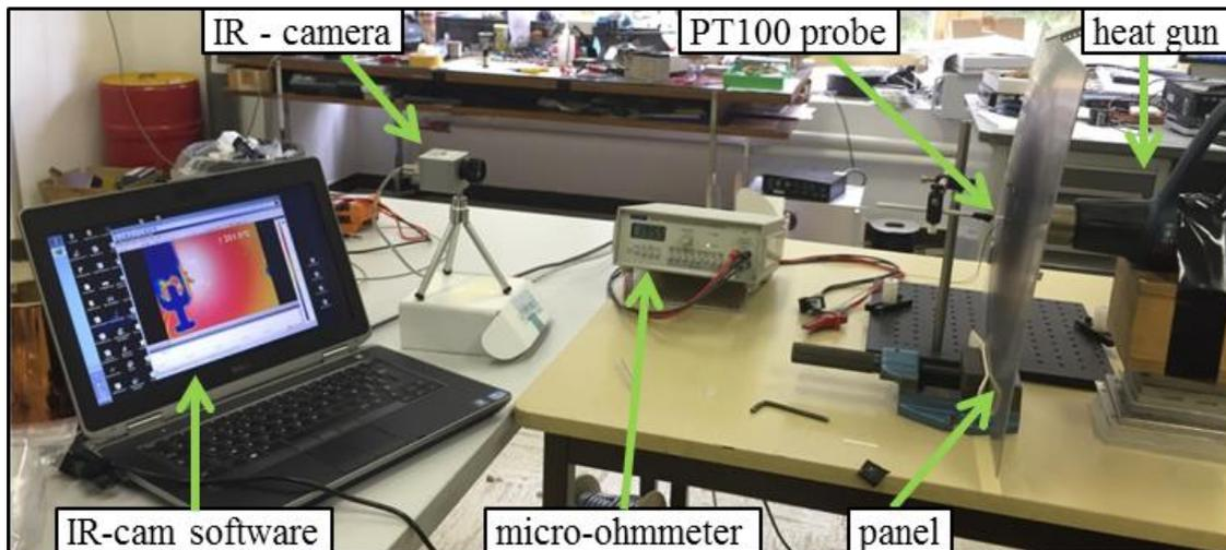
Figure VI.1. Diagnostic setup for infrared thermography measurement calibration.
