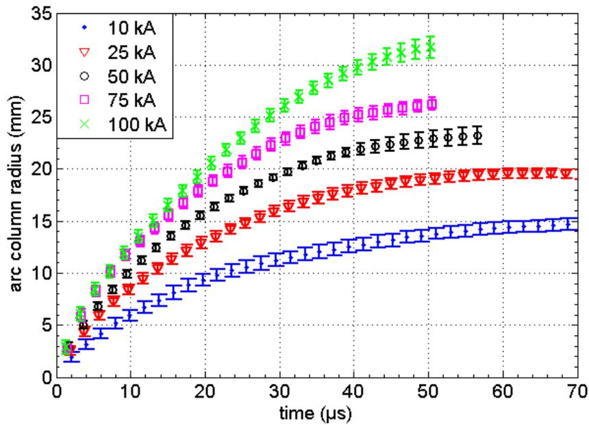
Figure III.6. Luminous arc radius for different current peaks.
