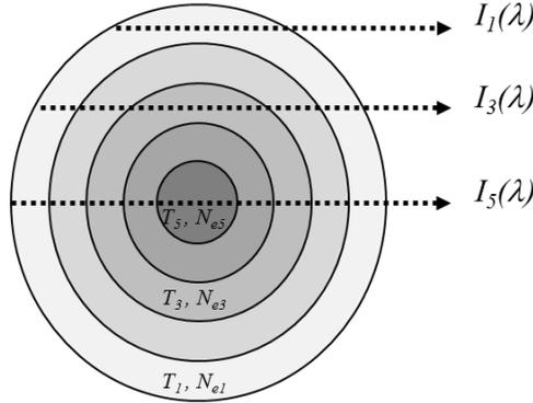
Figure V.7. Schematic for the chords that cross the arc channel in discretized homogeneous layers. Each layer  $i$  has a constant temperature  $T_i$  and electron density  $N_{ei}$ .
