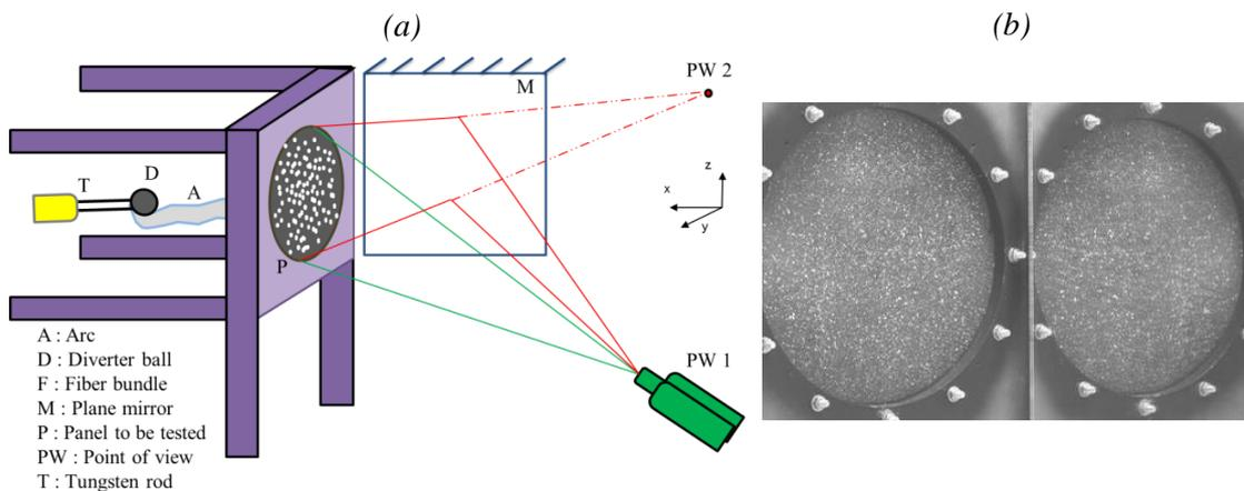
Figure II.13. (a) Setup for Stereo-DIC measurement. (b) Example of two points of view taken using only one HSC and a plane mirror (resolution:  $800 \times 500$  pixels; scale:  $0.75$  mm/pixel).
