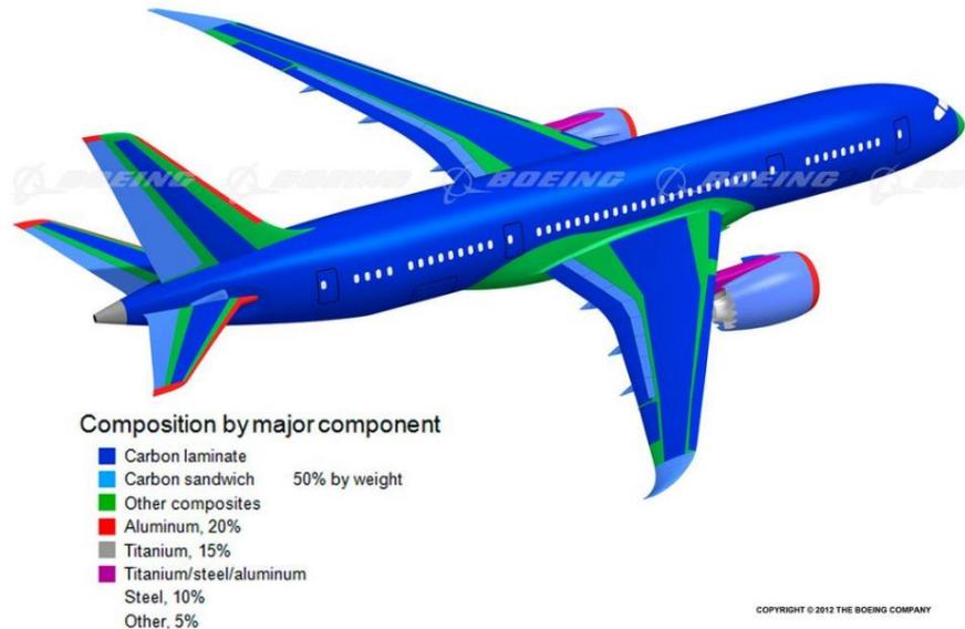
Figure I.9. Boeing 787 Dreamliner material composition (Source: ©Boeing).
