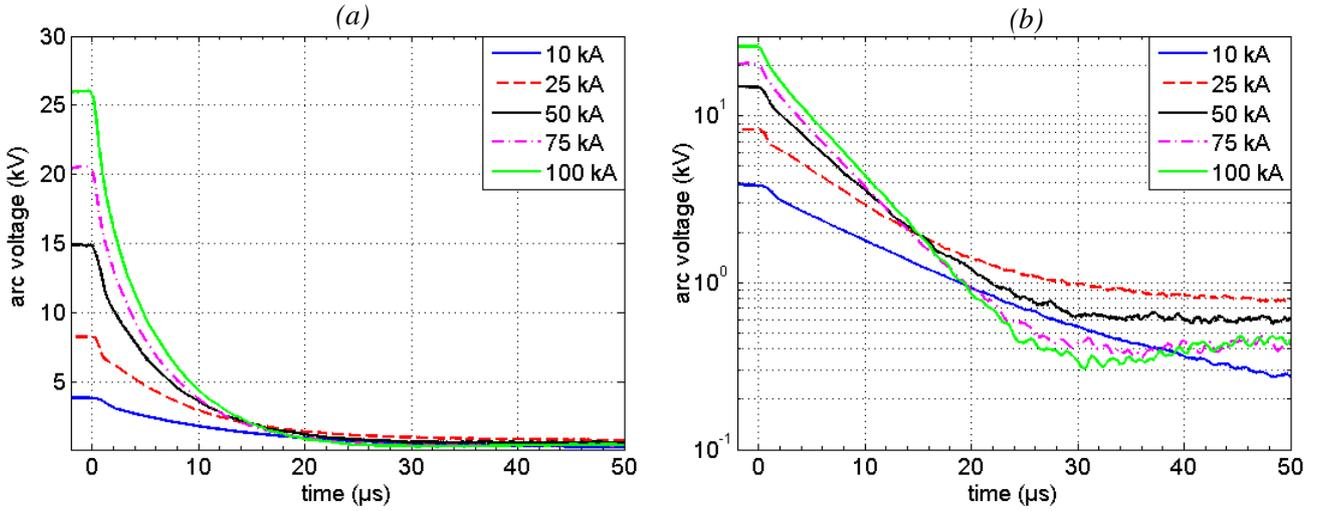
Figure IV.3. (a) Arc voltage for the five levels of current peak.
