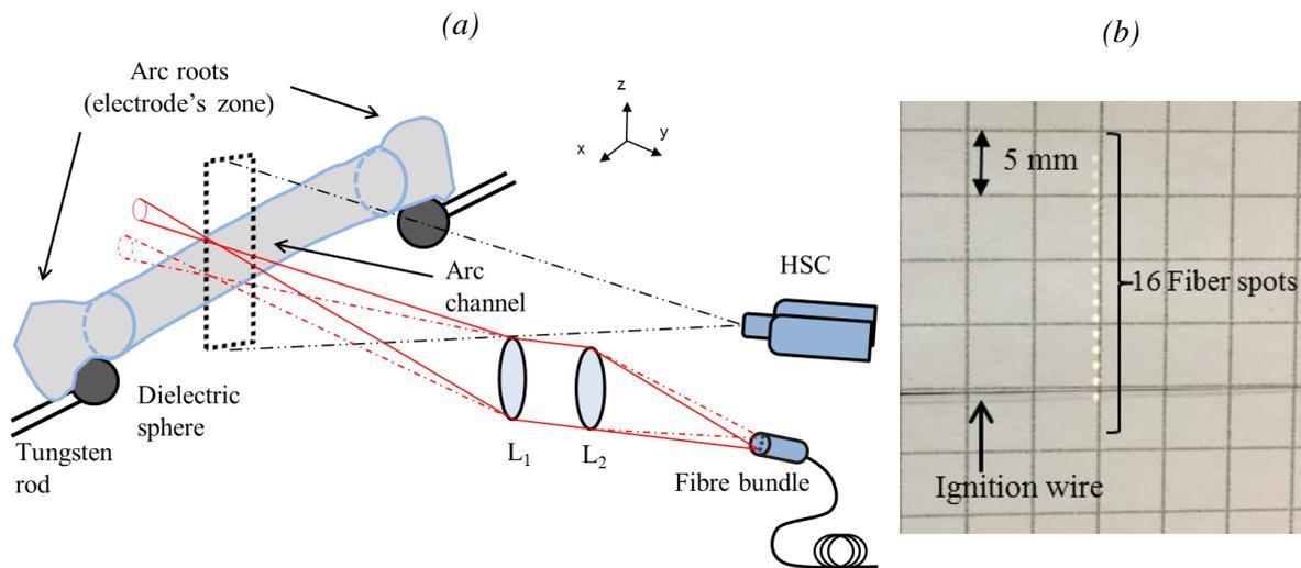
Figure II.8. (a) Optical system for OES measurements. (b) Fiber spots collected by the optical system for an asymmetrical bundle configuration.
