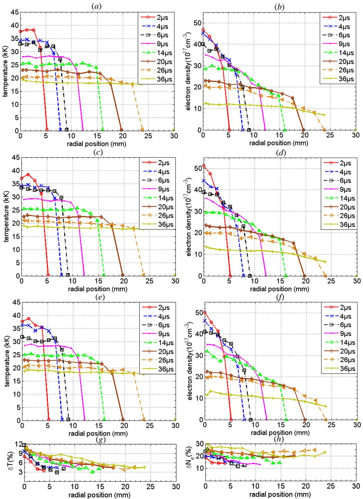
Figure V.11. Temperature and electron density profiles for the 100 kA current peak from the three spectral windows; (a-b) 431.5 nm to 485 nm; (c-d) 481.5 nm to 535 nm; (e-f) 531.5 nm to 585 nm; (g-h) maximum percentage uncertainty according to the criterion of section V.1.5.
