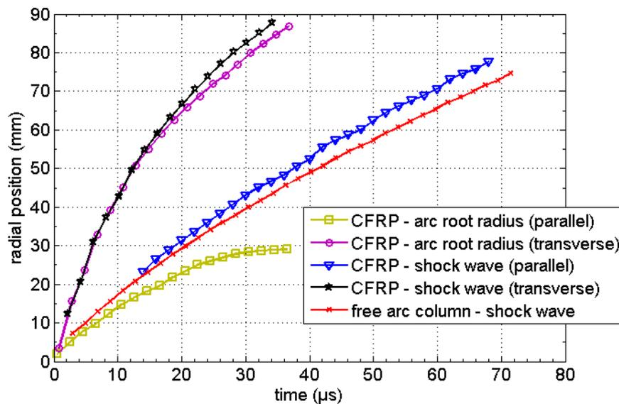
Figure VI.15. Shock wave position and arc root radius for the CFRP panel in the parallel and transverse direction to the surface ply.
