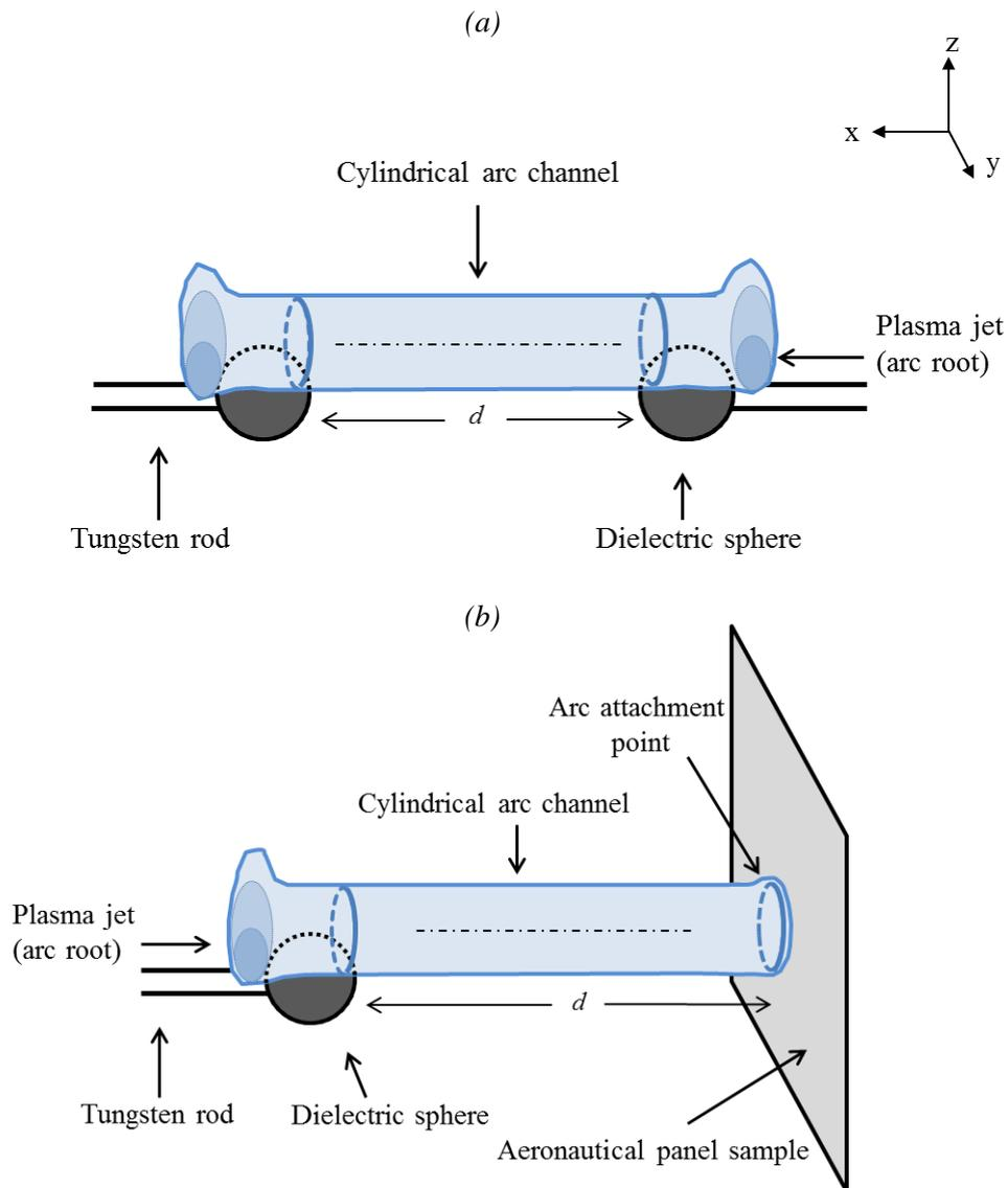
Figure II.2. Electrodes configuration. (a) *diverter-diverter*. (b) *diverter-panel*.
