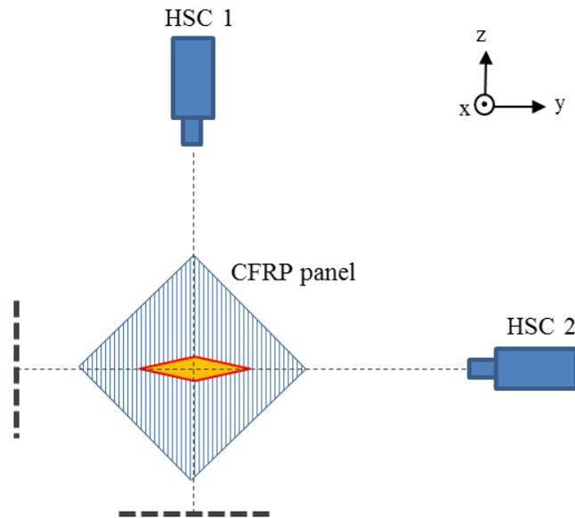
Figure VI.8. Schematic diagram of the different camera positions.
