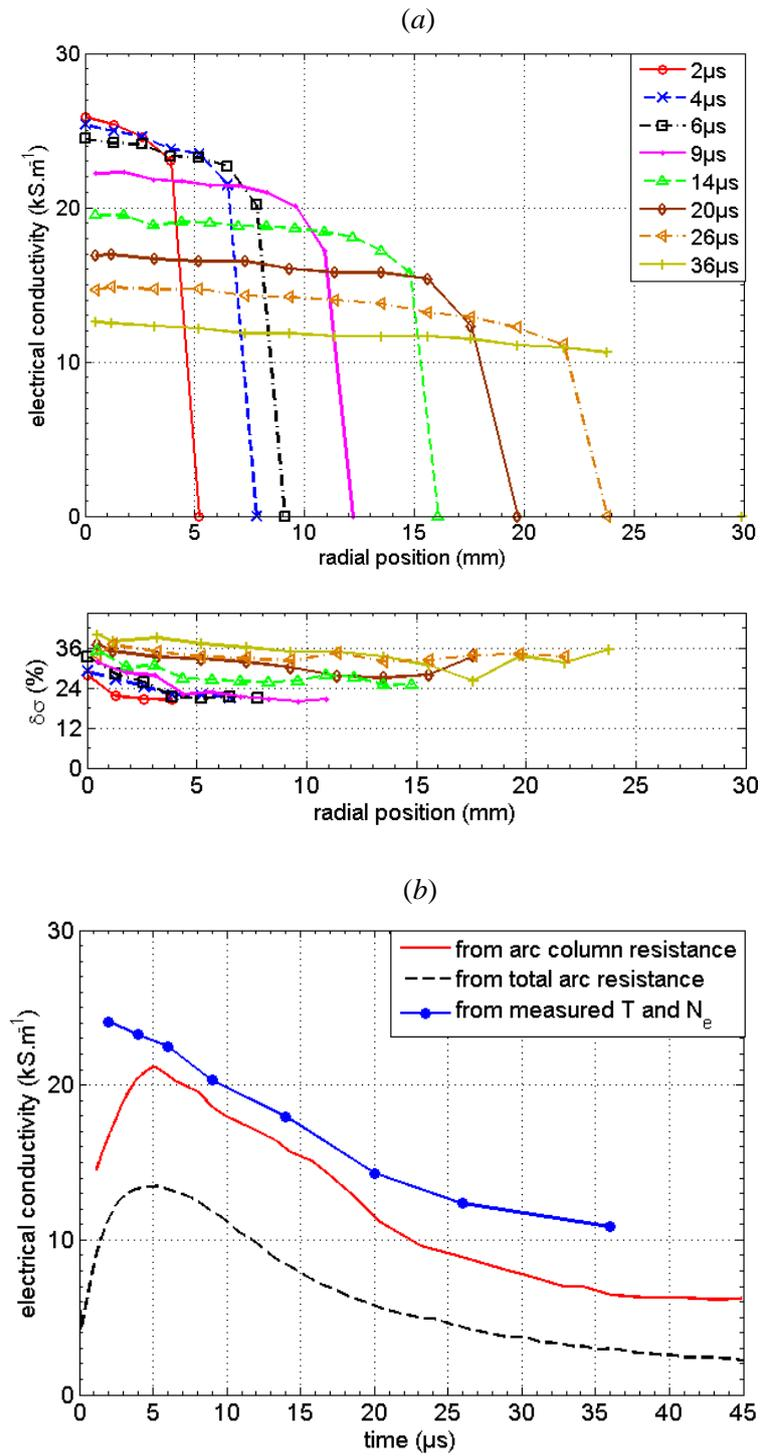
Figure V.17. (a) Electrical conductivity profile for the 100 kA current peak level. (b) Comparison of the radial average values over the cross section estimated from  $T$  and  $P$ , and from electrical measurements.
