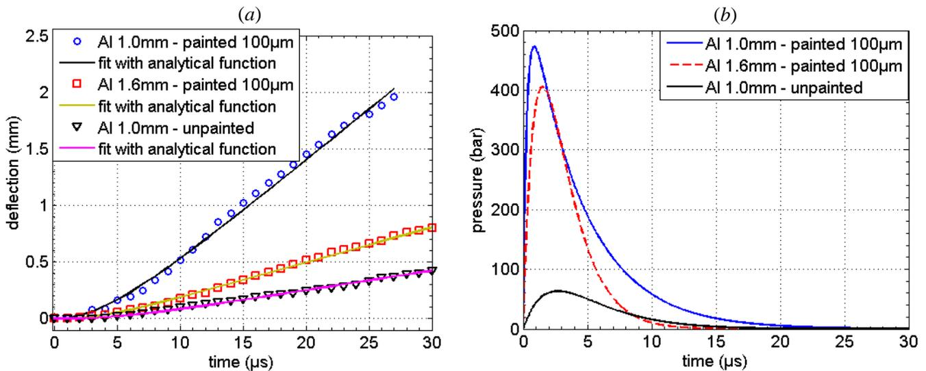
Figure VI.27. (a) Measured and calculated deflection, using the analytical function derived from a bi-exponential pressure (equation (VI.10)).
