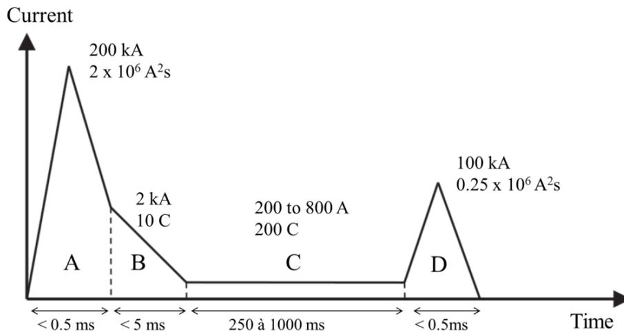
Figure I.13. Standardized lightning current waveforms for lightning direct effect tests (ARP5412A (2005)).
