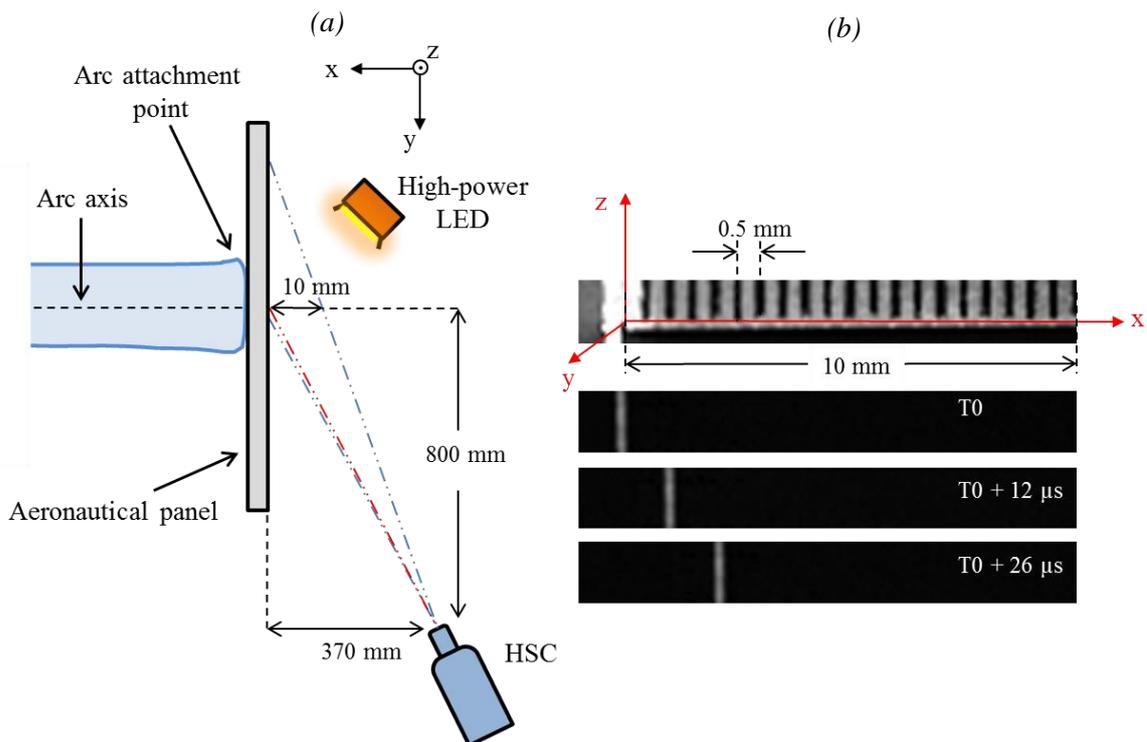
Figure II.15. (a) Top-view of the diagnostic setup for fast direct deflection measurements. (b) Pictures taken using the camera setup of  $128 \times 16$  pixels to the scale settings and an example of deflection measurement for a 100 kA peak current waveform applied to a painted aluminum panel.
