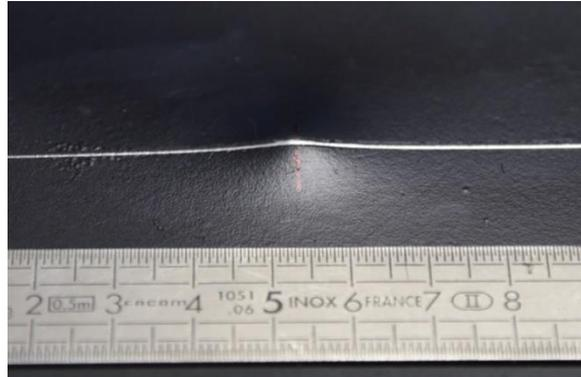
*Figure VI.17. View of the rear face of the panel, highlighting the plastic deformation for the 1 mm aluminum 100  $\mu$ m paint, after the application of a 100 kA current waveform.*
