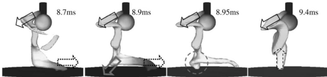
*Figure I.15. Simulation of an unsteady continuous arc (400 A) using the MHD approach, considering the electrode effects and the arc reattachment process. The grey region represents an isotherm surface at 8000 K (Chemartin et al. (2011)).*
