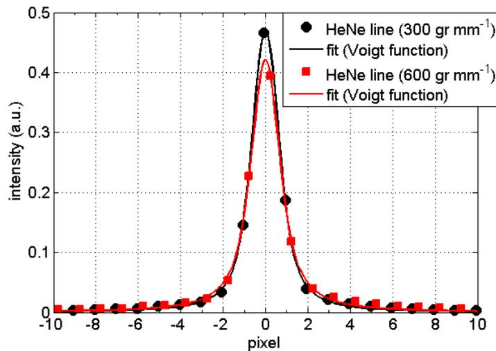
Figure II.9. Measured HeNe line (632.816 nm) used for slit function determination. For the gratings of 300 grooves  $\text{mm}^{-1}$  and 600 grooves  $\text{mm}^{-1}$ , one pixel corresponds to 0.104 nm and 0.05 nm, respectively.
