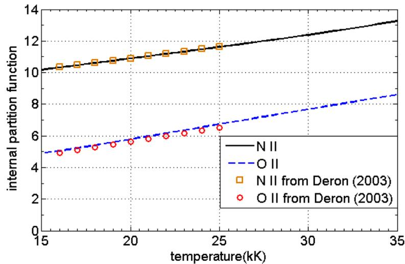
Figure V.4. Comparison of the evolution with temperature of the internal partition functions to the results of *Deron (2003)*.
