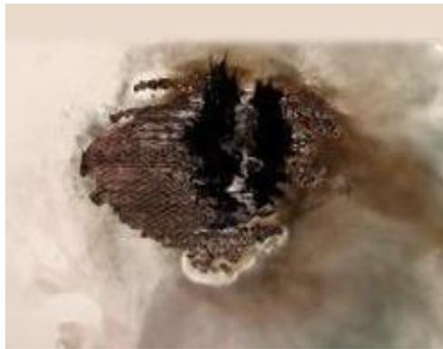
*Figure I.11. Damage of carbon fibers tows at the lightning attachment point
