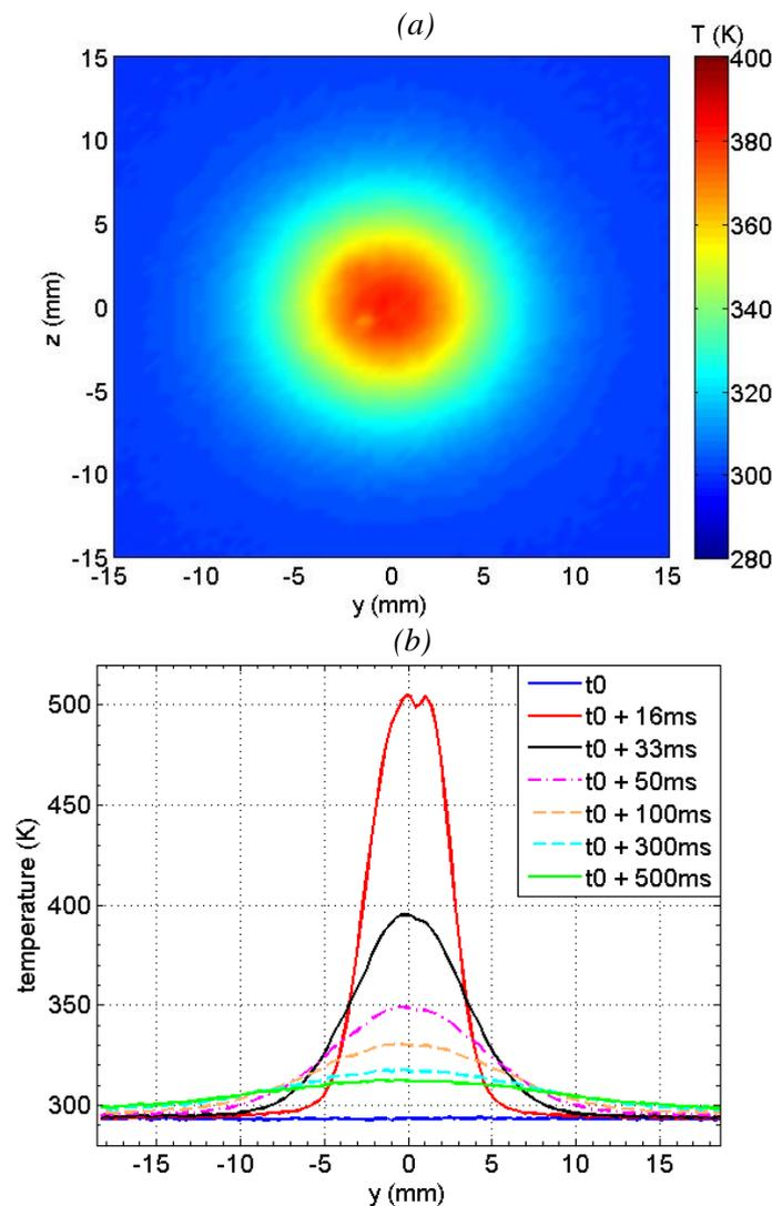
Figure II.12. (a) Surface temperature in the rear face of an aluminum panel of 1 mm thickness with paint of  $100 \mu\text{m}$  at 33 ms after the trigger. (b) Temperature profiles for  $z = 0$  at different times (scale:  $0.31 \text{ mm/pixel}$ ; current peak: 100 kA).
