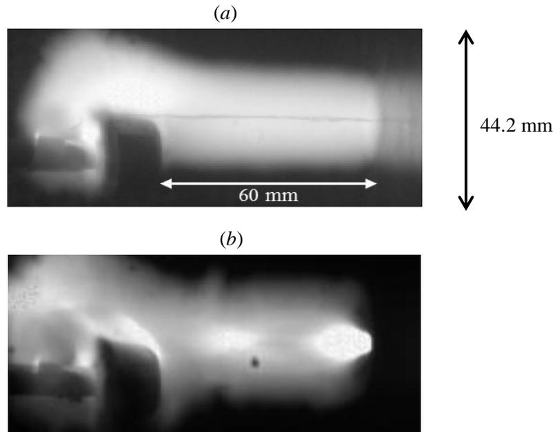
Figure VI.3. Example of arc picture taken at  $15 \mu\text{s}$  after the current triggering for the 100 kA peak waveform applied to unpainted aluminum (a) and painted aluminum (b). The jet diverter electrode is located on the left-hand side and the panel is on the right-hand side (resolution:  $256 \times 96$  pixels; scale:  $0.46 \text{ mm/pixel}$ ; exposure time:  $0.3 \mu\text{s}$ ; frame rate: 200 kfps)
