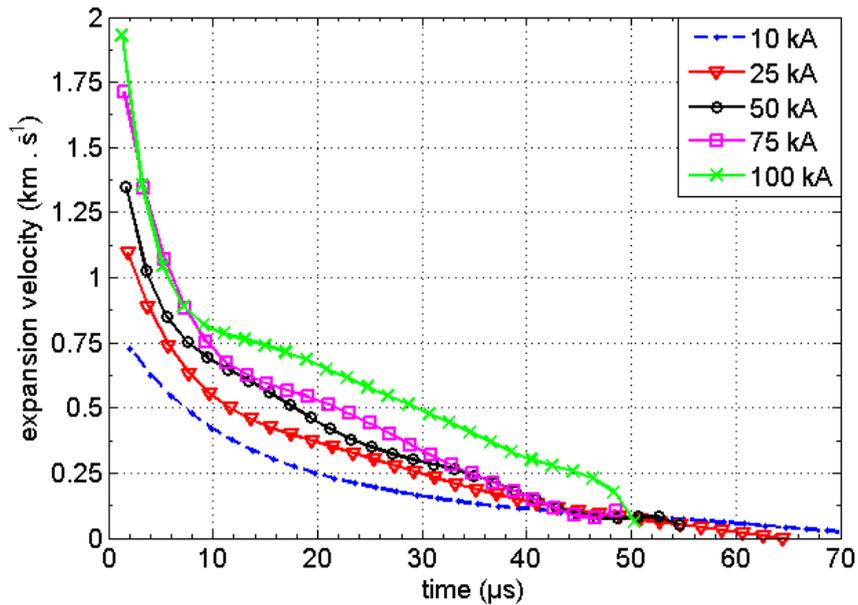
Figure III.8. Expansion velocity for different current peaks.
