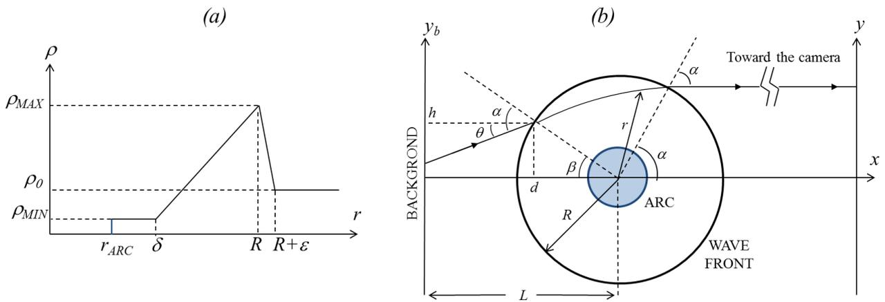
Figure III.12. (a) Schematic mass density profile inside the shock wave.
