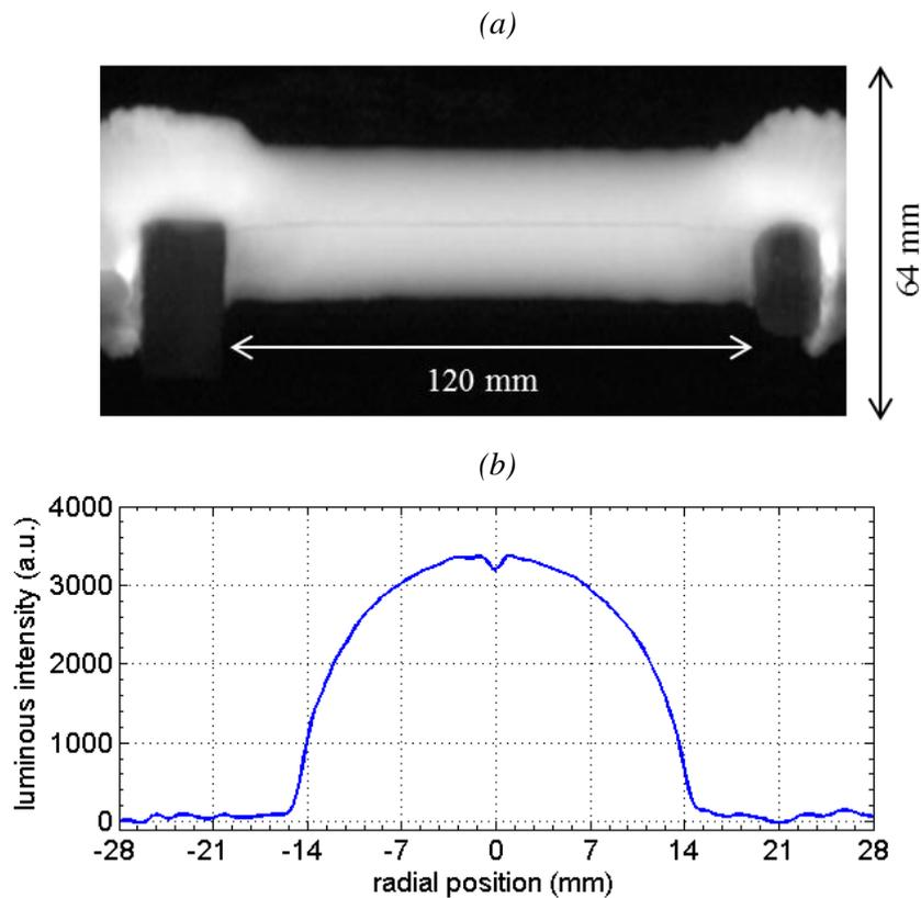
Figure II.5. (a) Picture of the arc in the diverter-diverter configuration for a 100 kA peak waveform at  $14 \mu\text{s}$  after ignition (resolution:  $256 \times 96$  pixels; scale:  $0.67 \text{ mm/pixel}$ ; exposure time: 300 ns). (b) Light intensity distribution along the radial direction at mid-distance between the dielectric spheres (saturation: 4095 a.u.).
