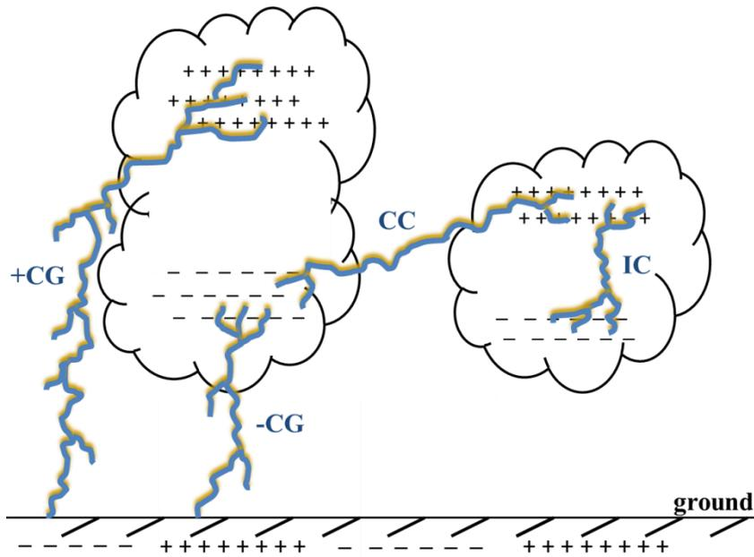
Figure I.4. Illustration of four types of lightning flashes.
