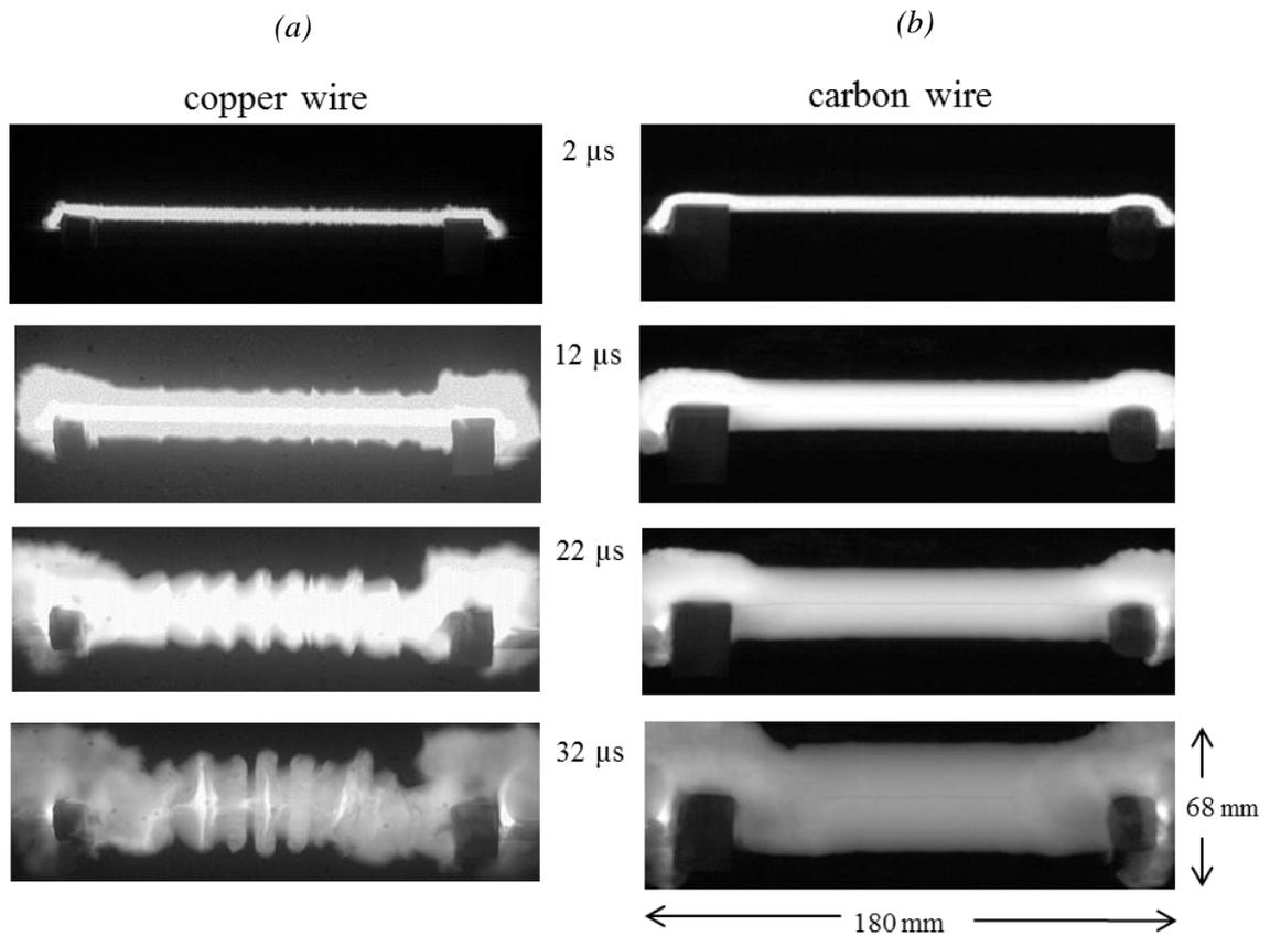
Figure III.1. Comparisons of the development of the arc column using two different ignition wire. (a) Copper wire. (b) Carbon wire. Experimental parameters - resolution:  $256 \times 96$  pixels; scale:  $0.70 \text{ mm/pixel}$ ; exposure time:  $300 \text{ ns}$ ; current peak:  $100 \text{ kA}$ .
