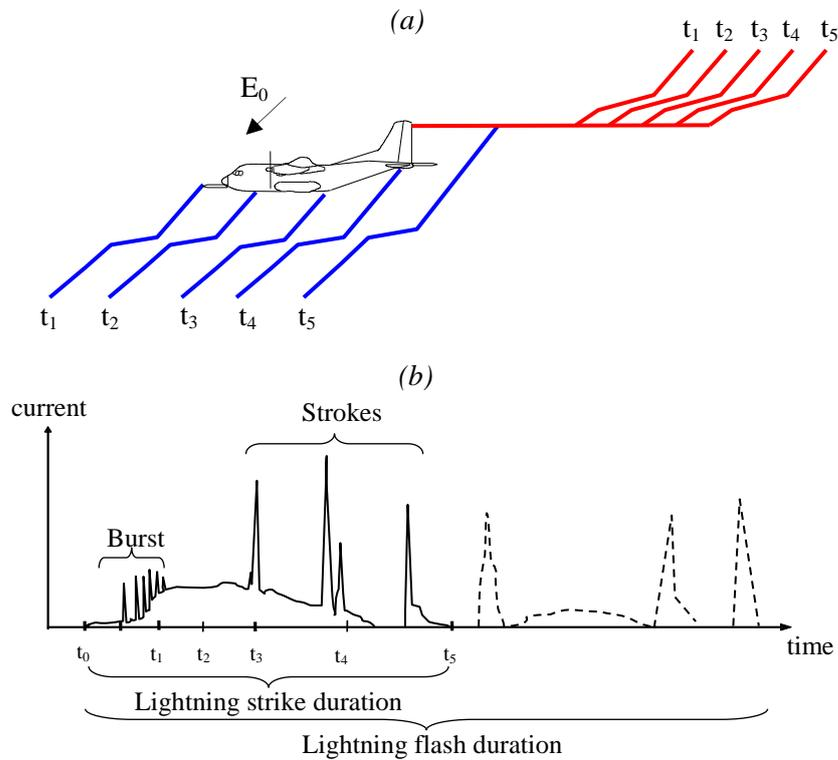
Figure I.7. Illustration of the swept stroke process. (a) The swept represented in the frame of reference of the aircraft for different times  $t_i$ . (Chemartin (2008)). (b) Typical current waveform obtained by in-flight measurements (Lalande et al. (1999)).
