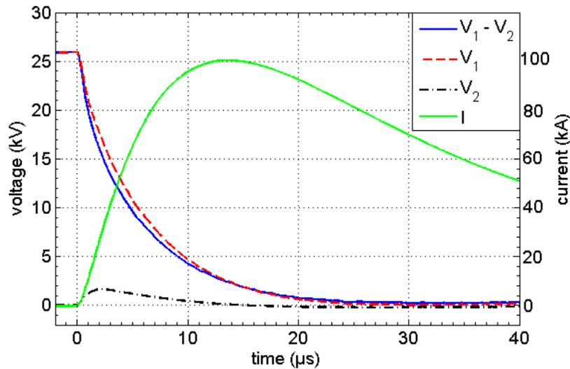
Figure IV.2. Example of voltage measurements by probes  $V_1$  and  $V_2$  and current measurements  $I$  by the probe A for the 100 kA peak.
