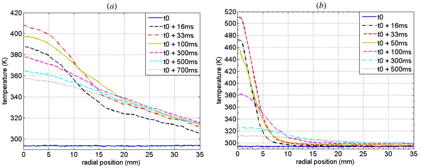
Figure VI.21. Radial profiles of temperature of aluminum panels with 1 mm thickness. (a) Unpainted panel. (b) 100 μm painted panel.
