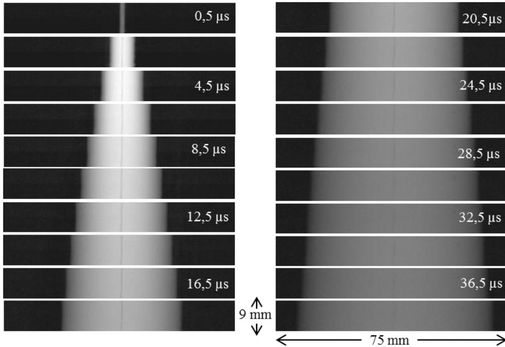
Figure III.5. Pictures of the column expansion during the first 38.5  $\mu$ s. Experimental parameters – current peak: 100 kA; resolution:  $256 \times 32$  pixels; scale: 0.29 mm/pixel; exposure time: 300 ns.
