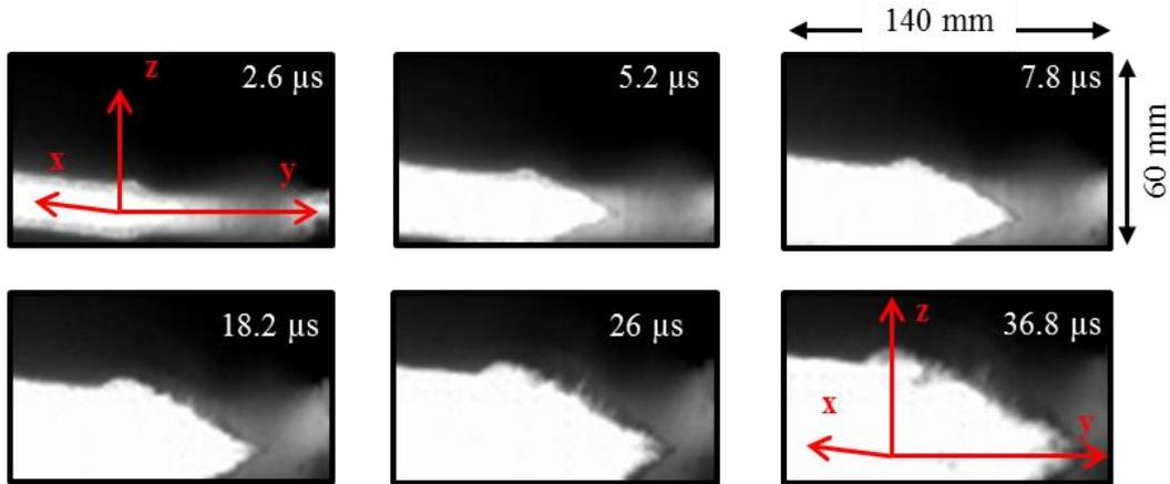
Figure VI.10. Pictures of the arc taken from an oblique angle to the material surface, to put in evidence the shape of the arc roots. The arc column axis oriented along the  $x$ -axis and the composite panel is in the plane  $yz$ , with the surface ply along the  $z$ -axis.
