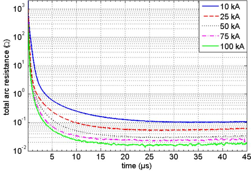
Figure IV.5. Evolution over time of the total arc resistance for all current levels.
