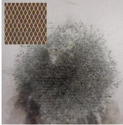
*Figure I.12. After test result for a carbon composite sample with copper mesh protection
