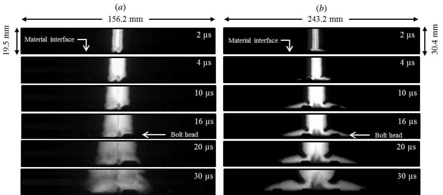
Figure VI.9. Pictures of the arc root evolution over time applied to a carbon fiber composite panel. (a) Camera axis perpendicular to the surface ply orientation (resolution:  $256 \times 32$  pixels; scale:  $0.61 \text{ mm/pixel}$ ; exposure time:  $0.3 \mu\text{s}$ ). (b) Camera axis parallel to the surface ply orientation (resolution:  $256 \times 32$  pixels; scale:  $0.95 \text{ mm/pixel}$ ; exposure time:  $0.3 \mu\text{s}$ ).
