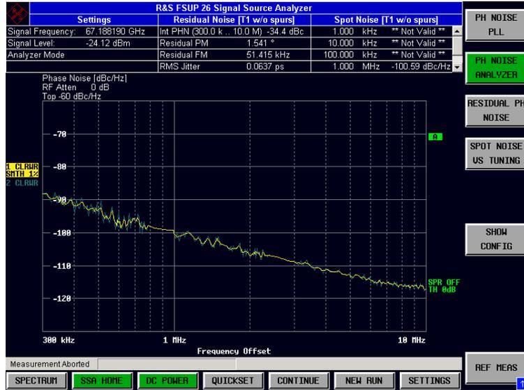
Figure 4.38: Measured Phase Noise at 1MHz of the 67GHz signal at the  $2 \times f_o$  port.
