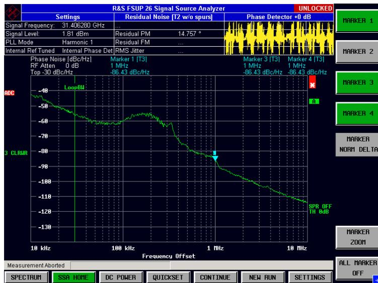
Figure 4.30: Measured Phase Noise at the  $f_o$ -port in the unlocked condition: "sub-harmonic VCO"–off.
