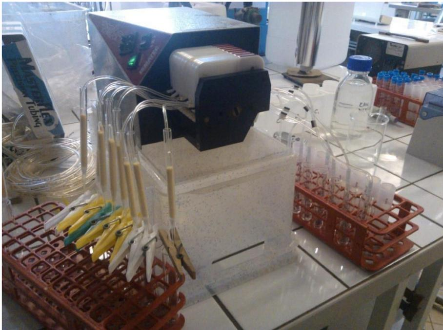
Figure 1: multi-pump de type ISMATEC - Ecoline VC-MS/CA.
