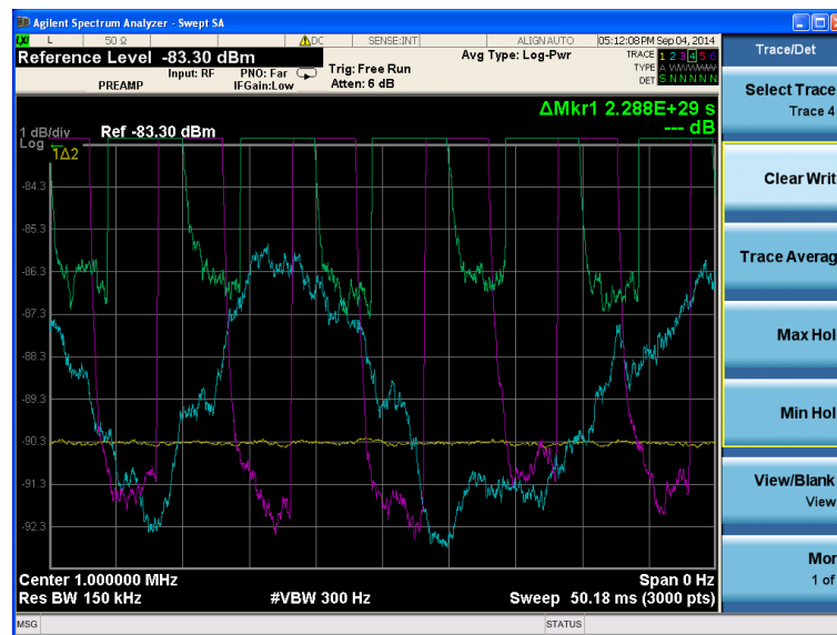
Figure 7.9: Locked squeezing and scan squeezing measured by a spectrum analyzer. The blue oscillation is the squeezing curve when scanning the homo phase. The pink curve is the vacuum squeezing when the deamplification and the amplitude quadrature are both locked with the shutter control. Similar for the green curve, when the amplification and the same homodyne quadrature phase are locked, we can see the locked anti-squeezing of the squeezed vacuum.
