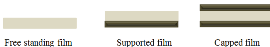
Figure 0-1. Three forms of polymer thin films: free standing, supported and capped films.
