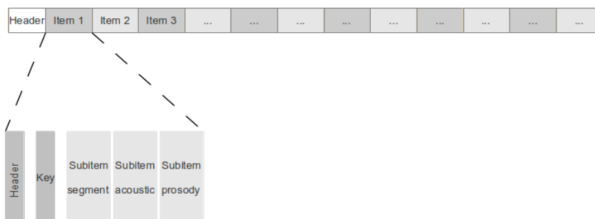
Figure 5.5: Structure of the TTS corpus. Each segment is prefixed by a header and a key and has a fixed size to make recovery and reading speed faster
