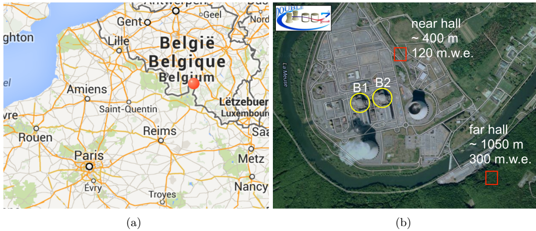
Figure 2.1: 2.1(a): The Chooz nuclear power plant is located in the French Ardennes region in the north of France, at the border with Belgium. 2.1(b): The two detector sites (red rectangles) are located at \sim 400 m and \sim 1050 m from the cores B1 and B2 (yellow circles).
