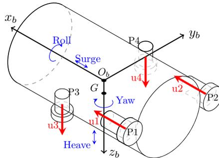
Figure 4.2: RSM fixed propulsive topology.
