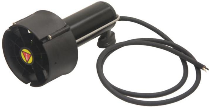
Figure 4.5: Seabotix BTD 150 thruster.
