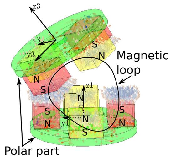
Figure 4.9: Magnetic coupling and forces (TE2M using Flux3D).
