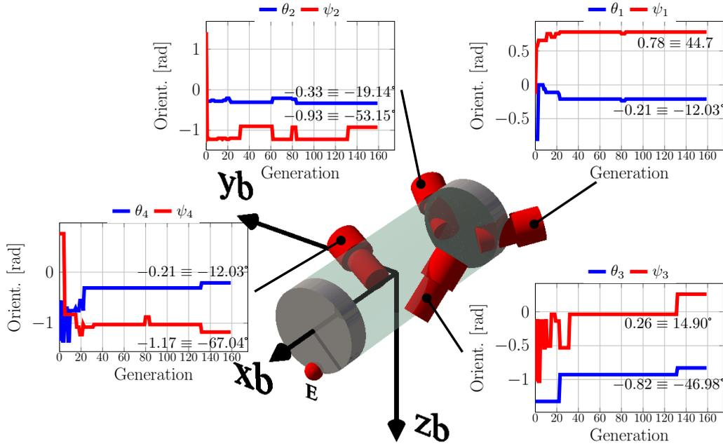
Figure 6.16: Orientation of thrusters on the RSM robot.
