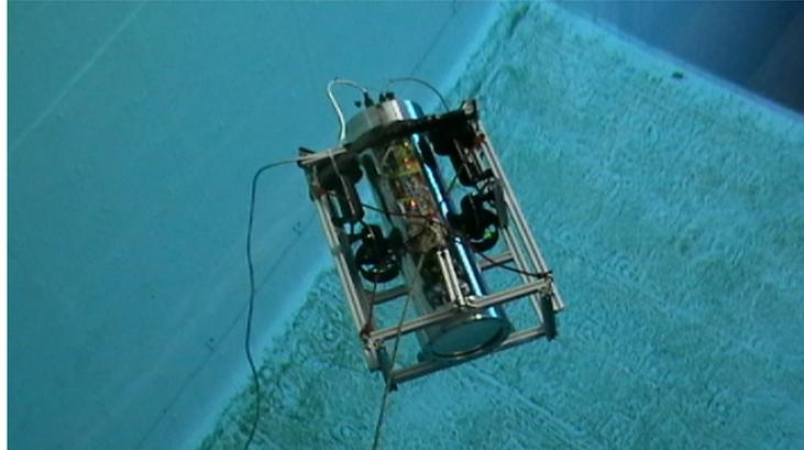
Figure 4.19: RSM robot tested in Ifremer bassin (sea water, 20 m).
