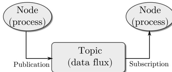
Figure 5.12: ROS minimal structure example.
