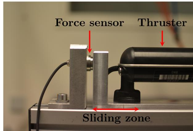
Figure 4.6: Force measuring test rig.
