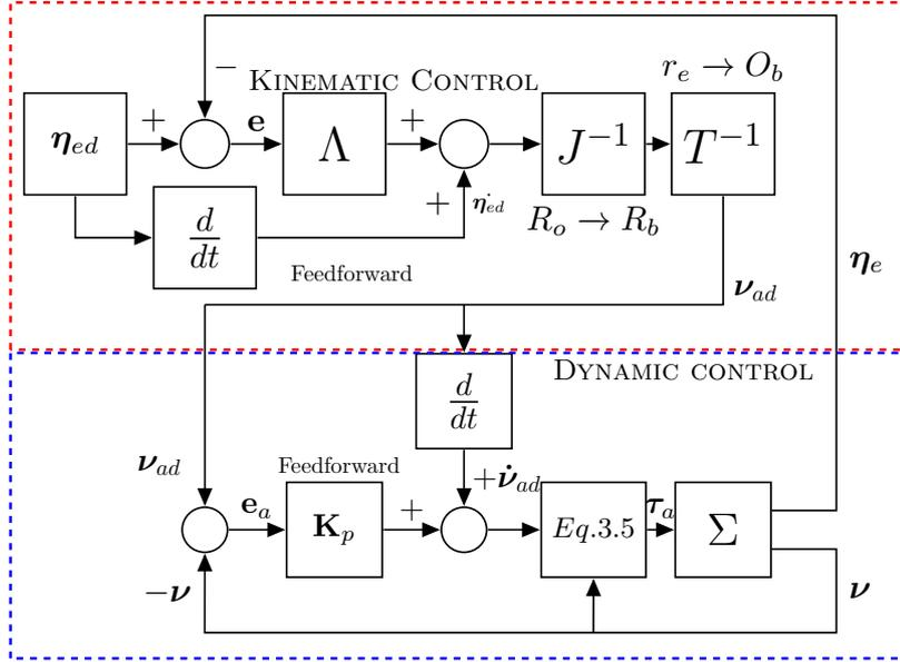
Figure 5.2: Computed torque control layers.
