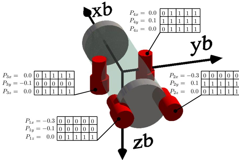
Figure 6.6: Thrusters position encoding (example of RSM robot).
