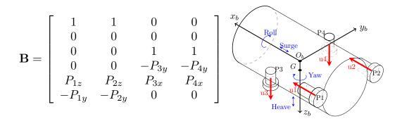
Figure 4.2: RSM fixed propulsive topology.
