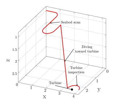
Figure 6.25: Trajectory for water turbine inspection.
