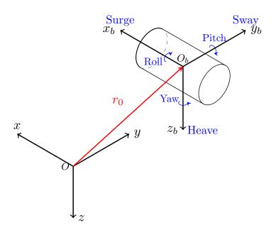
Figure 4.1: Earh-fixed and body-fixed frames.
