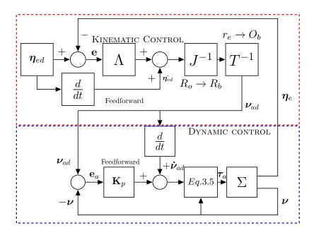
Figure 5.2: Computed torque control layers.
