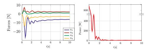
Figure 6.37: Forces and power consumption during the tomography task.
