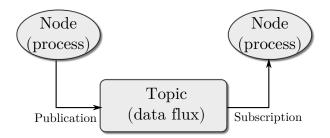
Figure 5.12: ROS minimal structure example.
