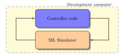
Figure 5.14: Software-in-the-loop schematic representation.
