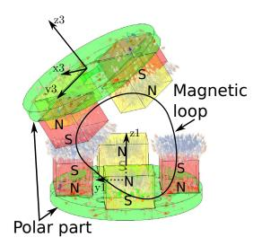
Figure 4.9: Magnetic coupling and forces (TE2M using Flux3D).
