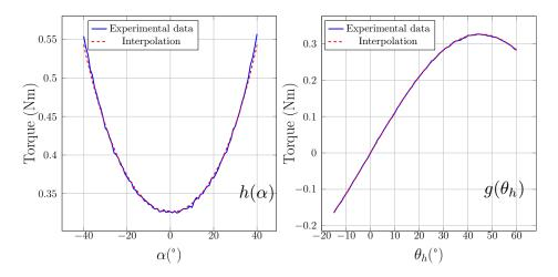
Figure 4.11: Interpolation curves for the magnetic coupling torque.
