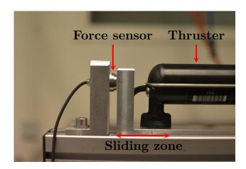
Figure 4.6: Force measuring test rig.
