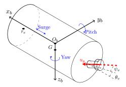
Figure 5.4: RSM robot with vectorial thruster.
