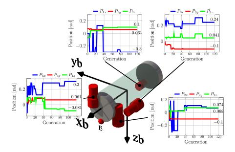
Figure 6.14: Position of thrusters on the robot.
