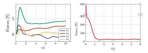
Figure 6.45: Forces and power consumption during diving phase (dyn. conf.).
