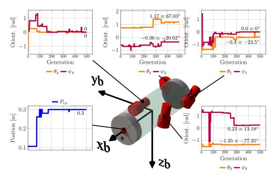
Figure 6.44: Final robot for diving phase (dynamic conf.).
