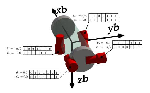
Figure 6.7: Thruster orientation encoding.
