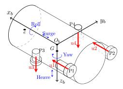
Figure 5.3: RSM robot with fixed propulsion topology.
