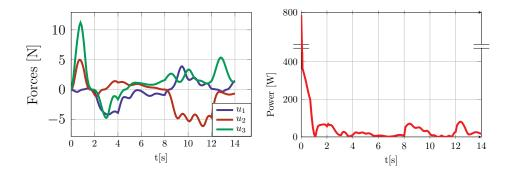
Figure 6.29: Forces and power consumption during the seabed scanning task.
