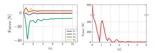
Figure 6.49: Forces and power consumption during tomography(dyn. conf.).
