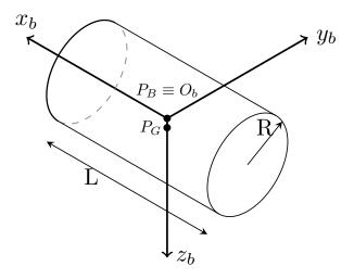
Figure 4.20: Simplified representation of the RSM AUV.
