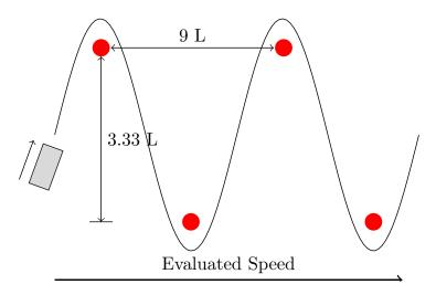
Figure 4.28: Slalom trajectory (horizontal or vertical).
