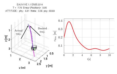
Figure 6.31: EAUVIVE simulation and kinematic error evolution for diving phase.
