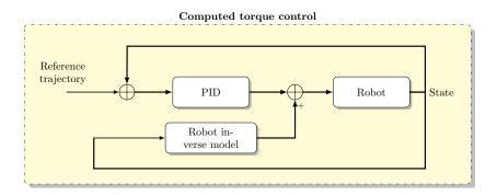
Figure 5.1: Computed torque control method principle.
