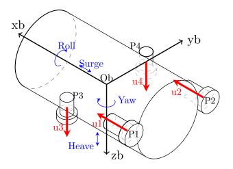
Figure 4.21: RSM fixed propeller architecture.
