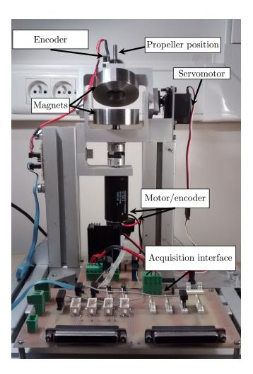
Figure 4.14: Flat RMCT prototype.
