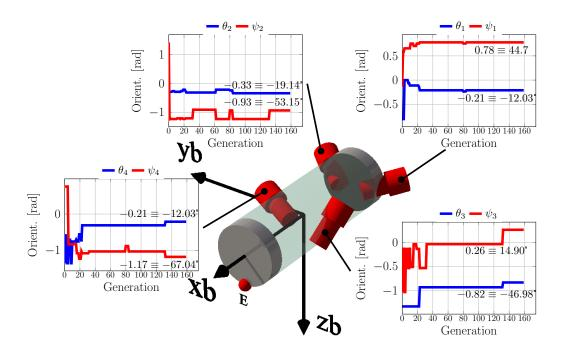
Figure 6.16: Orientation of thrusters on the RSM robot.
