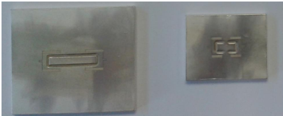
Figure 21: Picture of a compact resonator (32mmx27mm) and the previous design (22x16.8mm)
