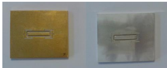
Figure 16: Copper and silver plated resonators
