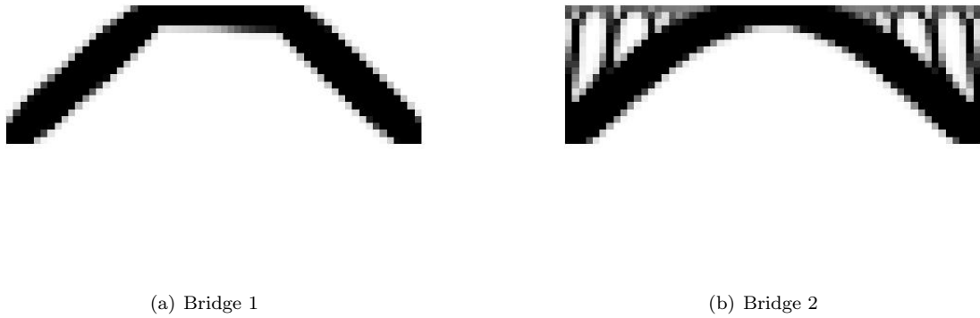
Figure 2: Results with the SIMP method, for two bridges. The structure is embedded on the left and right bottom side. A force is applied on the upper side, on a the whole side for 2(b) and on just a part 2(a).
