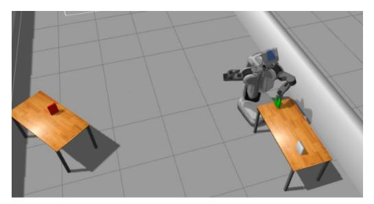
Figure 5.6: PR2 robot executing a plan in the Gazebo similator, with two of the three tables being visible.
