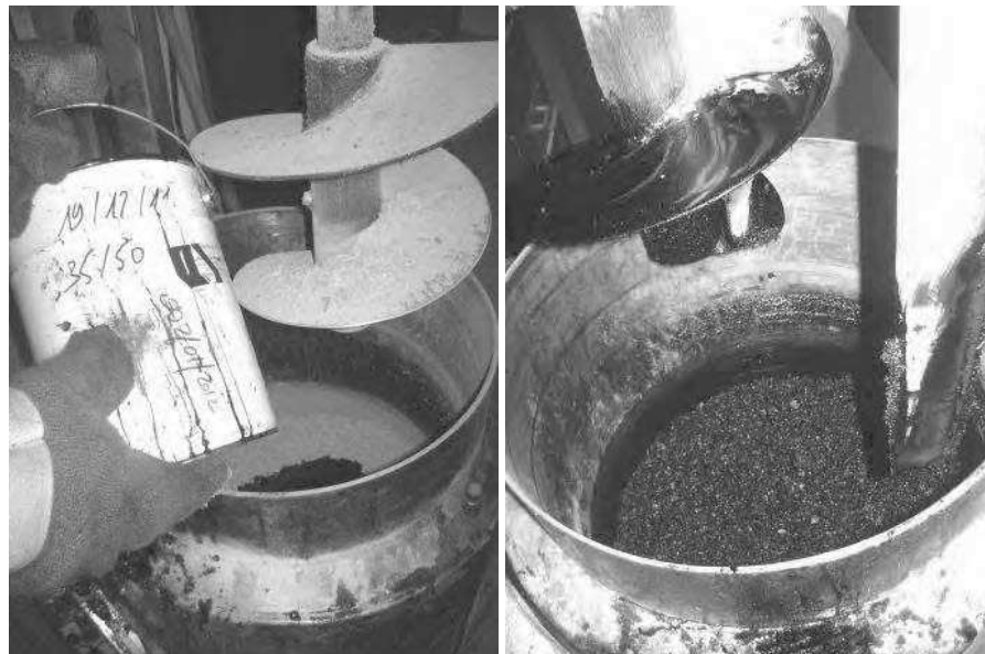
Figure 3-3 Addition of bitumen (at 160°C) to aggregates in mixer (left) and asphalt after mixing (right)
