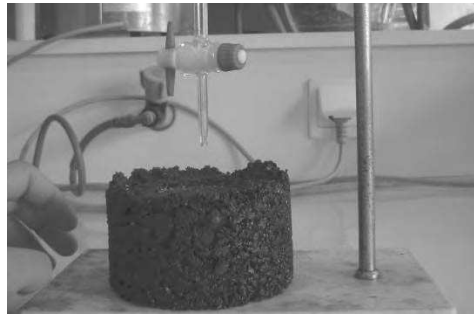
Figure 3-13 Application of ARA in the center of the sample
