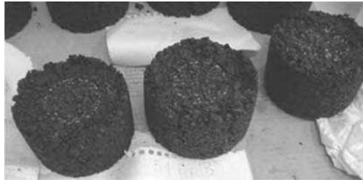
Figure 3-15 Asphalt samples after CBR loading
