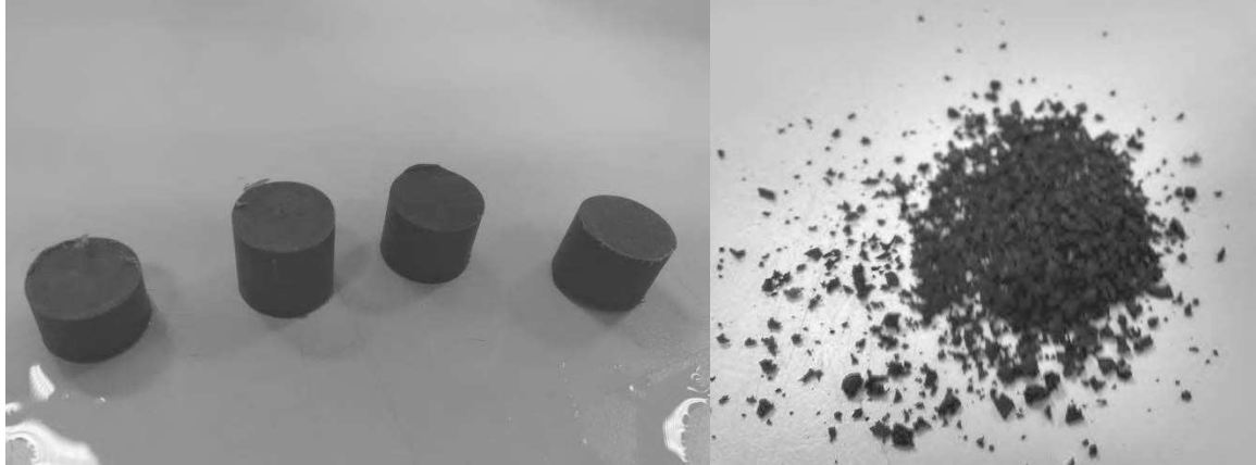
Figure 3-24 PVC and crumb rubber samples for testing BR degradation of construction materials
