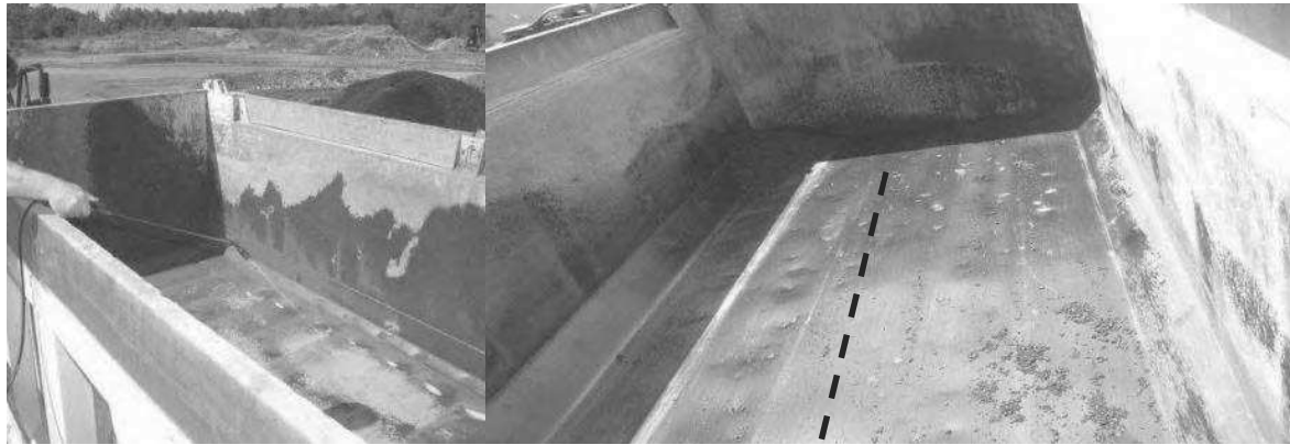
Figure 2-16 Application of ARA on truck bed (left); part of field Trial showing effectiveness of two ARAs (right) ("SITTM Asphalt Release Agent Field Trial," 2010)
