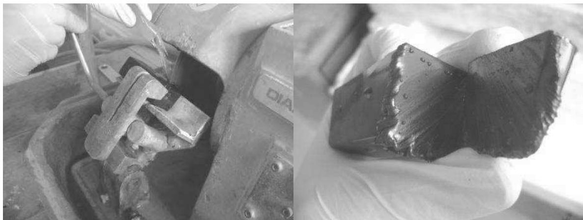
Figure 4-3 Bitumen sample for SEM being cut with a diamond saw
