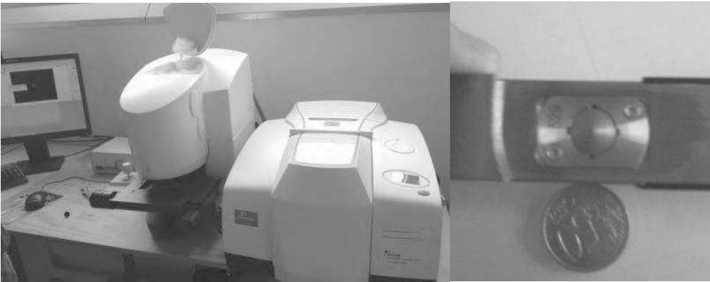
Figure 4-23 PerkinElmer Spotlight 400 coupled with a PerkinElmer Frontier Imager (left) and ZnSe ATR crystal (right)
