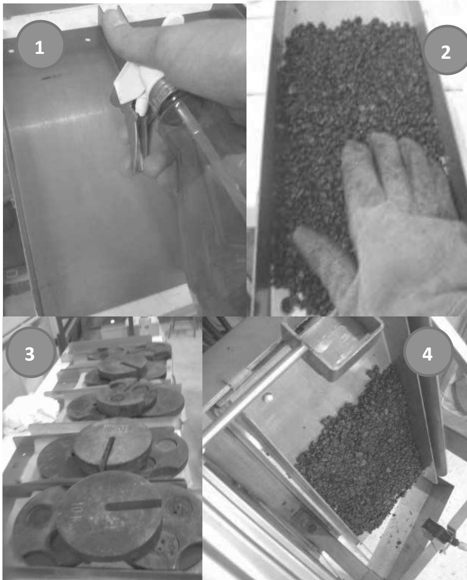
Figure 3-8 Asphalt Slide Test: 1) applying ARA, 2) asphalt spread on the plate, 3) load of 2.5kPa distributed on top of the asphalt and 4) the inclination of the plate on ARA-PEA at 45°
