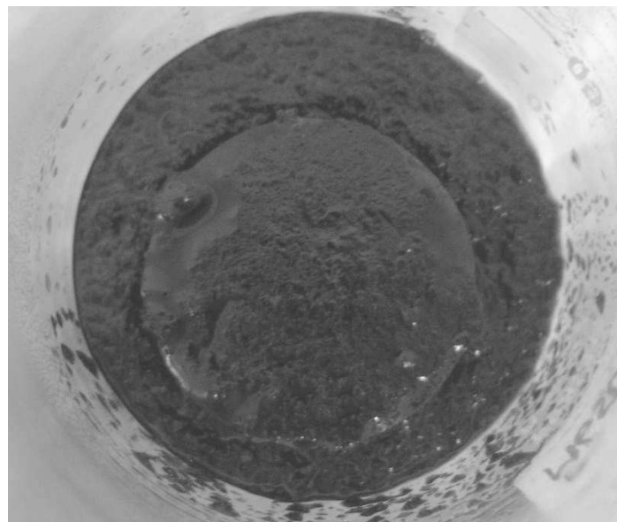
Figure 3-38 BDT sample showing bitumen after 1d exposure to MUG 50 ARA2 50; the bitumen has been degraded by the solution and the solution has coagulated
