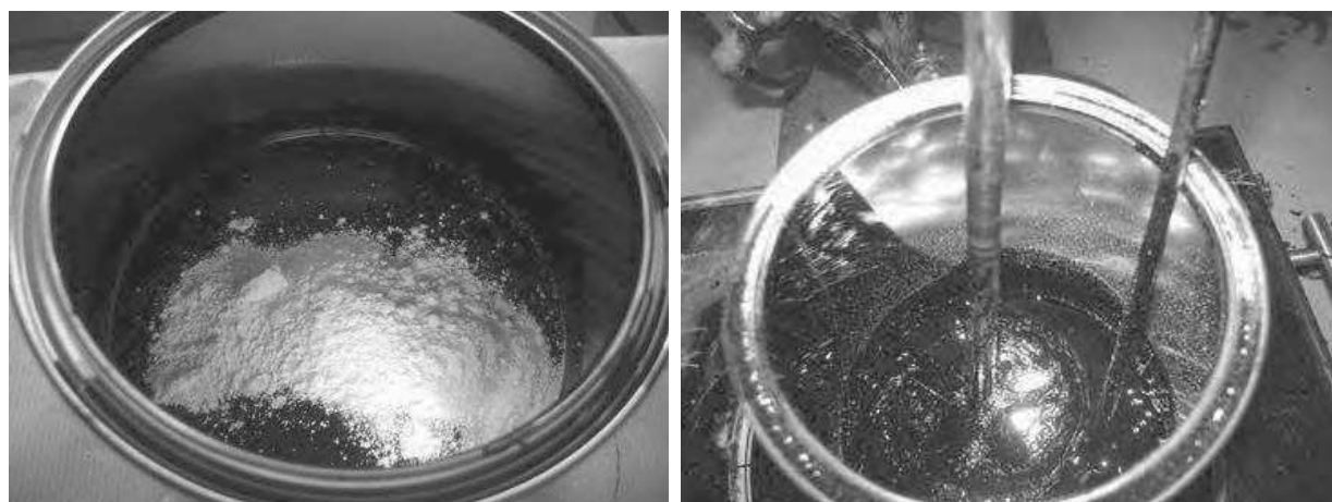
Figure 4-1 : Préparation the samples for SEM analysis including the addition of TiO 2 tracer (left) and the mixing with a Heidoph RZR mixer (right)
