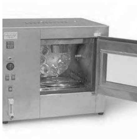
Figure 2-21 Rolling Thin Film Oven Test (Jet Materials)
