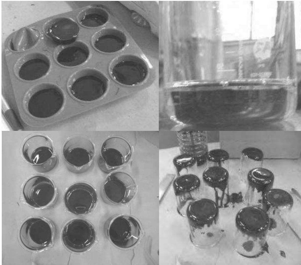
Figure 3-22 BDT silicon sample moulds (top left), sample submerged in ARA product (top right and bottom left) and beakers after test (bottom right)
