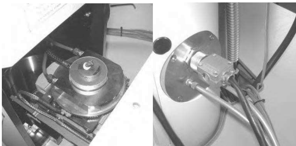
Figure 4-5 Peltier effect device with mastic sample inside the chamber and on the device (left) and the device coming out of the SEM chamber to the water source cooling the device (right)
