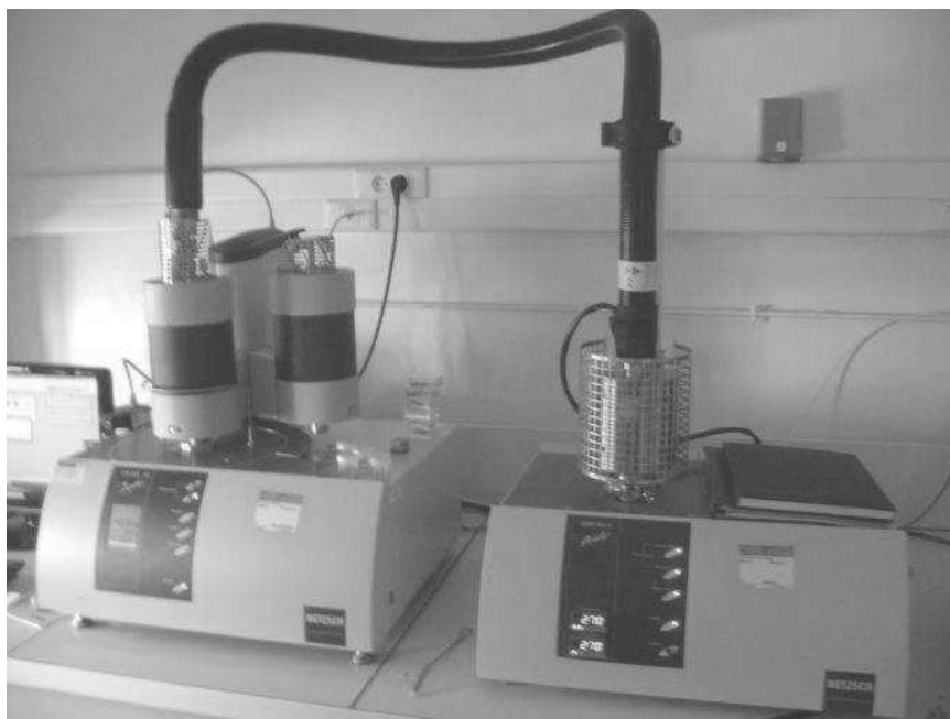
Figure 4-25 Netzsch thermogravimetric analyzer coupled with a mass spectrometry attachment (right, not used)
