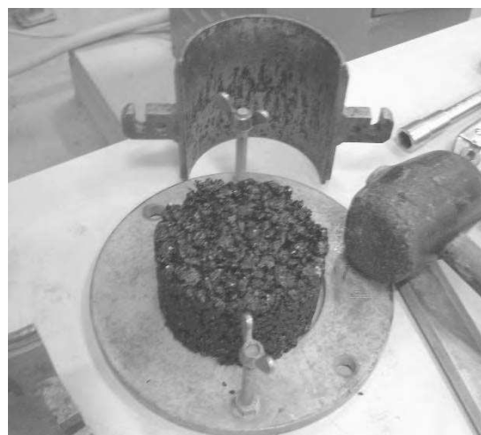
Figure 3-10 Demolding asphalt sample
