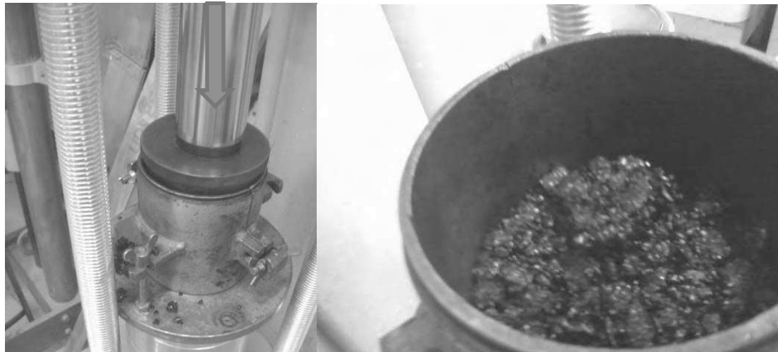
Figure 3-11 Compaction of asphalt sample by hydraulic compressor (left) and damaged surface of sample from the use of a cold piston (right)
