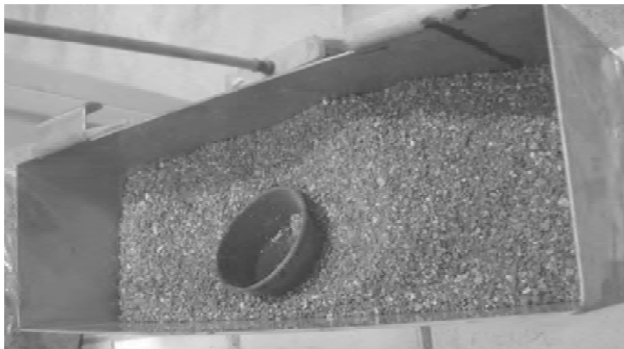
Figure 4-17 Larronde – Ainhoa limestone sand graded to 0.315/1 mm
