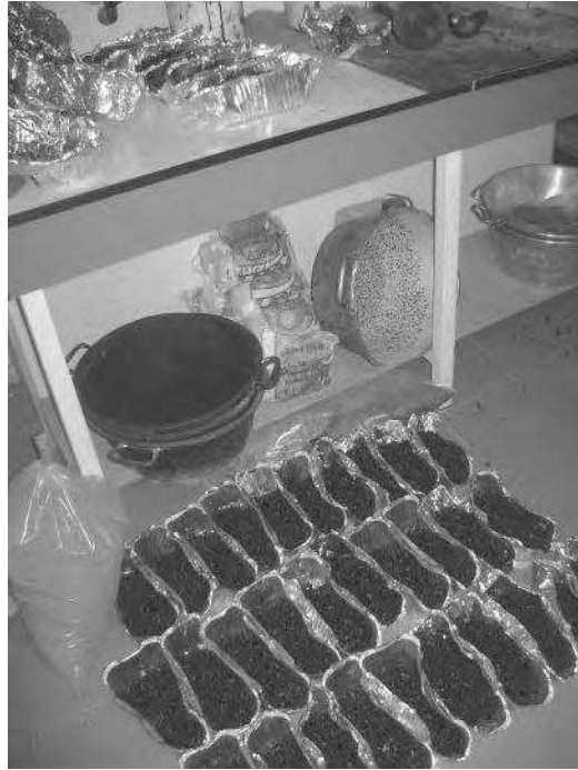
Figure 3-4 Asphalt after being placed into aluminum containers for storage
