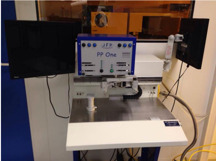
Figure 3.8: Photography of “pick and place” machine
