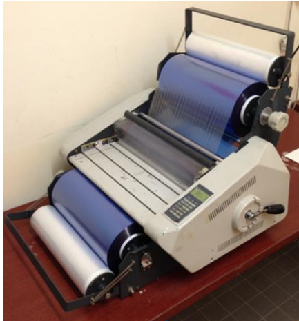
Figure 3.15: Photography of a film laminator and its principle function [96]
