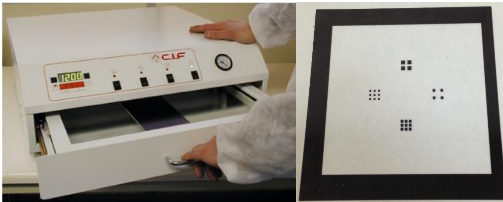
Figure 3.16: Photography of exposure machine [21] and a mask example
