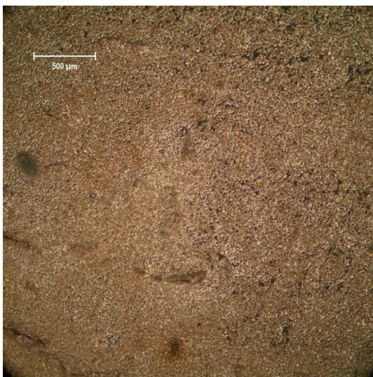
20 min copper plating on aluminum
