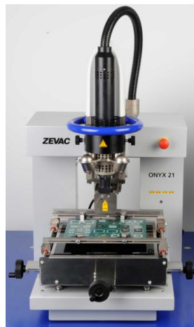
Figure 2.12: ZEVAC ONYX 21 Flip-chip bonder [102]
