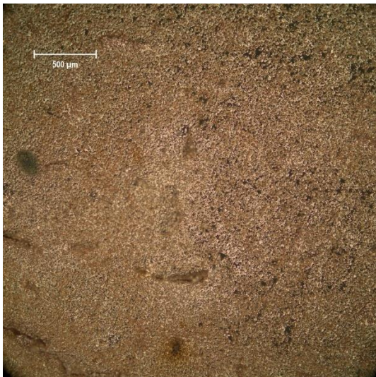
20 min copper plating on aluminum
