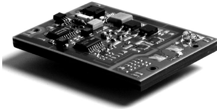
Figure 1.32: Thin 60-W offline converter with PCB integrated transformer and capacitors [76]
