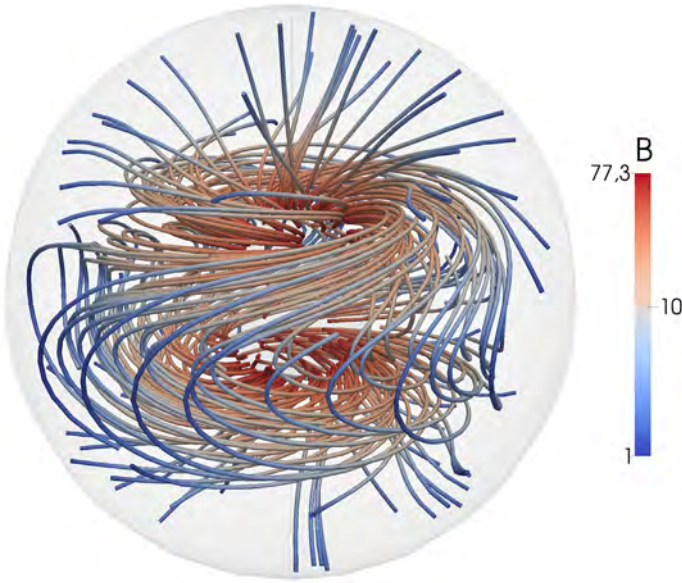
Fig. 9. 3D view of the magnetic configuration obtained with our 2D simulations at t_{\max} . It is computed for L_u = 10^2 , a density contrast \rho_c/\rho_0 = 7 \times 10^3 , the radial differential rotation profile defined by Eq. (12) and \Omega fixed at the inner radius.
