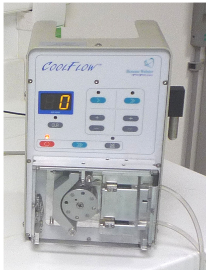
Fig. 3.17 – Pompe d'irrigation Coolflow (Biosense Webster) [179].
