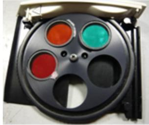
Figure 5.3: Customized filter wheel ensuring no light leakage around the filters.
